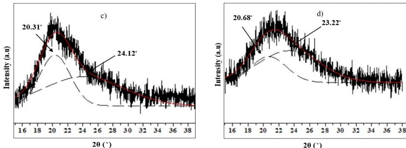
**Figure 9.** Deconvolution for several weight percent of CaSCN–agarose within range  $13^\circ$  and  $37^\circ$  at room temperature. (a) 0 wt.%, (b) 10 wt.%, (c) 25 wt.%, and (d) 40 wt.
