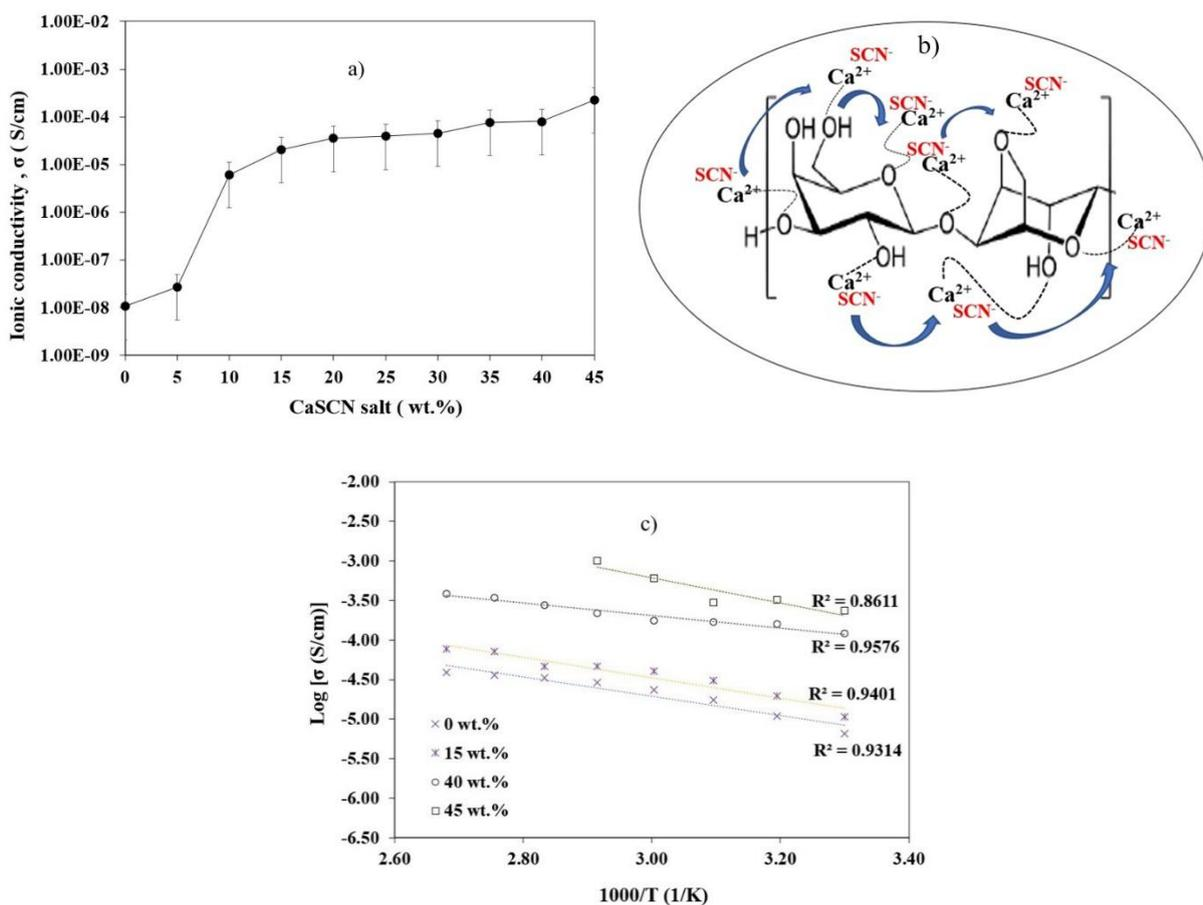
**Figure 3.** (a) Ionic conductivity of different amounts of CaSCN salt at room temperature, (b) Hopping mechanism of  $\text{Ca}^{2+}$  in CaSCN–agarose biopolymer electrolytes, (c) Temperature dependence plots of different concentration of CaSCN–agarose biopolymer electrolytes.
