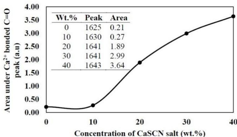
**Figure 7.** The area under peak  $\text{Ca}^{2+}$  bonded  $\text{C}=\text{O}$  as a function of  $\text{CaSCN}$  concentration in selected  $\text{CaSCN}$ –agarose biopolymer electrolytes.
