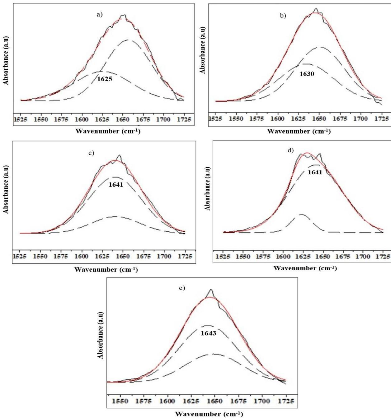
**Figure 6.** Deconvolution at C=O region within range 1525 cm<sup>-1</sup> to 1725 cm<sup>-1</sup> for several weight percent of CaSCN—agarose biopolymer electrolytes. (a) 0 wt.%, (b) 10 wt.%, (c) 20 wt.%, (d) 30 wt.%, e) 40 wt.%
