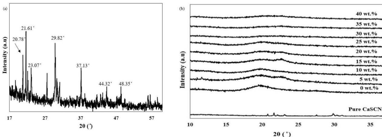
**Figure 8.** (a) Diffractogram of pure  $\text{CaSCN}$ , (b) XRD spectrum of  $\text{CaSCN}$ –Agarose biopolymer electrolytes system.
