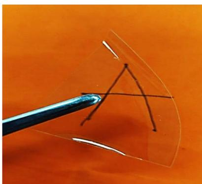
**Figure 1.** A clear thin film of CaSCN–agarose biopolymer electrolyte.
