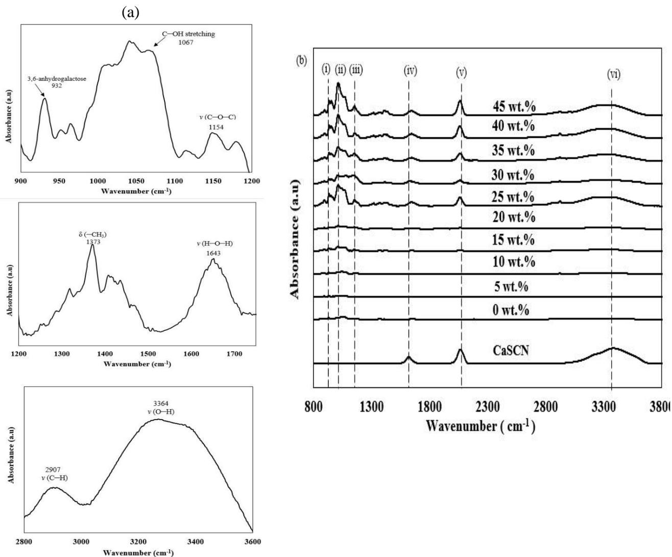
**Figure 5.** (a) Significant peaks for pure agarose (b) FTIR spectrum for pure CaSCN salt and CaSCN–agarose biopolymer electrolytes’ system.
