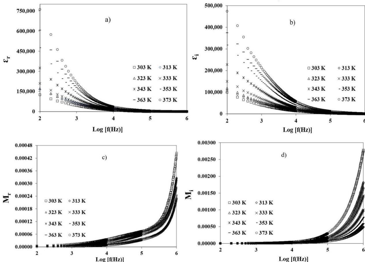
**Figure 4.** Electrical properties of CaSCN–agarose biopolymer electrolytes (a) Dielectric storage, (b) Dielectric loss, (c) Real modulus, (d) Imaginary Modulus.
