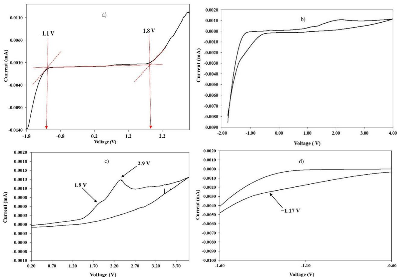
**Figure 10.** Electrochemical studies of the highest conducting film (a) Linear sweep voltammetry and (b) Cyclic voltammetry (scan rates  $5 \text{ mV}\cdot\text{s}^{-1}$ ), (c) Anodic peak, (d) Cathodic shoulder peak.
