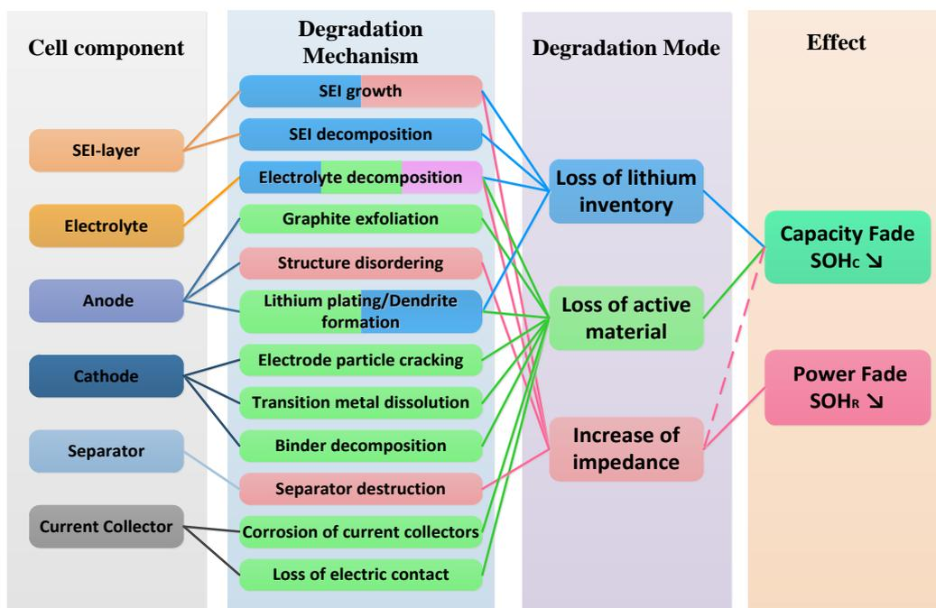
**Figure 5.** The causal relationship of the influence of different parts of the aging mechanism of lithium batteries on the SOH.
