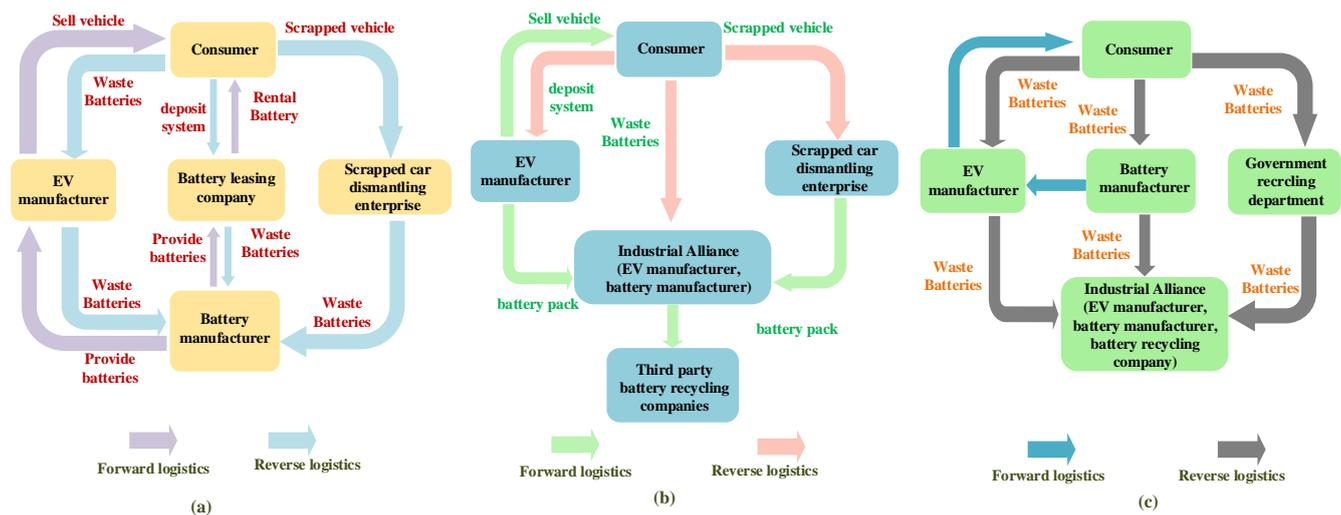
**Figure 2.** Recycle modes of waste batteries in different regions: (a) Japan, (b) USA/EU, and (c) China.
