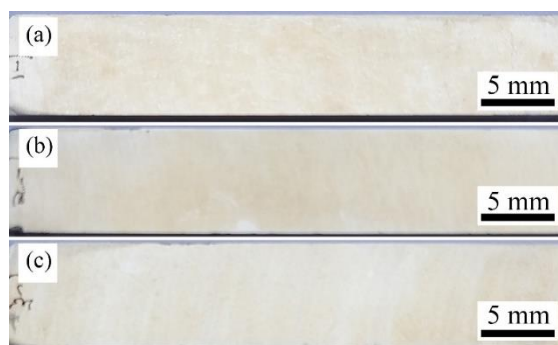
Figure 2. Macroscopic corrosion morphology of the steels after immersion and removing corrosion products: (a) 0.63N; (b) 0.79N; (c) 0.86N.
