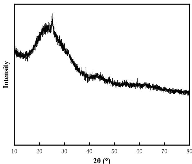
**Figure 2.** XRD pattern of the porous carbon-based anode material
