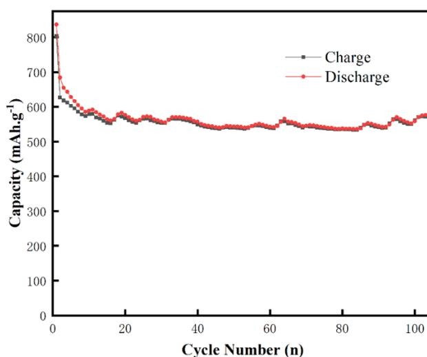
**Figure 6.** Cycling performance of the porous carbon-based anode material at a current density of 100 mA/g
