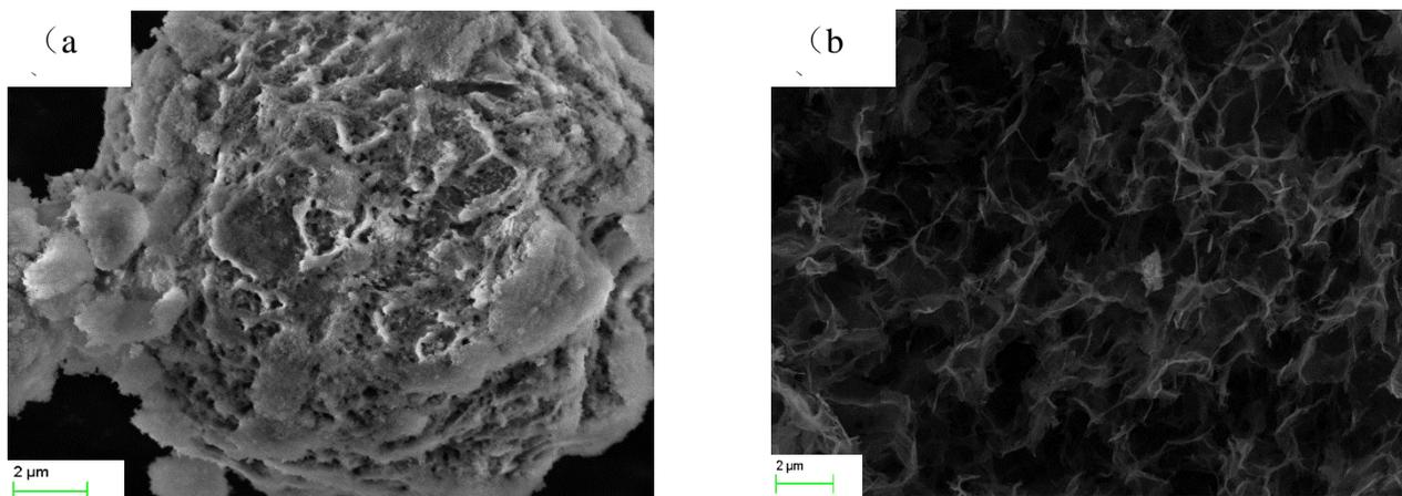
**Figure 1.** SEM micrographs of the precursor cellulose aerogel (a) and porous carbon-based anode material (b)
