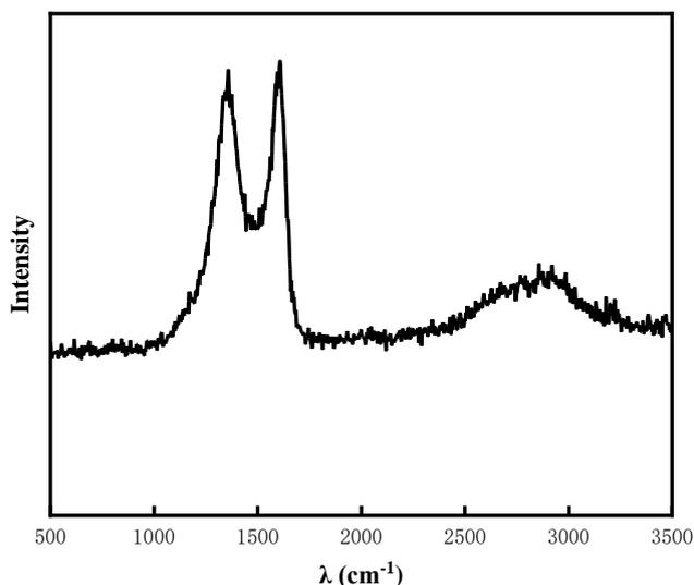
**Figure 3.** the Raman spectrum of the porous carbon-based anode materials
