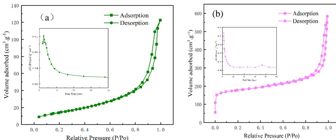
**Figure 4.** N<sub>2</sub> adsorption/desorption isotherms of the precursor cellulose aerogel (a) and porous carbon-based anode material (b)
