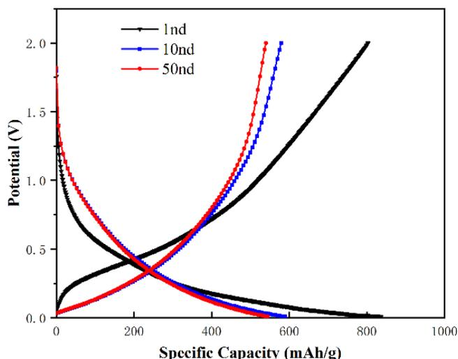
**Figure 5.** Charge–discharge curves of the porous carbon-based anode material obtained at a current density of 100 mA/g
