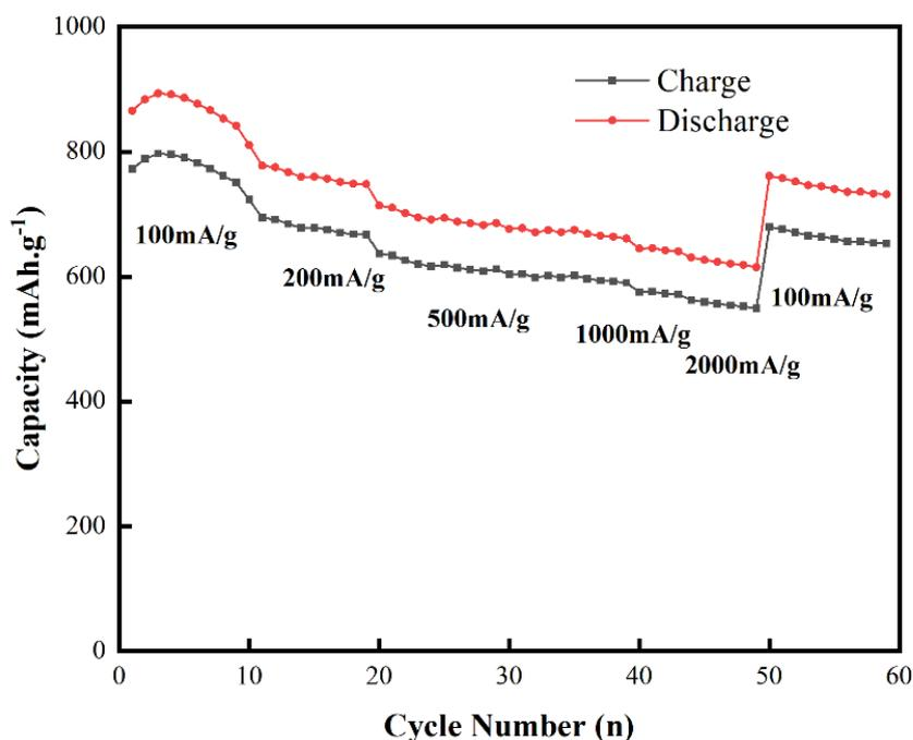
**Figure 7.** Rate capability at different current densities of the porous carbon-based anode material
