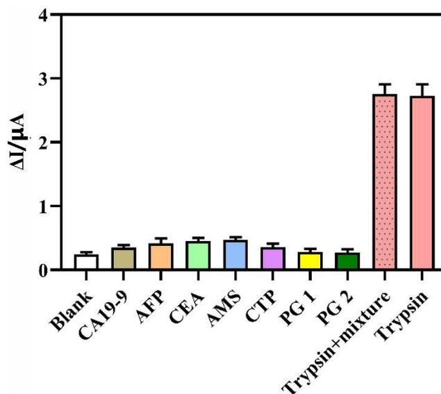
**Figure 7.** Histogram of detecting result of six clinical common typical serum markers (including CA19-9, AFP, CEA, AMS, CTP, PG 1 and PG 2), trypsin+mixture and trypsin; Concentrations were all 1 ng/mL. The error bars were relative standard deviation of six parallel experiments.
