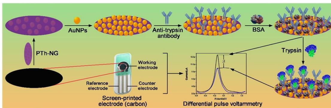
**Figure 1.** Schematic diagram of preparing label-free electrochemical immunosensor based on polythionine-nanogold nanocomposite for detection of trypsin on screen-printed electrode
