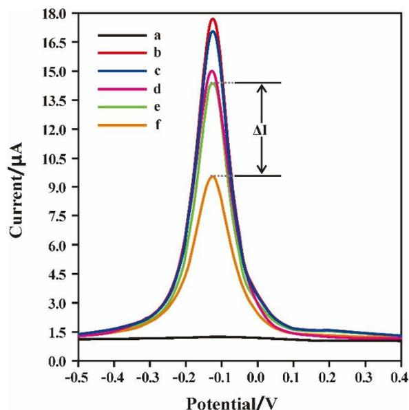
**Figure 6.** DPV curves of bare SPE (a), PTh-NG/SPE (b), Au/PTh-NG/SPE (c), Antibody/Au/PTh-NG/SPE (d), BSA/Antibody/Au/PTh-NG/SPE (e) and Trypsin/BSA/Antibody/Au/PTh-NG/SPE (f) were measured in PBS with pH of 5.5.
