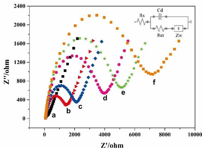
**Figure 5.** EIS of bare SPE (a), PTh-NG/SPE (b), Au/PTh-NG/SPE (c), Antibody/Au/PTh-NG/SPE (d), BSA/Antibody/Au/PTh-NG/SPE (e) and Trypsin/BSA/Antibody/Au/PTh-NG/SPE (f) were detected in 10 mmol/L  $[\text{Fe}(\text{CN})_6]^{3-/4-}$  solution containing 0.1 mol/L KCl; the inset was the equivalent circuit diagram.
