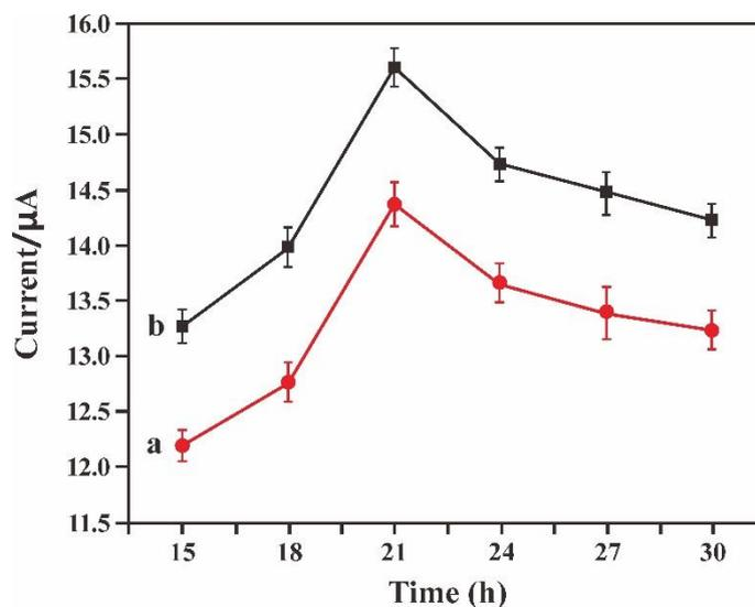
**Figure 4.** Broken line graph of DPV peak current of PTh (a) and PTh-NG (b) with different drying time on SPE surface; the error bars were relative standard deviation of three parallel experiments.
