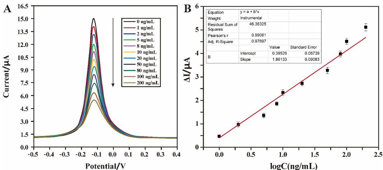
**Figure 8.** (A) DPV curves of different concentrations of trypsin; the concentrations of trypsin were successively 0, 1, 2, 5, 8, 10, 20, 50, 80, 100 and 200 ng/mL from top to bottom. (B) Calibration curve between logarithms of trypsin concentrations and variation of DPV peak current; the error bars were relative standard deviation of three parallel experiments.
