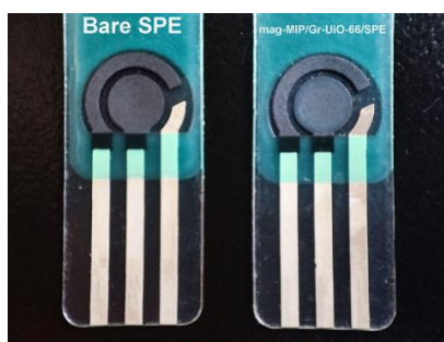
Figure 6. The images of mag-MIP/Gr-UiO-66/SPE (right) and bare SPE (left).
