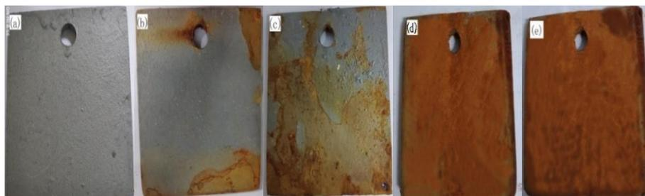
**Figure 2.** Macroscopic morphology of the sample after corrosion in different corrosive media (a. non-corroded sample, b. DO concentration=0.5 mg/L; c. DO concentration=0.5 mg/L & pH=6 d. simulated seawater, e. pH=6)
