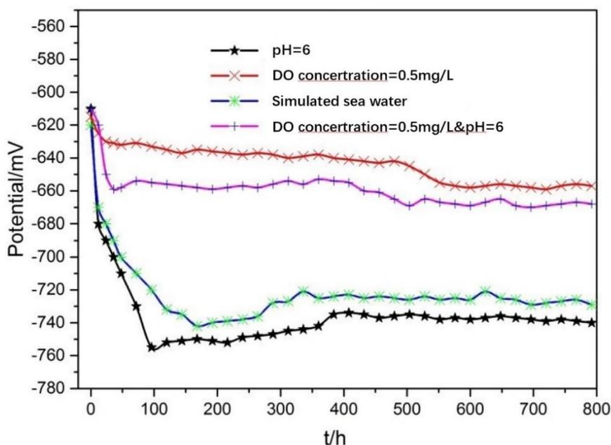
**Figure 4.** Open circuit potential-time curve of samples in different corrosive media
