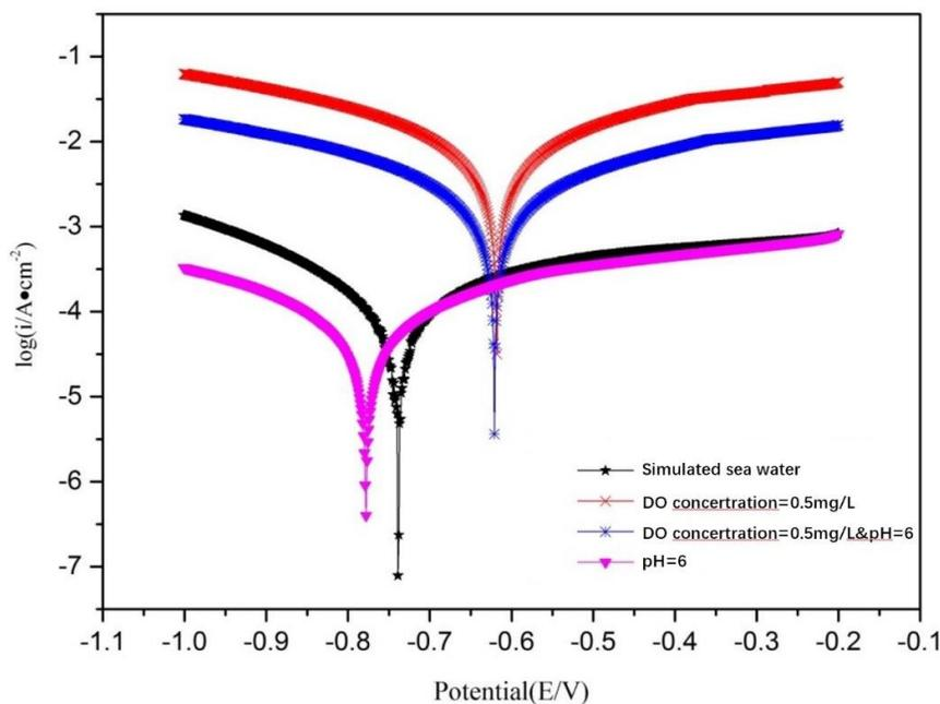
**Figure 5.** Polarization curve of the sample in different corrosive media
