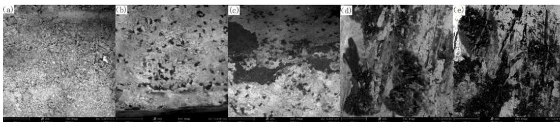
**Figure 3.** Macroscopic morphology of the sample after corrosion in different corrosive media (a. non-corroded sample; b. DO concentration=0.5 mg/L; c. DO concentration=0.5 mg/L & pH=6 d. simulated seawater; e. pH=6)
