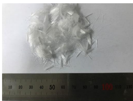
Figure 3. PVA fiber with a length of 8 mm and diameter of 40 μm.
