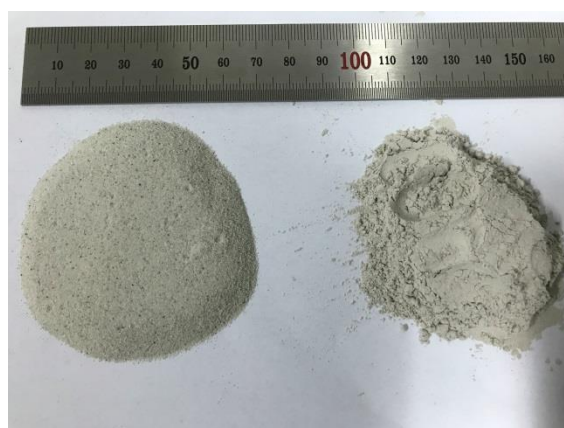
Figure 1. Crushed ceramic sand(left) and ground ceramic powder(right) made from demolished floor tiles (Sand particle size: 0.075-0.15 mm; ground ceramic powder particle size: less than 60 \mu\text{m} ).
