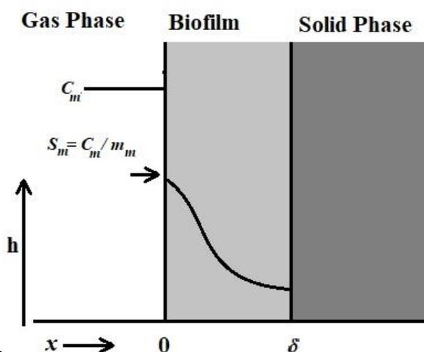
**Figure 1.** Biophysical model for the biofilm structure based on biofilter packing materials and concentration profiles across the biofilm [15-17].
