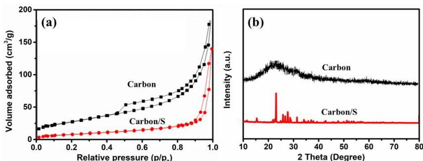
**Figure 1.** (a) N<sub>2</sub> adsorption and desorption profiles of the carbon and carbon/S composites. (b) XRD patterns of the carbon and carbon/S composites at 2θ range of 10°-80°.
