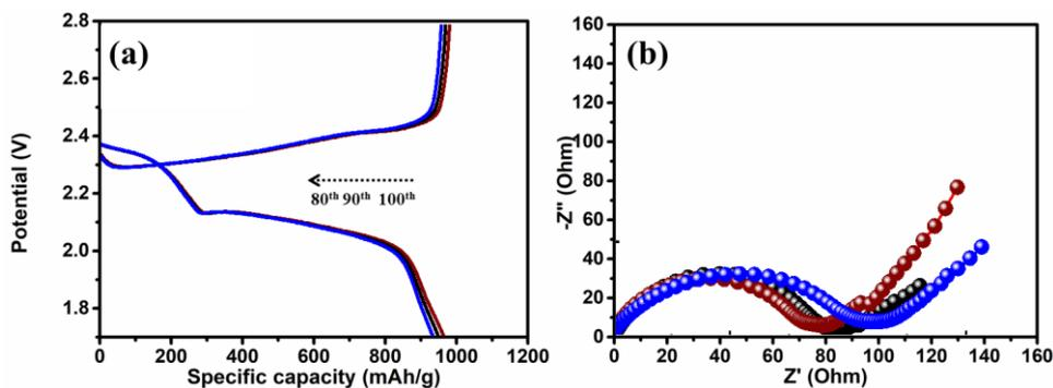
**Figure 4.** (a) The constant discharge and charge profiles of the carbon/S composites at the current density of 0.2 C. (b) Electrochemical impedance spectrum of the carbon/S composite at different cycles.
