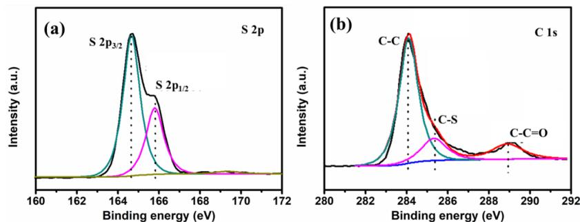
**Figure 3.** XPS spectrum for the carbon/S composite (a) S 2p and (b) C 1s.
