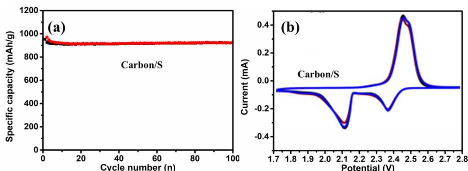
**Figure 5.** (a) Cycle performance of the carbon/S composite at the current density of 1 C. (b) CV curve of the carbon/S composites with scanning rate of  $0.1 \text{ mV s}^{-1}$ .
