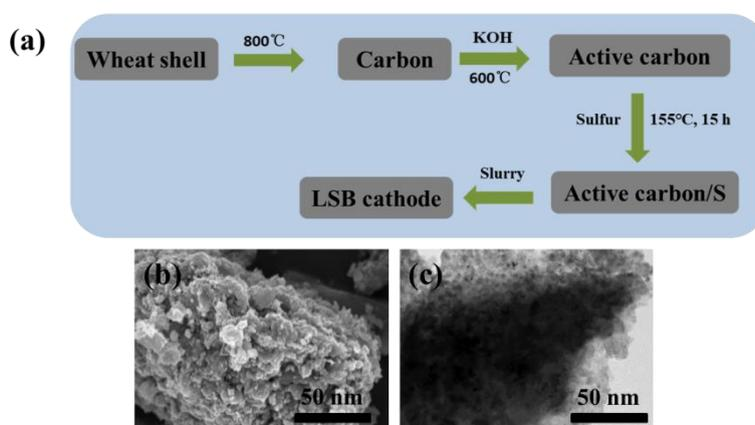
**Figure 2.** (a) Preparing process of the carbon/S composites. (b) and (c) SEM and TEM image of the carbon/S composites.
