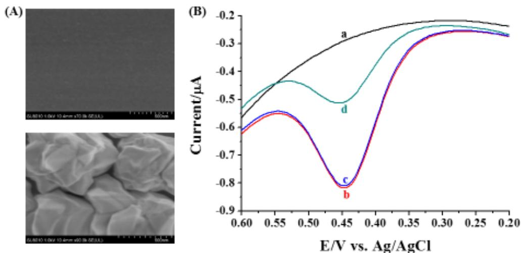
**Figure 1.** (A) SEM images of GCE before (top) and after (bottom) electrodeposition of AuNPs. (B) DPV responses of the SAMs-covered AuNPs/GCE (curve a) and the Fc-AuNPs/GCE before (curve b) and after incubation with buffer blank (curve c) or 20 pM Mpro (curve d).
