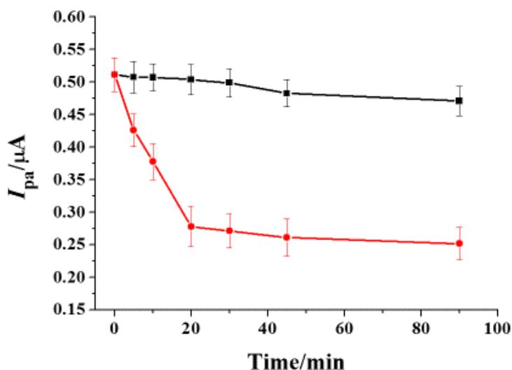
**Figure 2.** Effect of incubation time on the  $I_{pa}$  acquired at the Fc-AuNPs/GCE after incubation with buffer blank (black dotted curve) and Mpro (red dotted curve).
