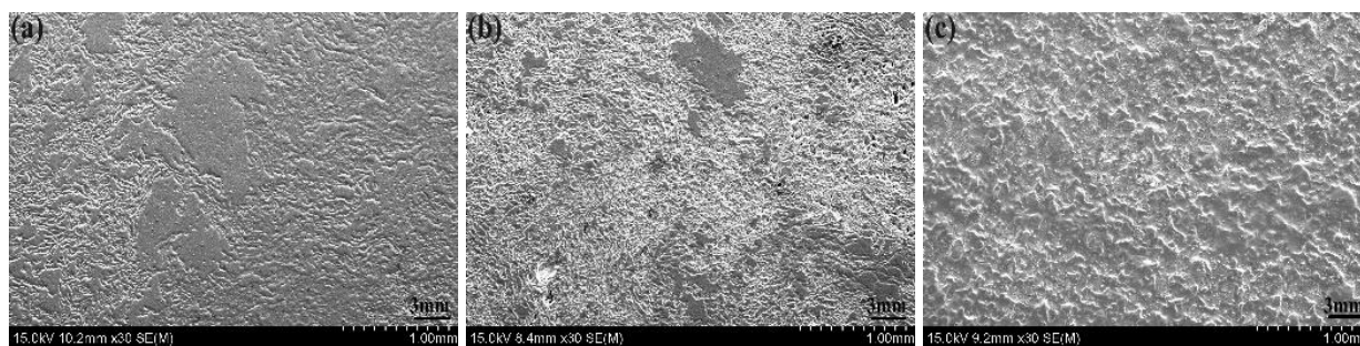
Figure 2. Morphology of Mg-1.5Mn-2.0Y alloy after being corroded for seven days in three solutions (a) 0.9wt.% NaCl, (b) 3.5wt.% NaCl, (c) SBF
