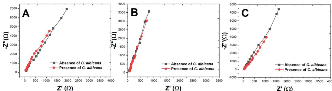
**Figure 6.** Nyquist plots of titanium-nickel in artificial saliva with and without *Candida albicans* at (A) 24 h, (B) 120 h and (C) 240 h.
