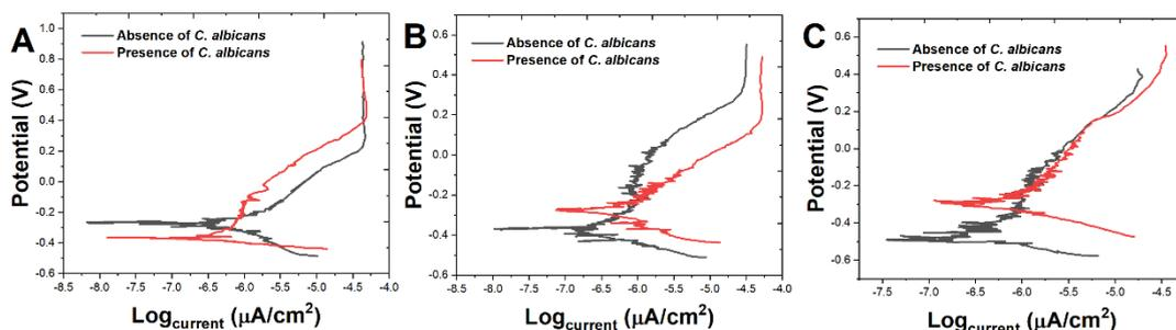
**Figure 5.** Potentiodynamic polarization curves of titanium-nickel alloy in artificial saliva with and without *Candida albicans* at (A) 24 h, (B) 120 h and (C) 240 h.
