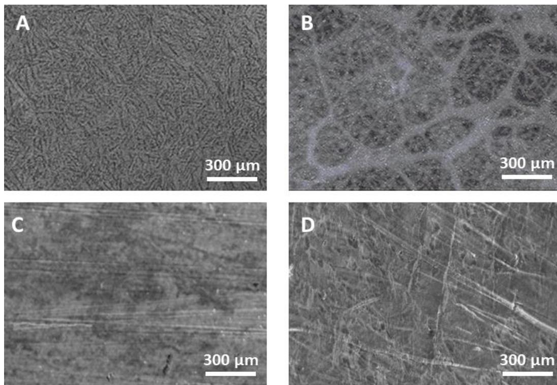
**Figure 7.** SEM images of titanium-nickel alloy surface in the (A) absence and (B) presence of *Candida albicans*. SEM image of titanium-nickel alloy surface (C) without *Candida albicans* and (D) removal of biofilm.
