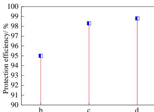
**Figure 5.** Protection efficiency of different anodic oxide films for aluminum alloy, b-anodic oxide film, c-anodic oxide film after sealing, d-anodic oxide film after sealing and surface modification
