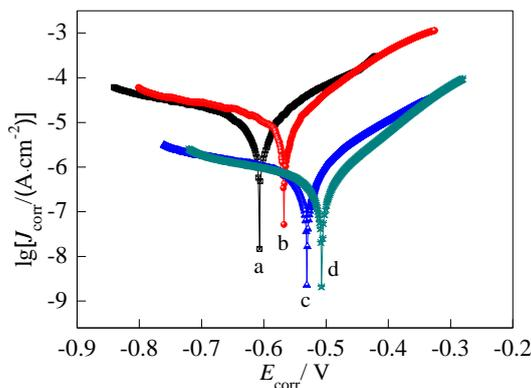
**Figure 4.** Polarization curves of aluminum alloy and different anodic oxide films, a-aluminum alloy, b-anodic oxide film, c-anodic oxide film after sealing, d-anodic oxide film after sealing and surface modification (scanning potential ranges from -250 mV~+250 mV with scanning rate 1 mV/s, saturated calomel electrode as the reference electrode, platinum plate as the auxiliary electrode and test plate as the working electrode, electrolyte is 3.5% sodium chloride solution)
