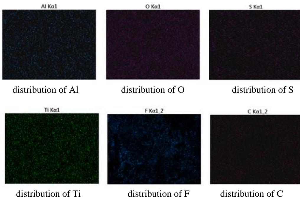
**Figure 2.** EDS spectrum and surface element distribution of anodic oxide film after sealing and surface modification (accelerating voltage 5 kV, surface sweep model, sampling depth 1  $\mu\text{m}$ )
