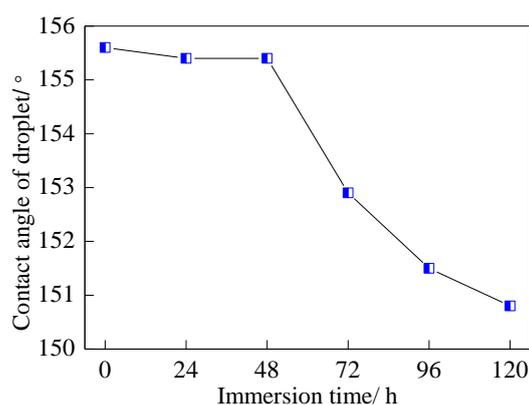
**Figure 6.** Contact angle of water droplets of anodic oxide film after sealing and surface modification during immersion experiment (corrosive medium is 3.5% sodium chloride solution, static immersion for 0~120 h, water volume 4  $\mu$ L, accuracy  $\pm 0.1^\circ$ )
