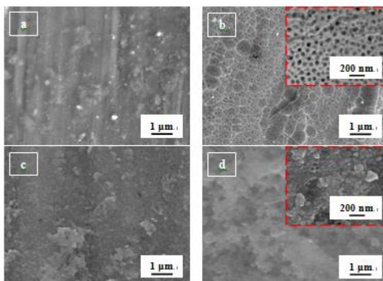
**Figure 1.** Surface morphology of aluminum alloy and different anodic oxide films; a-aluminum alloy, b-anodic oxide film, c-anodic oxide film after sealing, d-anodic oxide film after sealing and surface modification; (sample size 8 mm×8 mm×1 mm, magnification 30000 times, accelerating voltage 10 kV)
