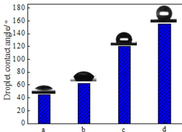
**Figure 3.** Droplet contact angle of aluminum alloy and different anodic oxide films, a-aluminum alloy, b-anodic oxide film, c-anodic oxide film after sealing, d-anodic oxide film after sealing and surface modification (water volume 4  $\mu\text{L}$ , accuracy  $\pm 0.1^\circ$ , sample size 15 mm $\times$ 15 mm)
