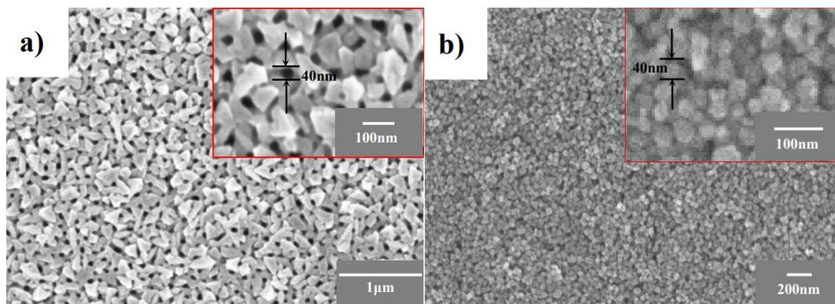
**Figure 1.** Top view of TiO<sub>2</sub> layers in each group, prepared by a) anodizing Ti/FTO substrate and annealing (Group A); b) spin-coating compact and porous TiO<sub>2</sub> films and annealing (Group B). The insets are close-up images of the corresponding group.
