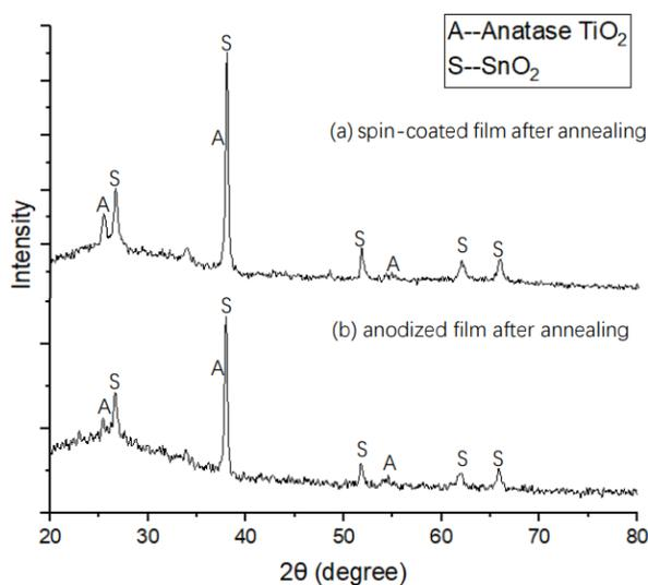
**Figure 4.** XRD patterns for TiO<sub>2</sub> films prepared by (a) anodizing Ti/FTO substrate and annealing; (b) spin-coating compact and mesoporous TiO<sub>2</sub> films and annealing.
