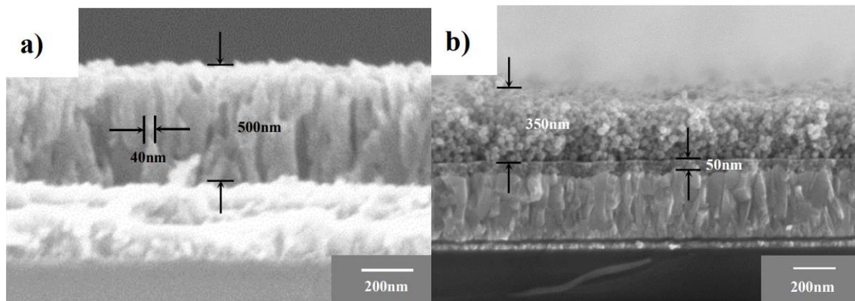
**Figure 2.** Cross-sectional SEM images of TiO<sub>2</sub> layers prepared by a) anodizing Ti/FTO substrate and annealing (Group A); b) spin-coating compact and mesoporous TiO<sub>2</sub> films and annealing (Group B).
