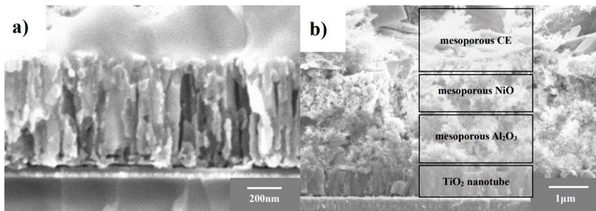
**Figure 3.** Cross-sectional SEM images of anodized PSCs in Group A: a) perovskite crystallized in TiO<sub>2</sub> nanotubes; b) anodized PSC consisting of TiO<sub>2</sub> nanotube/mesoporous Al<sub>2</sub>O<sub>3</sub>/mesoporous NiO/mesoporous CE.
