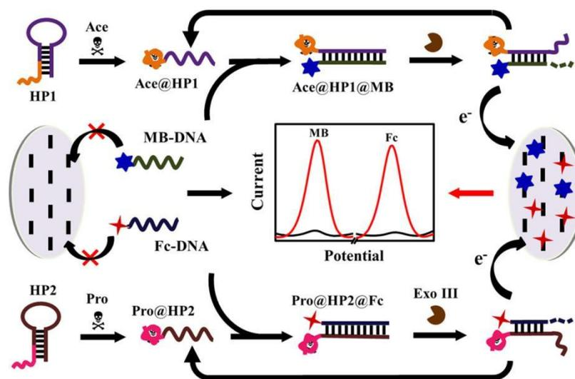
**Figure 4.** Schematic diagram of the electrochemical principle for the simultaneous detection of two pesticides. [77]. [Reprinted with permission from {Aptamer Recognition-Driven Homogeneous Electrochemical Strategy for Simultaneous Analysis of Multiple Pesticides without Interference of Color and Fluorescence}, Copyright {2020} American Chemical Society.]
