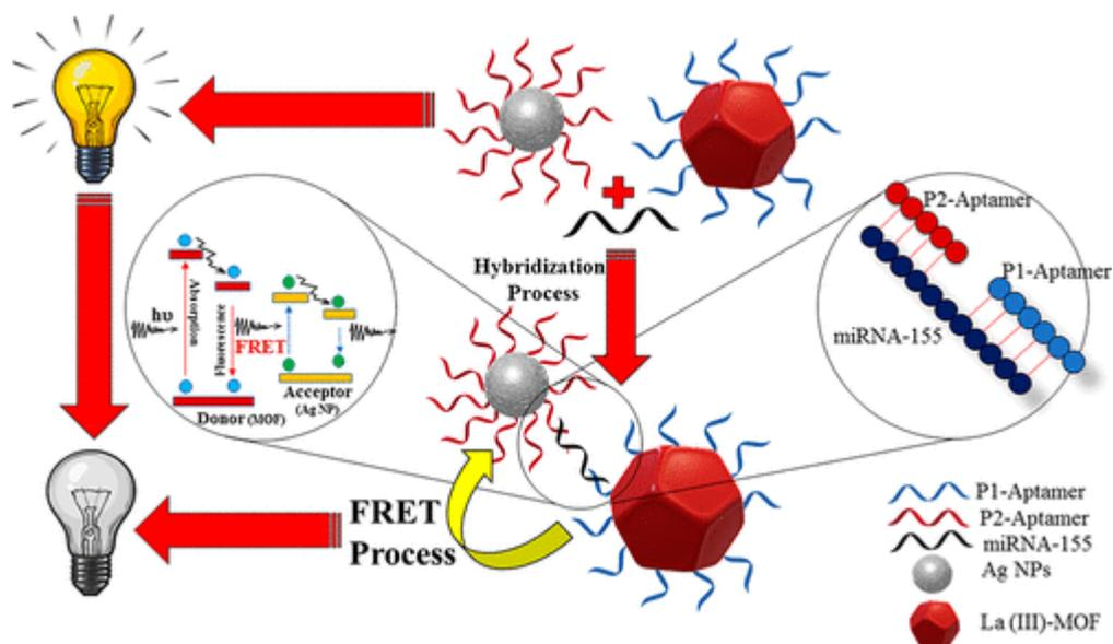
**Figure 3.** Schematic diagram of photoluminescence quenching-based detection of miRNA-155 as a cancer biomarker by the FRET process. [45]. [Reprinted with permission from {Ultrasensitive Fluorescent miRNA Biosensor Based on a “Sandwich” Oligonucleotide Hybridization and Fluorescence Resonance Energy Transfer Process Using an Ln(III)-MOF and Ag Nanoparticles for Early Cancer Diagnosis: Application of Central Composite Design}, Copyright{2020} American Chemical Society.]
