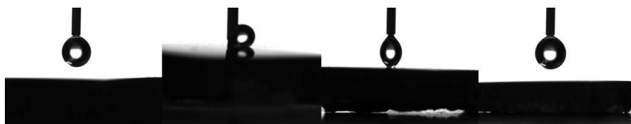
Figure 7. Screen capture of contact angle measurement of nano Ni-P- \text{Al}_2\text{O}_3 (15g/L) coating.
