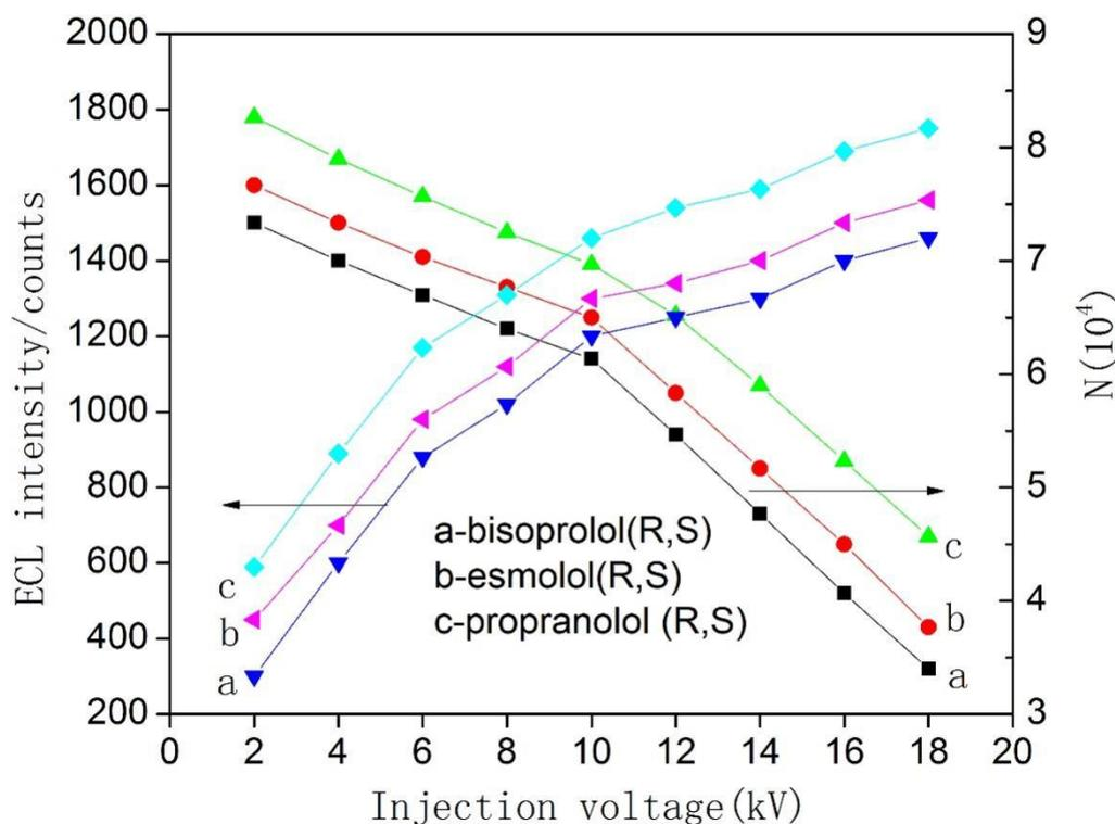
**Figure 5.** The effect of the injection voltage on enantiomers  $R_s$  of 1.5  $\mu\text{g/mL}$  bisoprolol, esmolol, propranolol. Except for the injection voltage, other conditions as Fig. 2.
