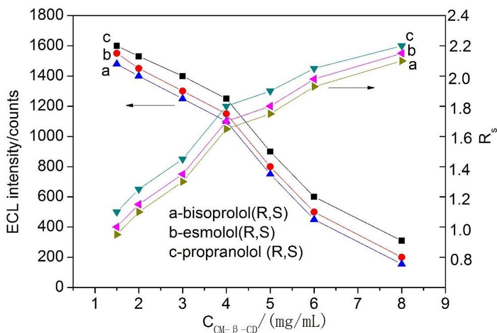
**Figure 2.** The effect of the CM- $\beta$ -CD concentration on enantiomers  $R_s$  of 1.5  $\mu$ g/mL bisoprolol, esmolol, propranolol. Conditions: detection potential: 1.2 V; detection buffer: 5 mM Ru(bpy) $_3^{2+}$ , 65 mM PBS (pH 8.0); separation buffer: 35 mM Tris-H $_3$ PO $_4$  (pH 8.5). separation voltage: 12 kV; electrokinetic injection: 10 kV $\times$ 12 s.
