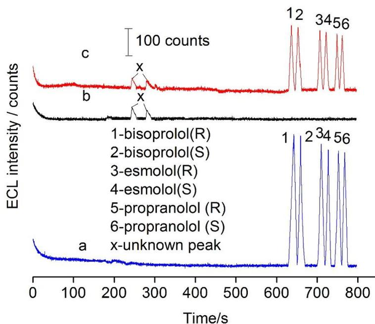
**Figure 6.** The electropherograms of the enantiomers separation for bisoprolol, esmolol, propranolol. a. 0.5  $\mu\text{g/mL}$  bisoprolol, esmolol, propranolol standard solutions; b. the blank urine; c. b spiked with 0.25  $\mu\text{g/mL}$  bisoprolol, esmolol, propranolol standard solutions; 4mg/mL CM- $\beta$ -CD, other conditions as Fig. 2.
