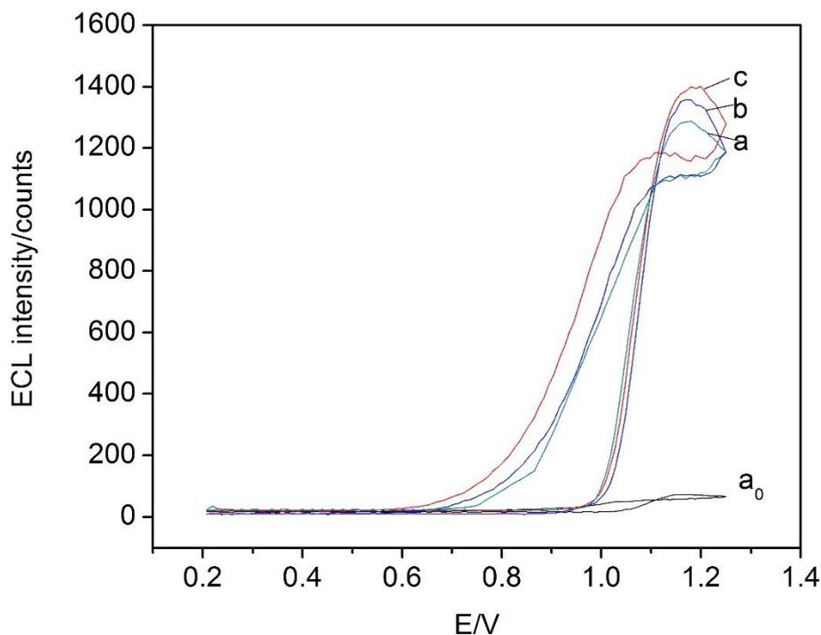
**Figure 1.** ECL behaviors of bisoprolol (a), esmolol (b) and propranolol (c) a<sub>0</sub>. 65 mM PBS (pH8.0) +5 mM  $\text{Ru}(\text{bpy})_3^{2+}$ ; a. a<sub>0</sub>+1.5  $\mu\text{g}/\text{mL}$  bisoprolol; b. a<sub>0</sub>+1.5  $\mu\text{g}/\text{mL}$  esmolol; c. a<sub>0</sub>+1.5  $\mu\text{g}/\text{mL}$  propranolol
