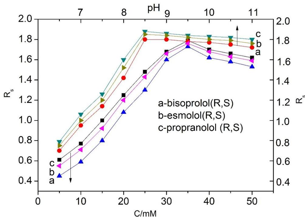
**Figure 4.** The effect of the separation buffer pH and concentration on enantiomers  $R_s$  of 1.5  $\mu\text{g/mL}$  bisoprolol, esmolol, propranolol. Except for the separation buffer pH and concentration, other conditions as Fig. 2.
