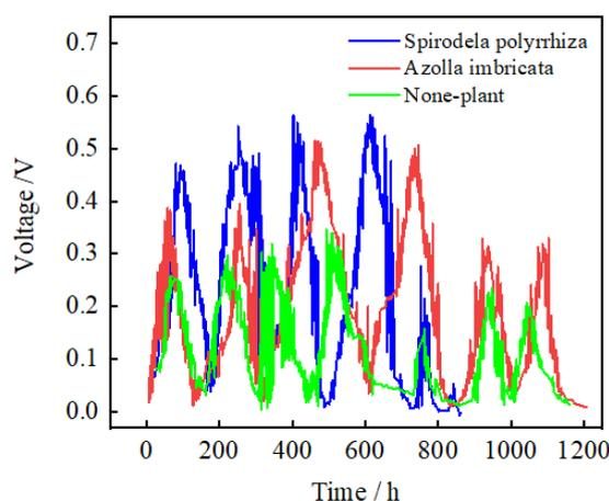
**Figure 3.** Voltage diagram of operation phase. Hydraulic retention time was selected as 15, 10 and 5 h in this experiment.
