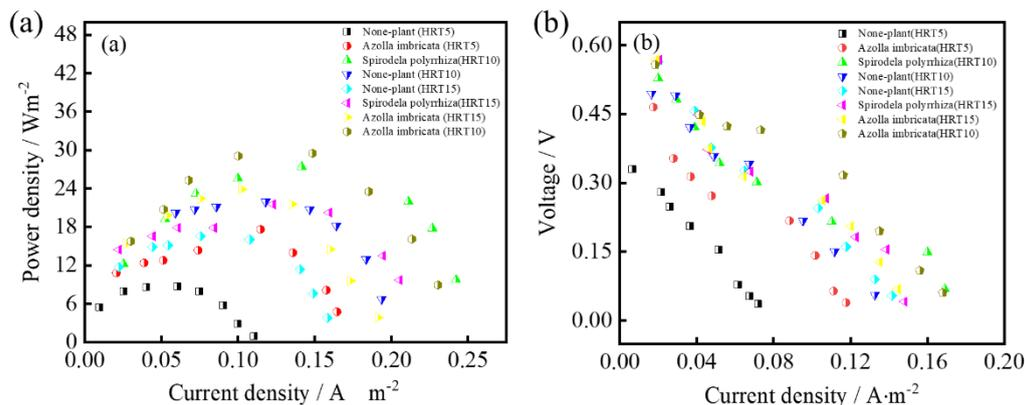
**Figure 4.** Effect of different plants on reactor (a) power density and (b) polarization curves under different HRTs.
