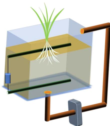
**Figure 1.** Schematic of a plant microbial fuel cell.
