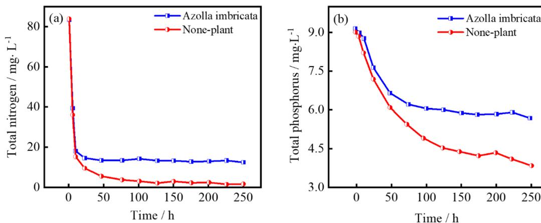
**Figure 6.** Influence of plant on the change of (a) total nitrogen and (b) phosphorus in the reaction process.
