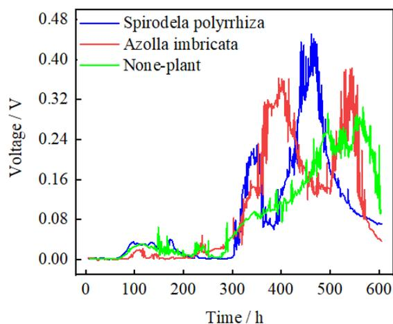
**Figure 2.** Voltage diagram during operation. The voltage of the external resistance is recorded every 5 min and measured by a multi-channel data acquisition instrument (model 2700, Keithley Inc, USA).
