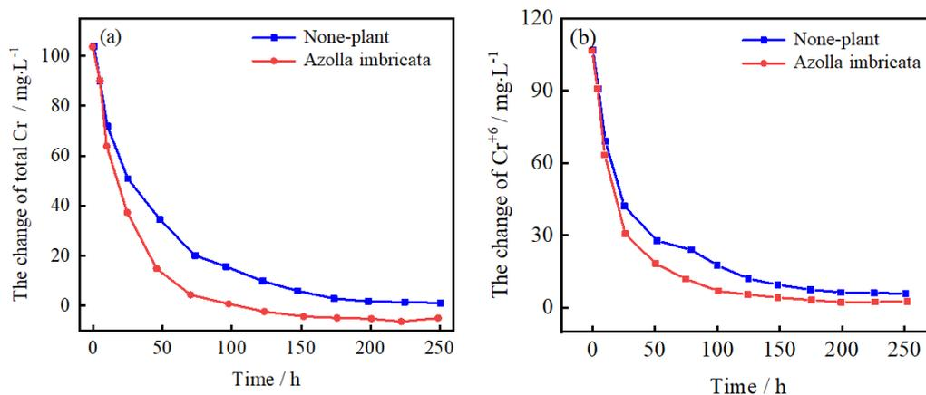
**Figure 7.** Changes in (a) total and (b) hexavalent chromium concentrations after adding *Azolla imbricata*.
