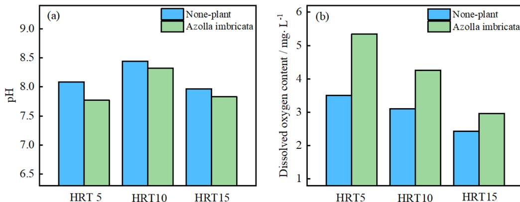
**Figure 5.** Influence of plant on the change of (a) pH and (b) dissolved oxygen in the reaction process.
