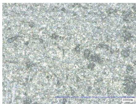
**Figure 6.** The surface morphology of 304SS after accelerated corrosion of stainless steel concrete after 60 days of immersion
