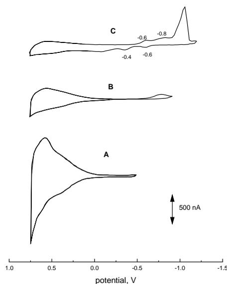
**Figure 2.** The background current of 0.1 M NaOH at CS at different potential windows starting at +0.75 V to -0.5 V (A), -1.0 V (B) and -1.2 V(C) respectively at 10 Vs<sup>-1</sup> vs SCE. The current was measured after 50 cycles in each potential window.
