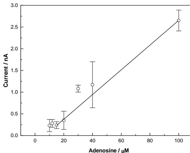
**Figure 9.** ADO calibration curve at CS after 100 cycles in 0.1  $\text{mol L}^{-1}$  NaOH, scan rate 100  $\text{Vs}^{-1}$ , the potential window is between +0.6 and 0.0 V. Currents measured at + 0.53 V.
