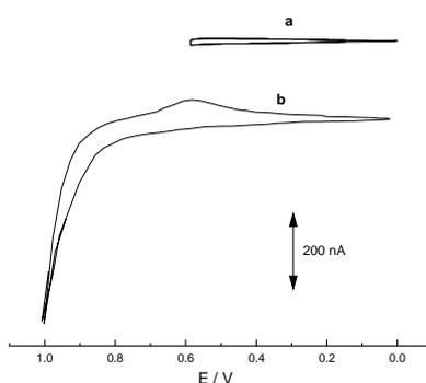
**Figure 3.**  $0.1 \text{ mol L}^{-1}$  NaOH background current at copper sensor at potential windows from 0.0 to +0.6 V (a) and to +1.0 V (b) respectively. The measured current is the average value for 50 cycles at  $10 \text{ V s}^{-1}$  vs SCE.
