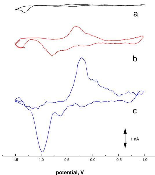
**Figure 6.** 10 mM adenosine in  $70 \text{ mmol L}^{-1}$  phosphate buffer pH 7.4 at CFS at different scan rates after 100 cycles: (a)  $10 \text{ Vs}^{-1}$ ; (b)  $100 \text{ Vs}^{-1}$  and (c)  $500 \text{ Vs}^{-1}$  vs SCE.
