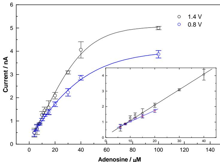
**Figure 7.** Adenosine calibration curves at CFS in 70 mmol L<sup>-1</sup> phosphate buffer pH 7.4, measured at +1.4 and +0.8 V with a scan rate of 100 V s<sup>-1</sup> vs SCE after 100 cycles. Inside Figure shows the linear dynamic range at both potential values (+0.8 V and + 1.4 V).
