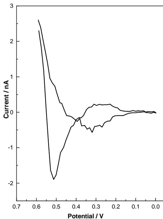
**Figure 8.** 100 mM adenosine at CS in 0.1 mol L<sup>-1</sup> NaOH, after 100 cycles at 100 V s<sup>-1</sup> vs SCE.
