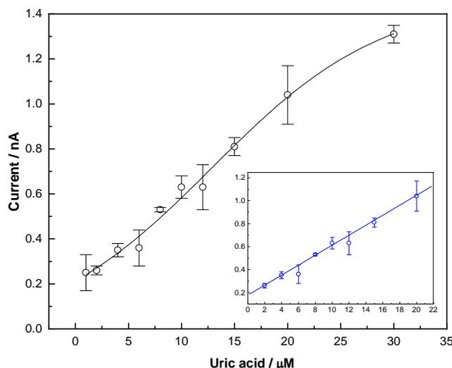
**Figure 5.** Analytical curve for UA at CFS, in 70 mmol L<sup>-1</sup> phosphate buffer pH 7.4, at 100 V s<sup>-1</sup> vs SCE, 100 cycles. Inside Figure represents the LDR.
