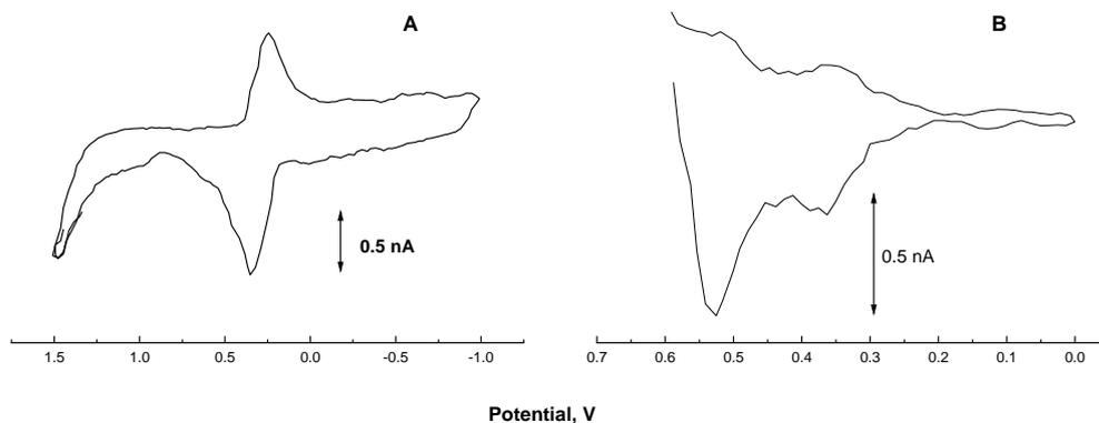
**Figure 4.** **A:** Cyclic Voltammogram of  $30 \text{ mM UA}$  in  $70 \text{ m mol L}^{-1}$  phosphate buffer pH 7.4, at CFS, scan rate is  $100 \text{ V s}^{-1}$  vs SCE after 100 cycles. **B:** Cyclic Voltammograms of  $10 \text{ mM UA}$  in  $0.1 \text{ M NaOH}$ , at CS, scan rate is  $100 \text{ Vs}^{-1}$  vs SCE after 100 cycles.
