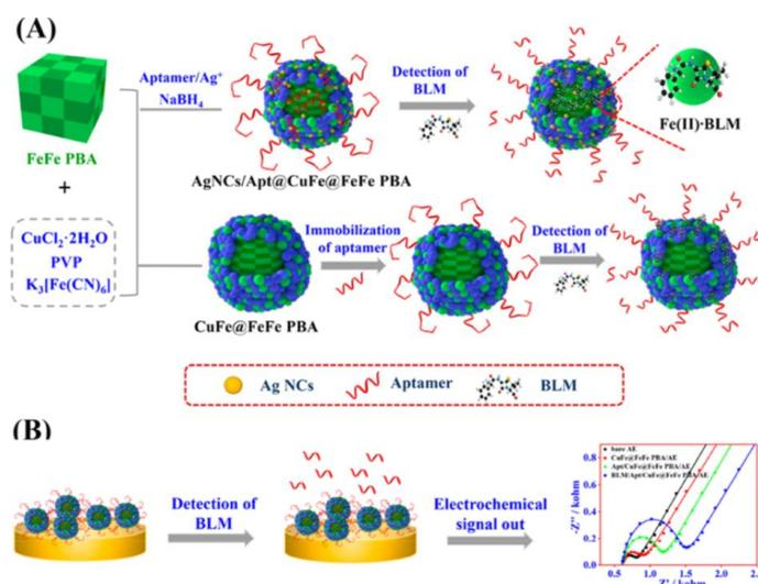
**Figure 14.** Schematic diagram of (A) the fabrication of BLM aptasensors based on AgNCs/Apt@CuFe@FeFe PBA and CuFe@FeFe PBA and (B) BLM detection and electrochemical signal out. Reprinted with permission from reference [61]. Copyright 2018 American Chemical Society.
