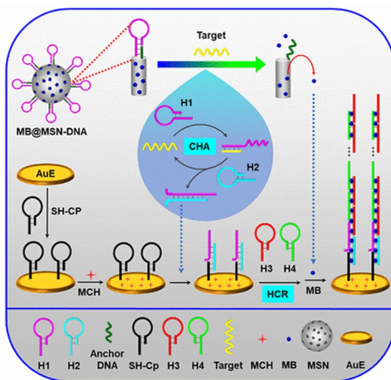
**Figure 8.** Schematic diagram of mesoporous silica containers and programmed catalytic hairpin assembly hybridization chain reaction based electrochemical sensing platform for miRNA ultrasensitive detection with low background. Reprinted with permission from reference [31]. Copyright 2019 American Chemical Society.
