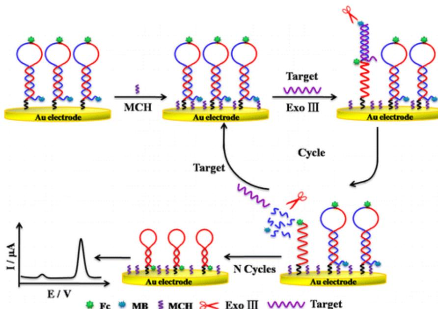
**Figure 2.** Schematic illustration of the electrochemical biosensor for target DNA detection. Reprinted with permission from reference [11]. Copyright 2015 American Chemical Society.
