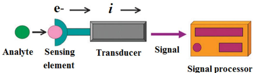
**Figure 1.** Schematic of a biosensor with electrochemical transducer.
