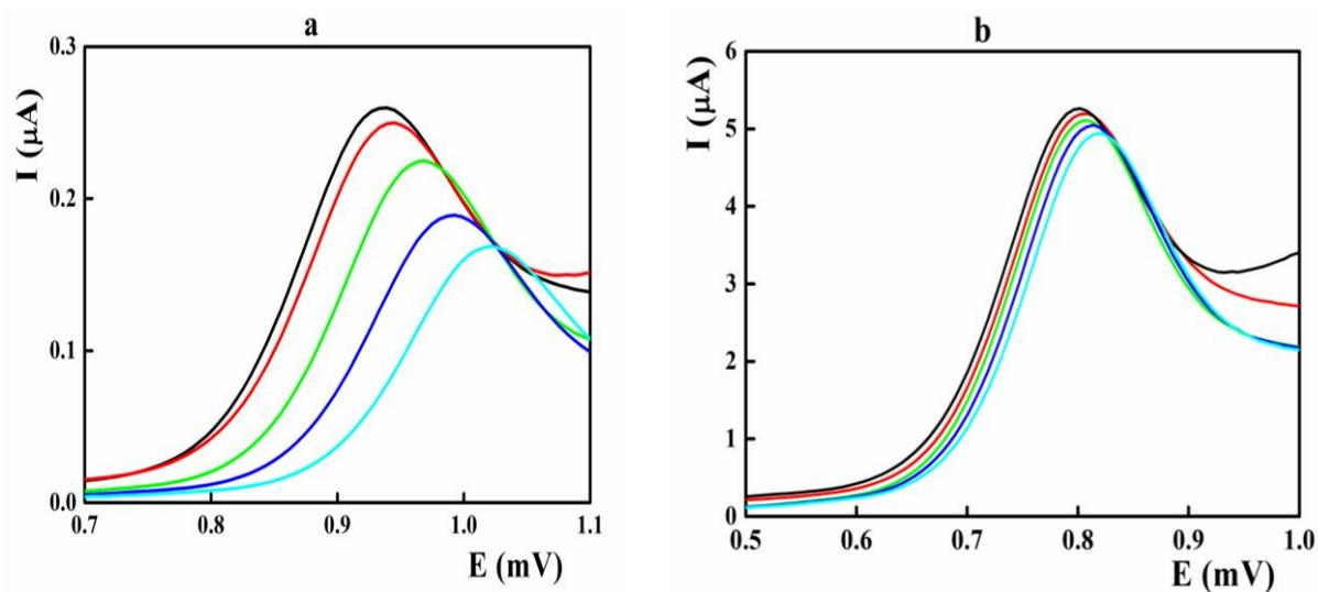
**Figure S2.** Successive differential pulse voltammograms of  $275 \text{ ng mL}^{-1}$  CLO on 7.5% zeolite based carbon paste electrode at pH 10.0. Scan rate  $40 \text{ mV s}^{-1}$
