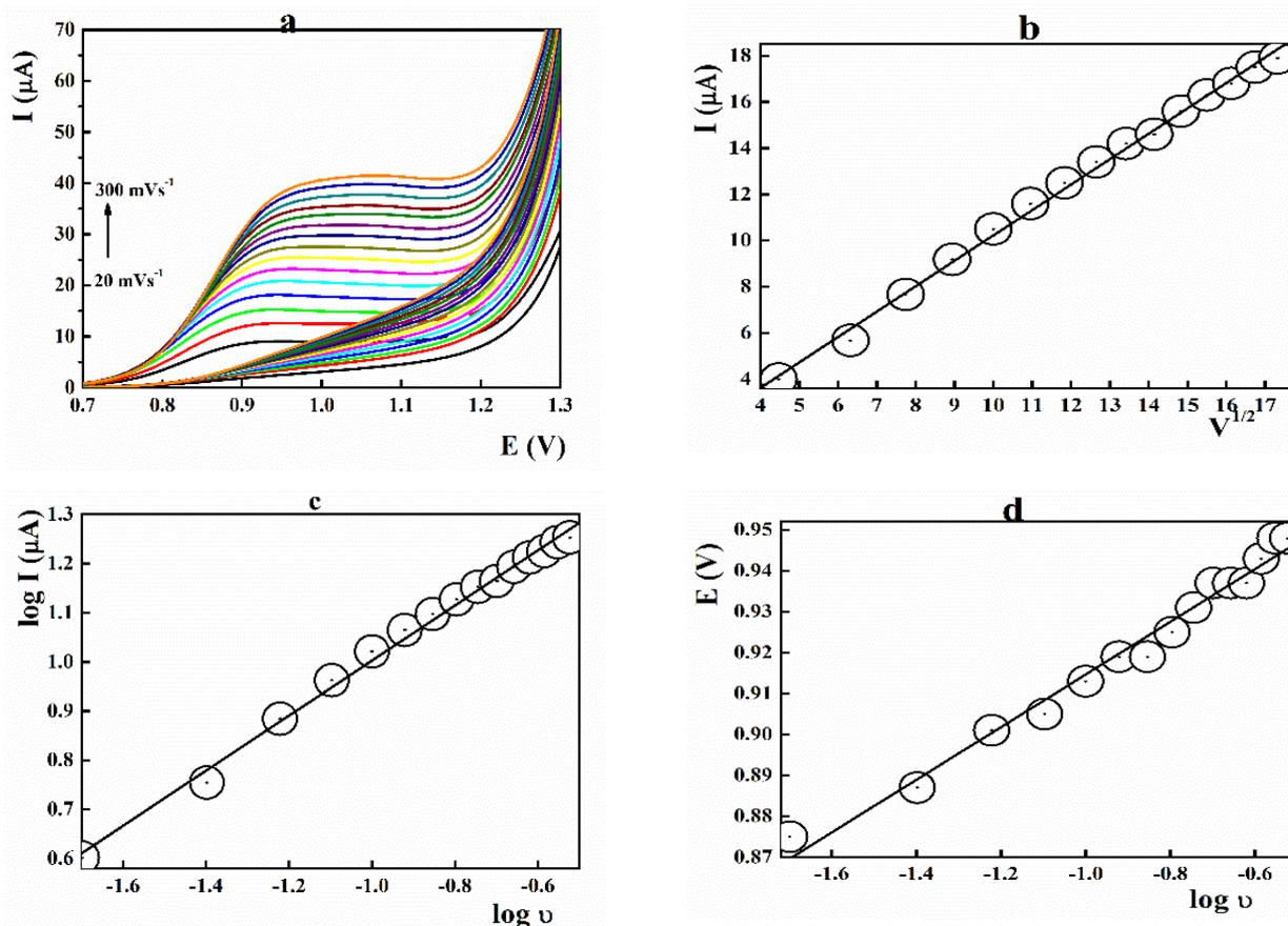
**Figure 3.** Voltammetric behavior of 275 ng mL<sup>-1</sup> cyclopentolate at different scan rate values using 7.5% ZY/CPE at pH 10.0
