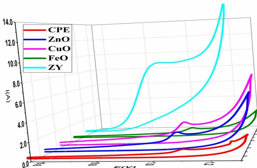
**Figure S1.** Voltammetric behavior of 275 ng mL<sup>-1</sup> cyclopentolate using carbon paste electrode modified with different nanostructures at pH 10.0. Scan rate 40 mV s<sup>-1</sup>.
