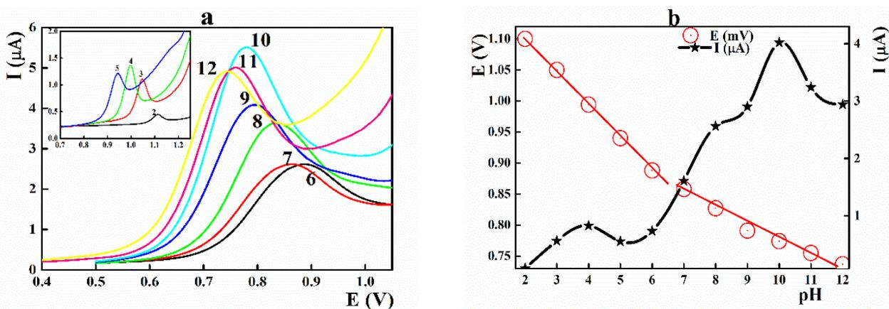
**Figure 2.** a) Differential pulse voltammograms of 275 ng mL<sup>-1</sup> cyclopentolate at different pH values on 7.5 % zeolite based carbon paste electrode; b) peak currents and peak potentials against pH. Scan rate was 0.040 V s<sup>-1</sup>
