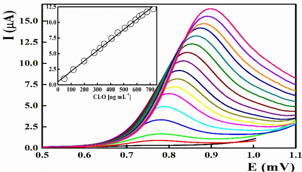
**Figure 4.** Differential pulse voltammetric determination of cyclopentolate using 7.5% ZY/CPE in BR buffer at pH 10.0 with scan rate  $0.040\text{V s}^{-1}$ .
