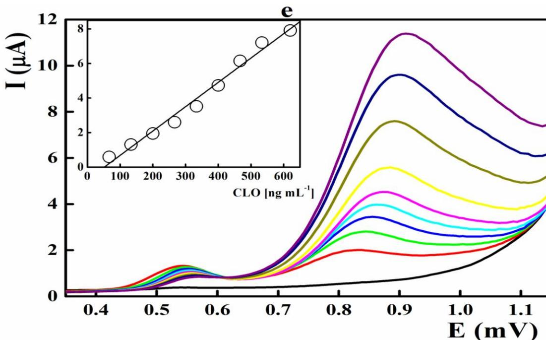
**Figure 5.** Simultaneous voltammetric determination of cyclopentolate and phenylephrine on 7.5% zeolite based carbon paste electrode; a, b) at pH 6.0, c, d) at pH 10.0; e) differential pulse voltammetric determination of CLO on Zy/CPE at pH 10.0 in presence of phenylephrine
