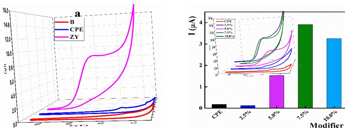
**Figure 1.** Voltammetric behavior of 275 ng mL<sup>-1</sup> cyclopentolate on ZY/CPE in BR buffer at pH 10. Scan rate 40 mV s<sup>-1</sup>.
