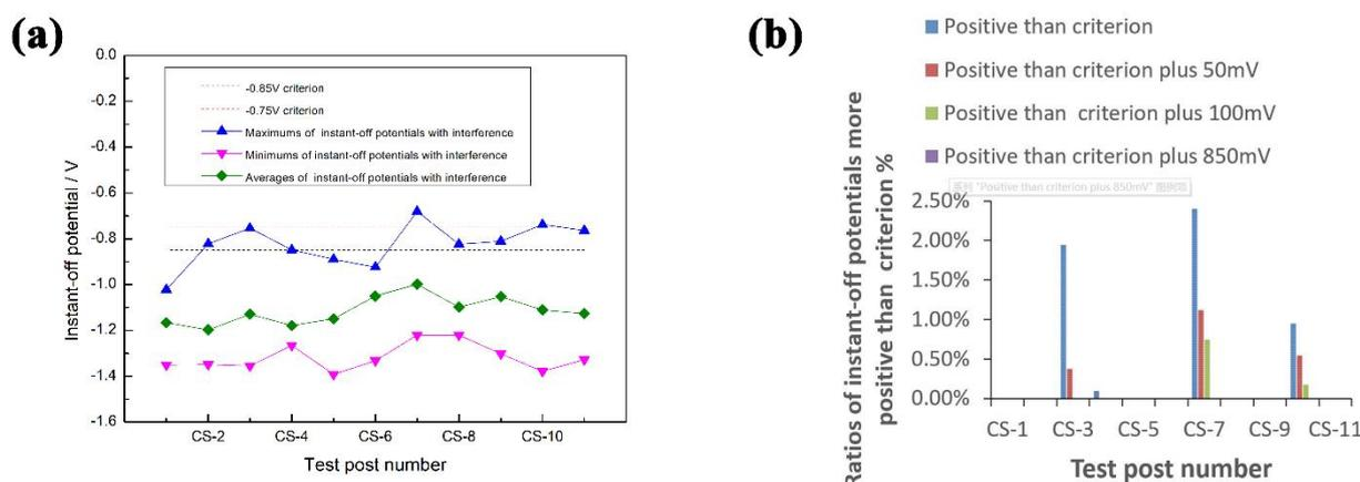
**Figure 7.** Extremes and averages of the instant-off potentials of the pipeline under 15 A cathodic current with DC interference (a). (b) Ratios of the instant-off potentials that fail to meet the cathodic protection criteria obtained at each test post with 15 A cathodic current. CS-1 to CS-11 signify the numbers of the test posts along the pipeline.
