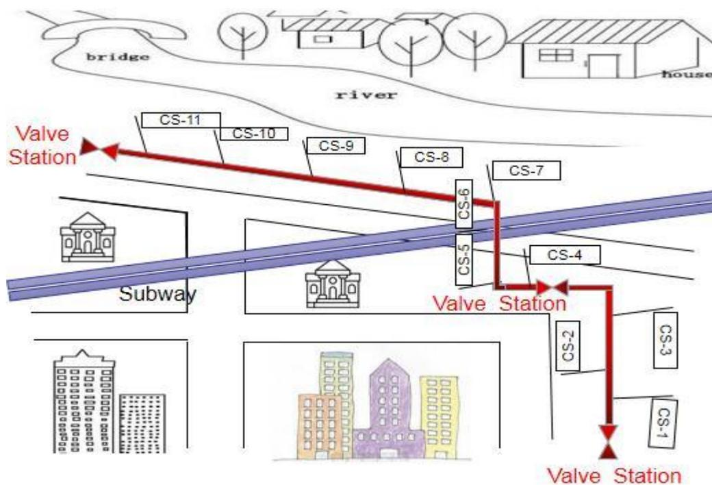
**Figure 4.** Comparative distribution of gas pipeline and subway lines No. 2, CS-1 to CS-11 signify the numbers of the test posts along the pipeline.
