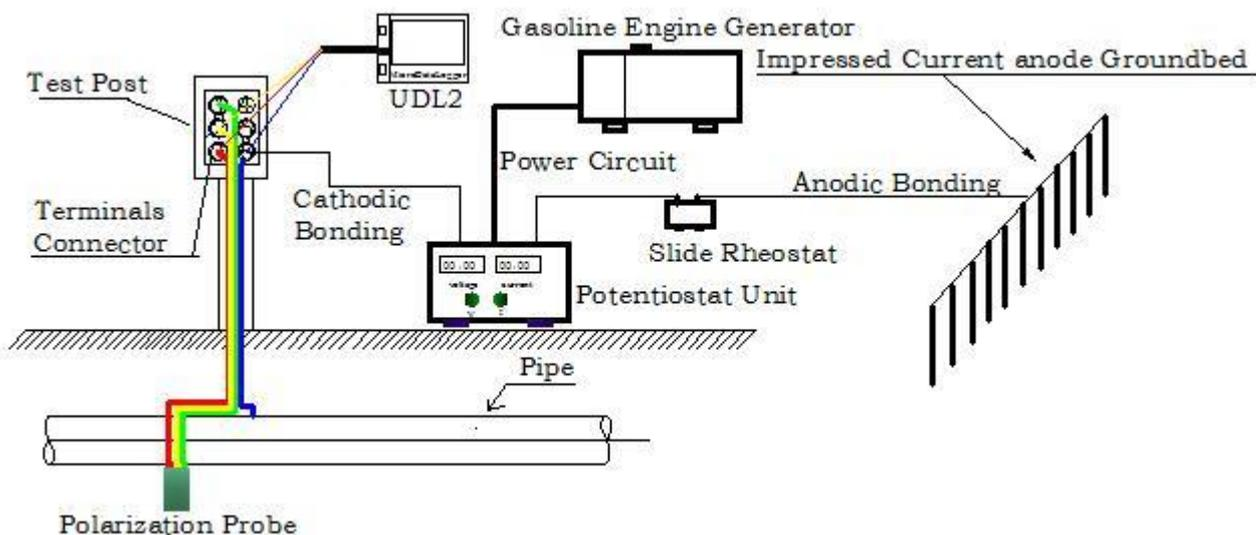
**Figure 3.** Connection diagram of the current requirement test.
