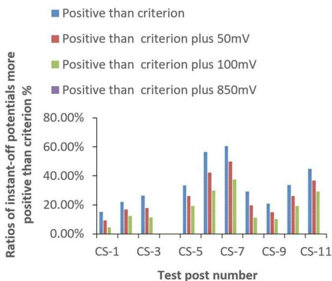
**Figure 6.** Ratios of the instant-off potentials that fail to meet the cathodic protection criteria obtained at each test post. CS-1 to CS-11 signify the numbers of the test posts along the pipeline.
