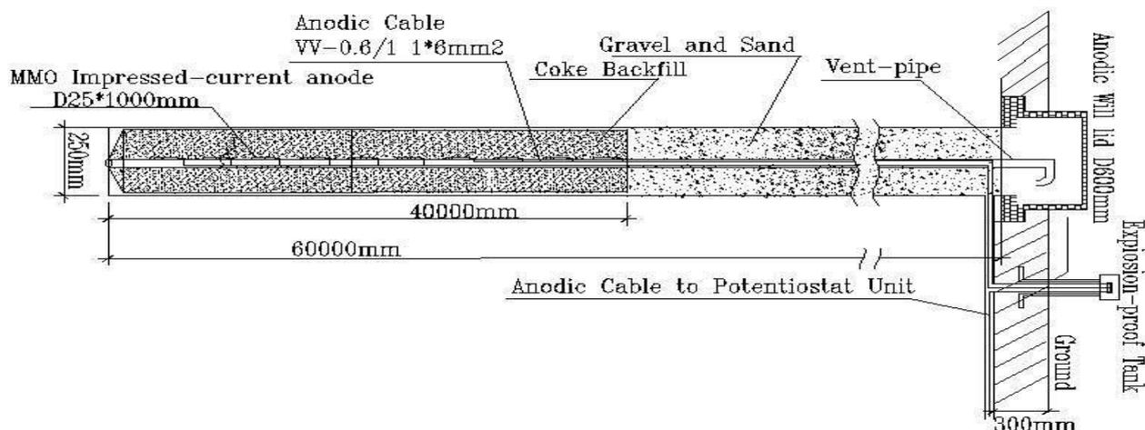
**Figure 8.** Schematic of the anode body [26].
