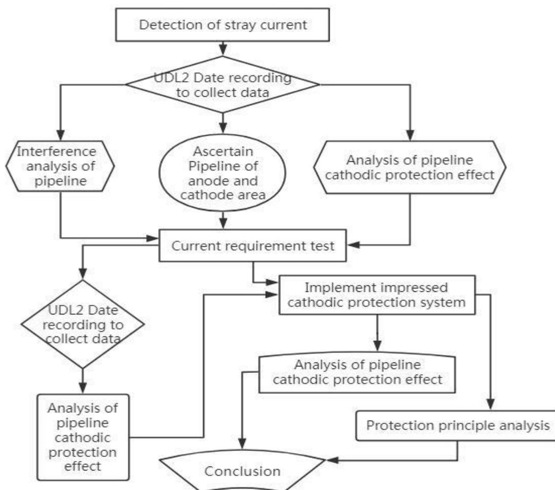
**Figure 1.** Implementation process of the analysis of an impressed current cathodic protection (ICCP) system.
