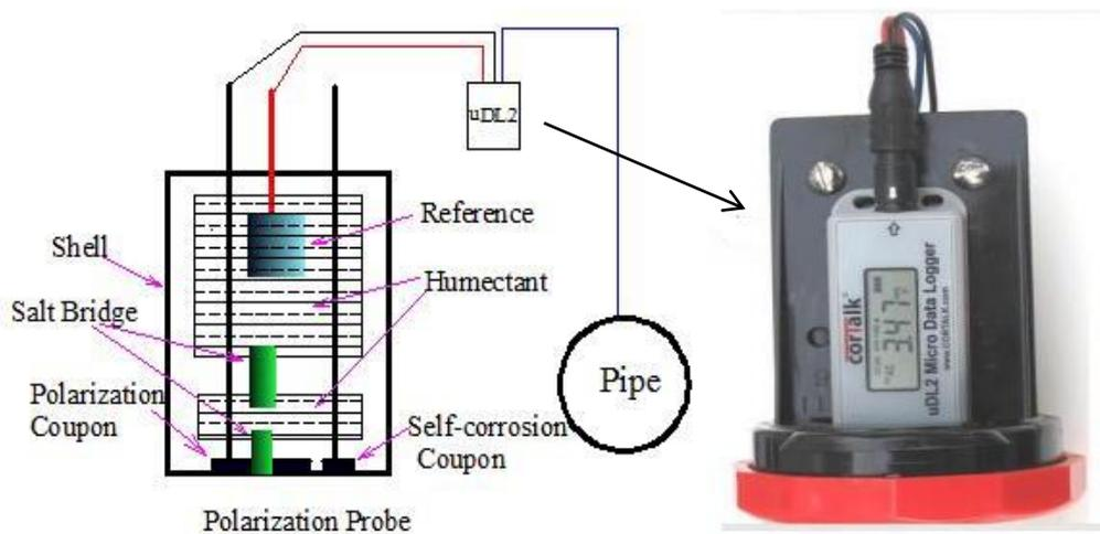
**Figure 2.** Schematic of the stray current testing system.
