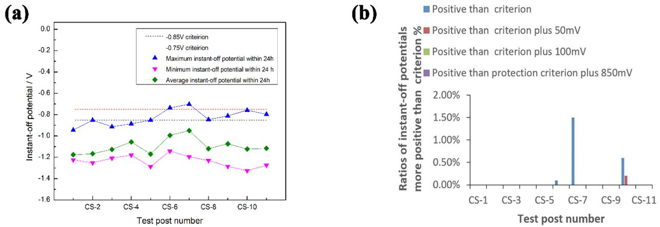
**Figure 9.** Extremes and averages of the instant-off potentials of the pipeline under 15 A cathodic current within 24 h (a). (b) Ratios of the instant-off potentials that fail to meet the cathodic protection criteria obtained at each test post with 15 A of cathodic current. CS-1 to CS-11 signify the numbers of the test posts along the pipeline.
