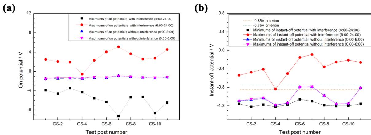
**Figure 5.** Extremes of the on (a) and instant-off (b) potentials of the pipeline monitored within 24 h of the absence and presence of stray DC interference. CS-1 to CS-11 signify the numbers of the test posts along the pipeline.
