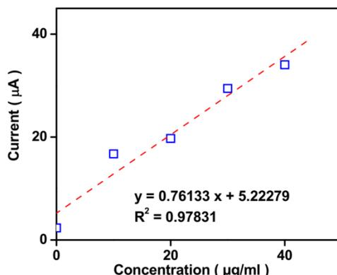
**Figure 5.** The calibration plot of electrochemical CV responses of PdNPs/SWCNTs to successive addition 10µg/ml of aspartame solutions in potential range from -0.3V to 0.3V at 20 mV/s scan rate in 0.1M PBS pH 7.0
