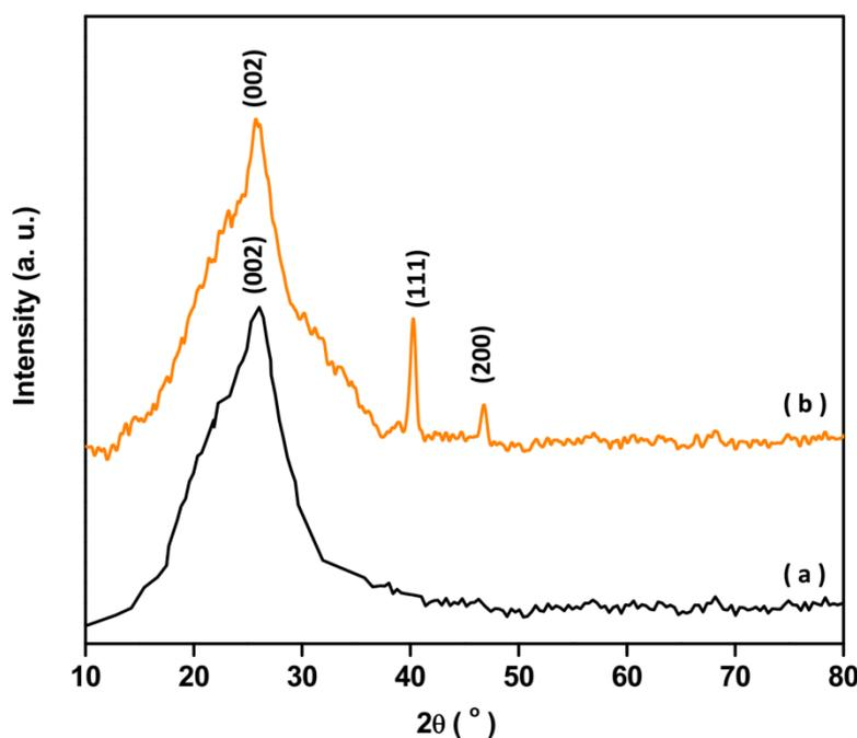
**Figure 2.** XRD patterns of the prepared (a) SWCNTs and (b) PdNPs/SWCNTs films.
