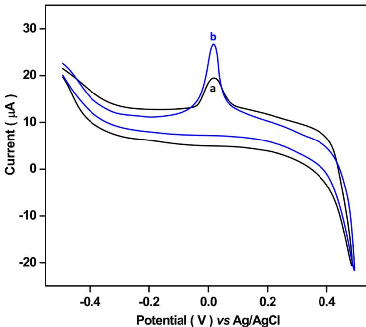
**Figure 3.** The first recorded CV of (a) SWCNTs and (b) PdNPs/SWCNTs electrodes in potential range from -0.5V to 0.5V at 20 mV/s scan rate in 0.1M PBS pH 7.0 containing 40 µM aspartame.
