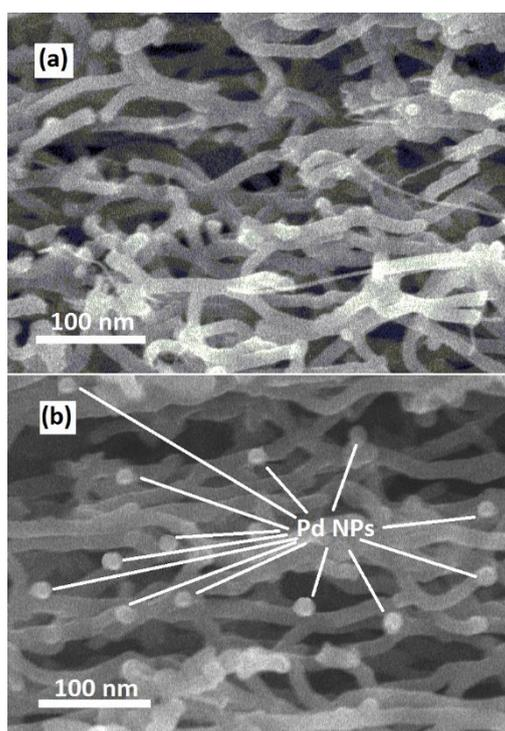
**Figure 1.** SEM images of the prepared (a) SWCNTs and (b) PdNPs/SWCNTs films.
