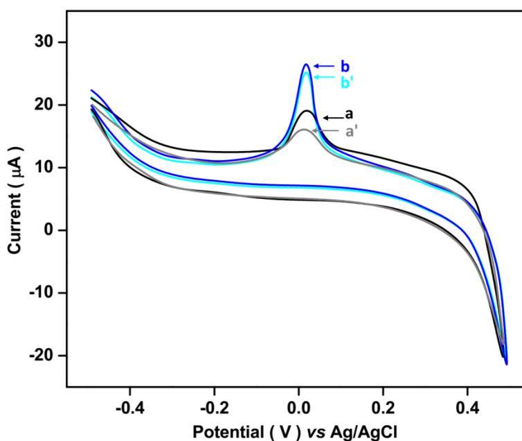
**Figure 4.** The first recorded CV of (a) SWCNTs and (b) PdNPs/SWCNTs electrodes, and 50<sup>th</sup> recorded CV of (a') SWCNTs and (b') PdNPs/SWCNTs electrodes in potential range from -0.5V to 0.5V at 20 mV/s scan rate in 0.1M PBS pH 7.0 containing 40 µM aspartame.
