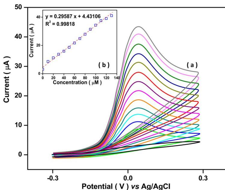
**Figure 5.** (a) Electrochemical CV response and (b) calibration plot of PdNPs/SWCNTs electrode to various concentration of aspartame in potential range from -0.3V to 0.3V at 20 mV/s scan rate in 0.1M PBS pH 7.0.
