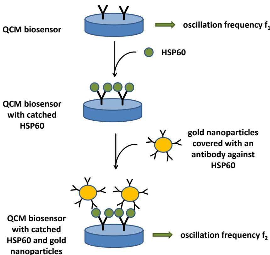
**Figure 2.** General principle of the QCM biosensor assay.
