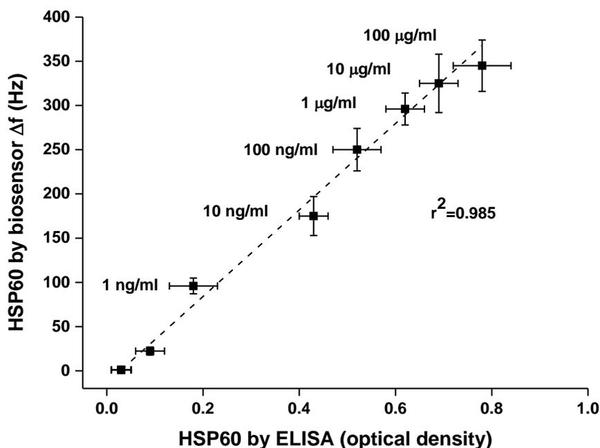
**Figure 4.** Comparison between biosensor and ELISA measurements of HSP60 containing samples. The point in brackets was obtained by blank assay. Error bars indicate standard deviation for five repeats of measurement (a sample assayed by five biosensors or five wells of ELISA microplate).
