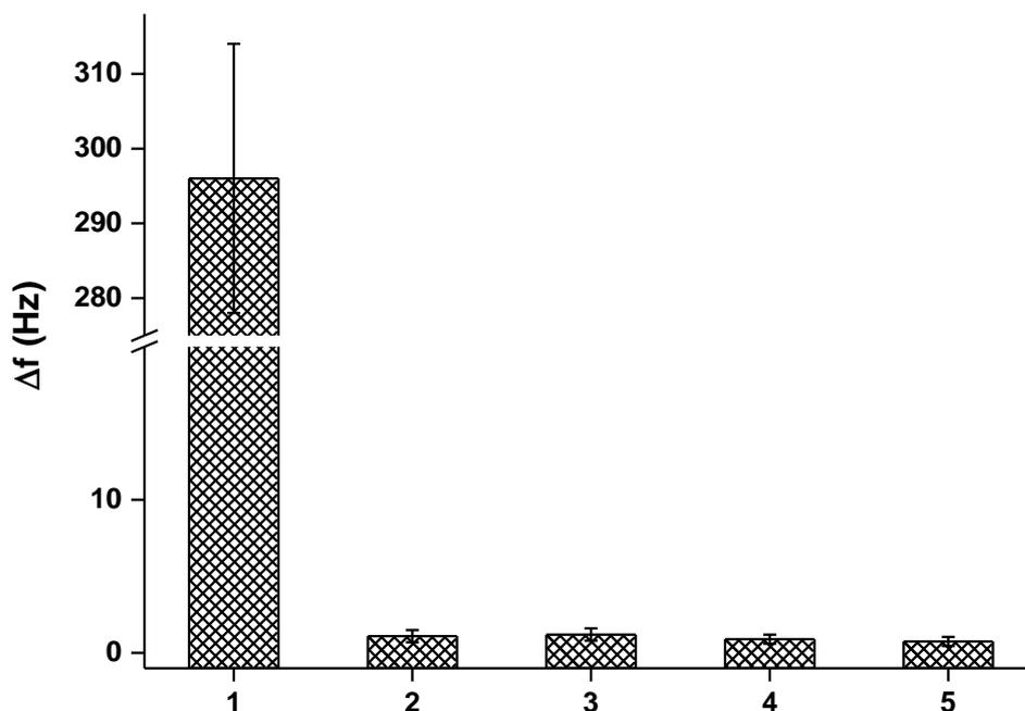
**Figure 5.** Testing of interferences caused by HSP70 100  $\mu\text{g/ml}$  (column 2), albumin 100  $\text{mg/ml}$  (column 3), IgG 100  $\text{mg/ml}$  (column 4) and PBS (column 5) while column 1 is a signal for HSP60 1  $\mu\text{g/ml}$ . Error bars indicate standard deviation for five repeats of measurement (a sample measured by five biosensors).
