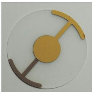
**Figure 1.** A 10 MHz QCM used for biosensor manufacturing.
