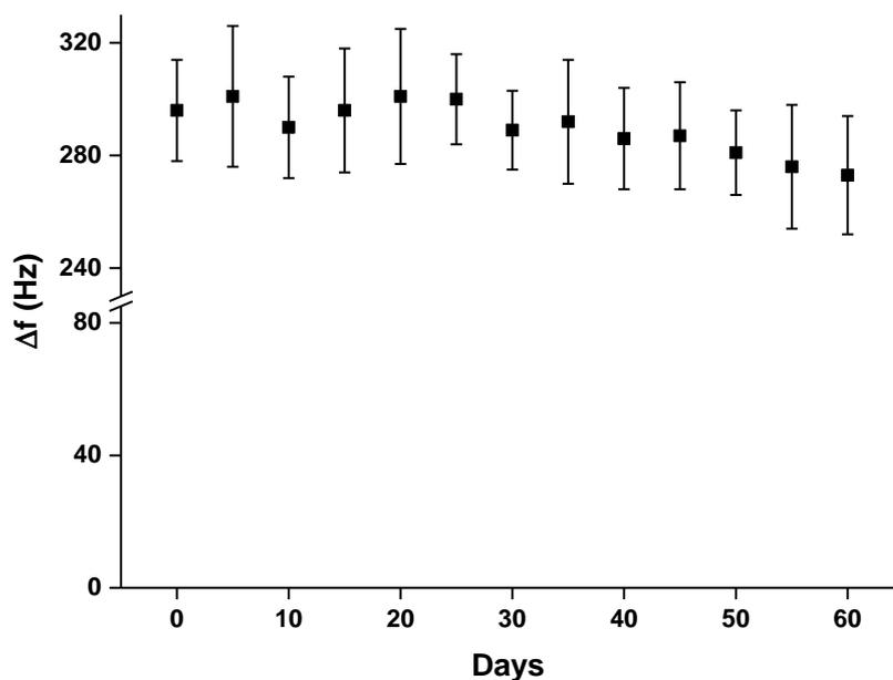
**Figure 6.** Long term stability of the tested biosensors and modified gold nanoparticles. Error bars indicate standard deviation for five repeats of measurement (a sample measured by five biosensors).
