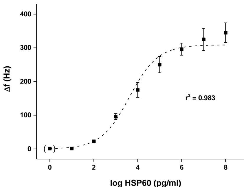
**Figure 3.** Calibration of QCM biosensor for HSP60 assay. Decimal logarithm used for HSP60 concentration expression. The point in brackets was obtained by blank assay. Error bars indicate standard deviation for measurement of a sample by five biosensors.
