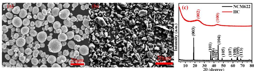
**Figure 2.** SEM images of (a) NMC622 and (b) HC and (c) XRD patterns of NMC622 and HC.
