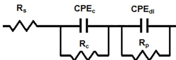
**Figure 3.** The used equivalent circuit for fitting of EIS data
