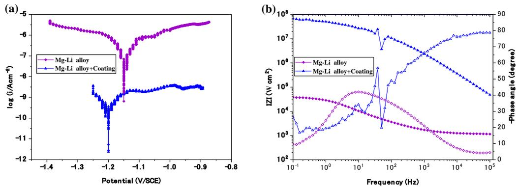
**Figure 2.** Potentiodynamic polarization curves and EIS plots of the bare and coated samples in 3.5 wt% NaCl solution: (a) potentiodynamic polarization curves, (b) EIS plots.
