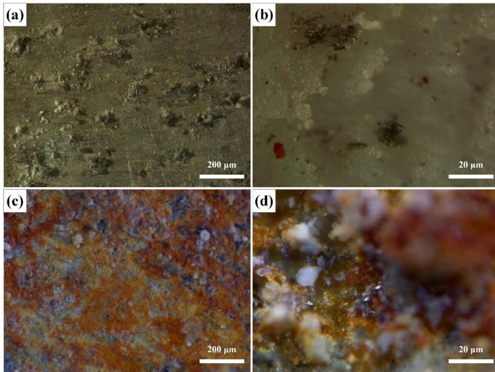
**Figure 3.** OM images in 3.5 wt% NaCl solution of bare alloy((a) and (b)) and coated samples ((c) and (d)).
