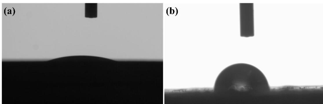
Figure 6. Contact angles of substrate, and coating/substrate
