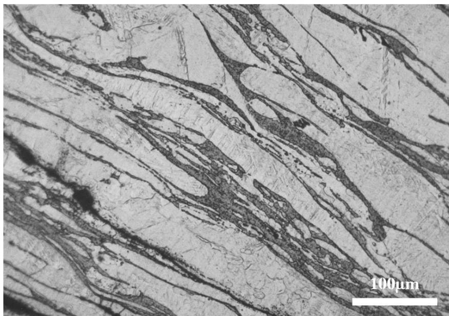
**Figure 1.** OM images of extruded Mg-7Li-3Al-1Si alloy
