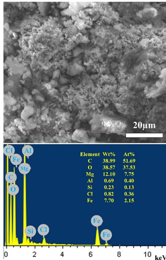
Figure 5. SEM images and EDS of bare alloy (a) and coated samples (b).
