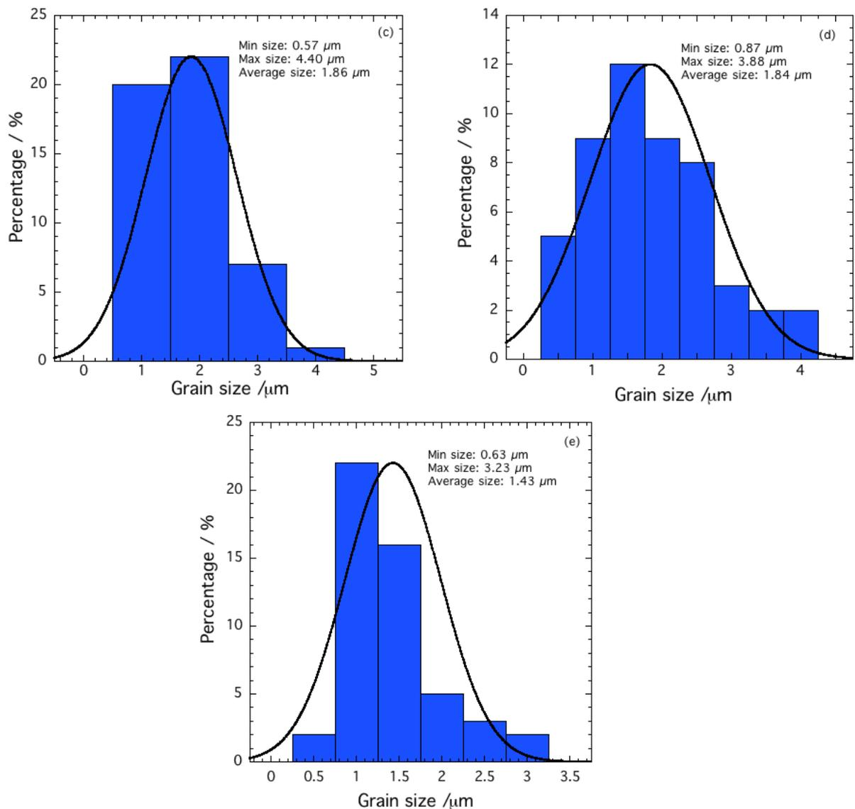
**Figure 4.** Histogram of grain size distribution of  $(Y_{1-x}Yb_x)Ba_2Cu_3O_{7-\delta}$  for (a)  $x = 0$ , (b)  $x = 0.2$ , (c)  $x = 0.5$ , (d)  $x = 0.7$  and (e)  $x = 1.0$ .
