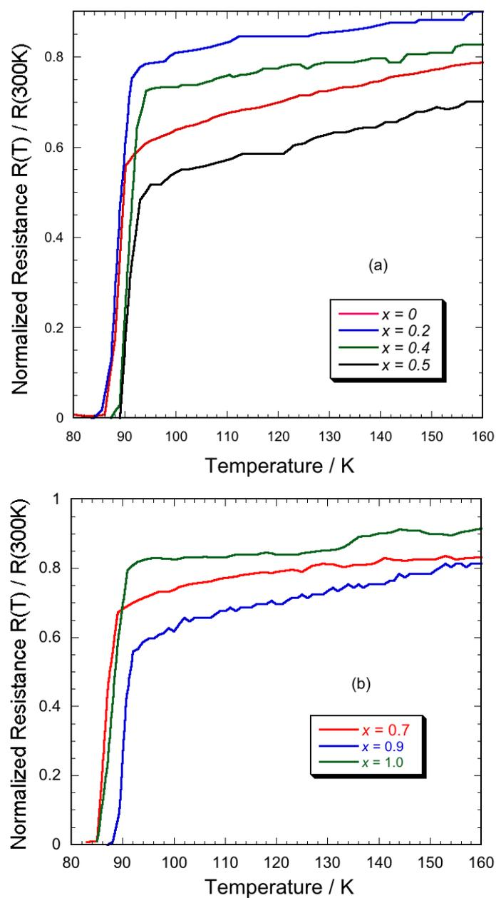
**Figure 5.** Electrical resistance temperature dependence of  $(Y_{1-x}Yb_x)Ba_2Cu_3O_{7-\delta}$  for (a)  $x = 0, 0.2, 0.4, 0.5$  and (b)  $x = 0.7, 0.9, 1.0$ .
