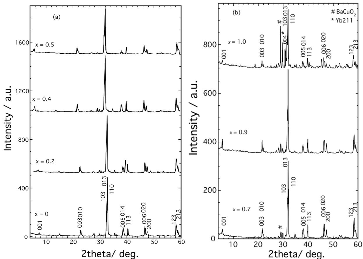
**Figure 1.** Powder X-ray diffraction patterns of  $(Y_{1-x}Yb_x)Ba_2Cu_3O_{7-\delta}$  for (a)  $x = 0, 0.2, 0.4, 0.5$  and (b)  $x = 0.7, 0.9, 1.0$ . Impurities: # -  $BaCuO_2$  and \* -  $Yb_2O_3$ .
