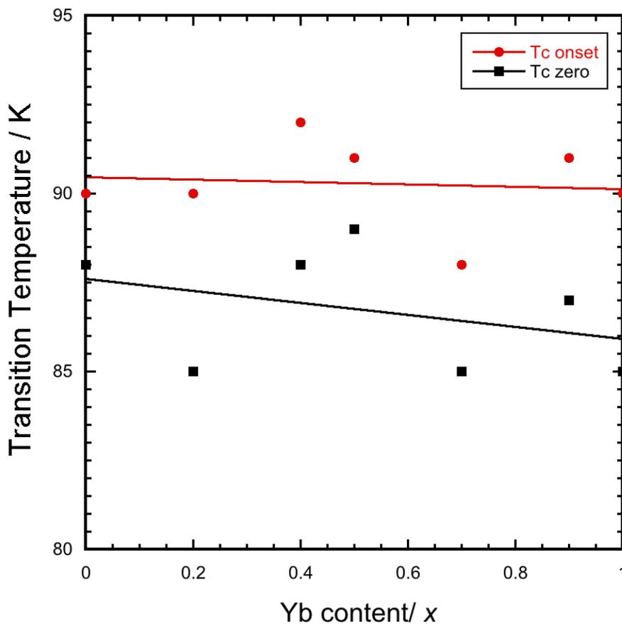
**Figure 6.** The variation of  $T_{c-zero}$  and  $T_{c-onset}$  as a function of  $x$  for  $(Y_{1-x}Yb_x)Ba_2Cu_3O_{7-\delta}$ . The solid lines are linear fits that show a decreasing trend in the transition temperature.
