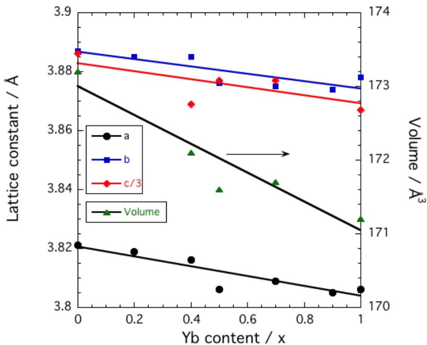
**Figure 2.** Lattice parameters and unit cell volume versus  $x$  for  $(Y_{1-x}Yb_x)Ba_2Cu_3O_{7-\delta}$
