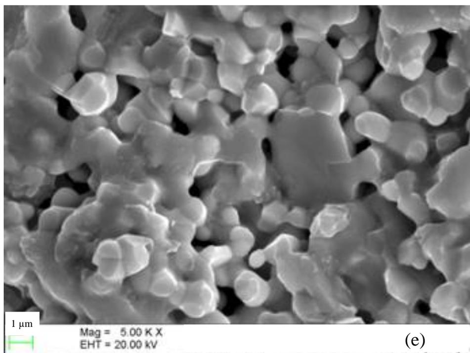
**Figure 3.** Scanning electron micrographs of  $(Y_{1-x}Yb_x)Ba_2Cu_3O_{7-\delta}$  for (a)  $x = 0$ , (b)  $x = 0.2$ , (c)  $x = 0.5$ , (d)  $x = 0.7$ , (e)  $x = 1.0$
