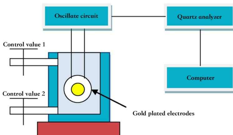
**Figure 6.** Block diagram of testing system
