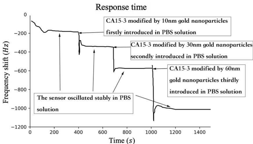
**Figure 11.** Response time of QCM sensor
