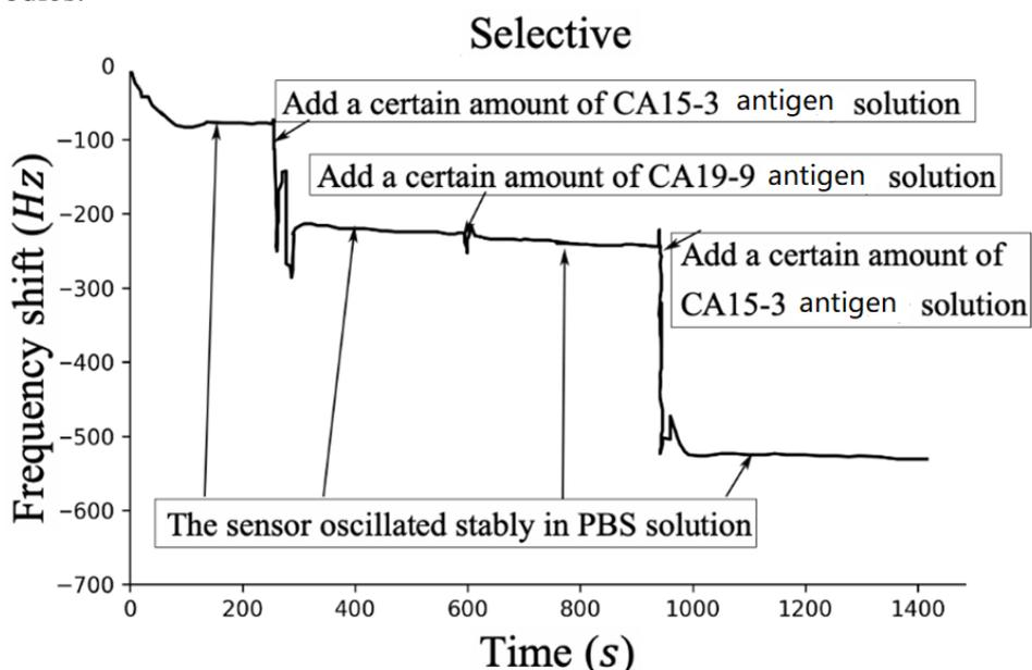
**Figure 12.** Selectivity characteristic of the QCM sensor
