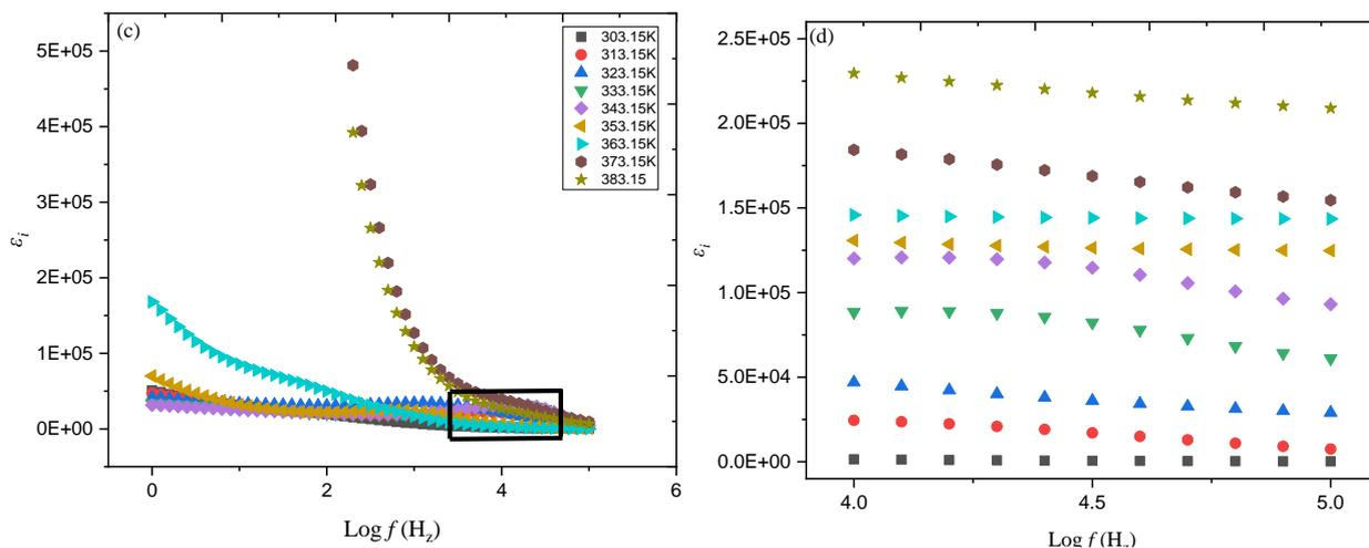
**Figure 3.** Temperature dependence of (a) dielectric constant ( $\epsilon_r$ ), (b) enlarged dielectric constant, (c) dielectric loss and (d) enlarged dielectric loss ( $\epsilon_i$ ) for PVA- $\text{K}_2\text{CO}_3$  (PK30) electrolytes at different temperatures
