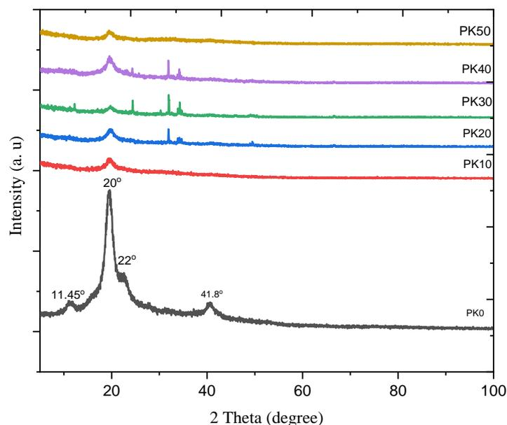
**Figure 1.** The XRD patterns of PVA-  $K_2CO_3$  composites.
