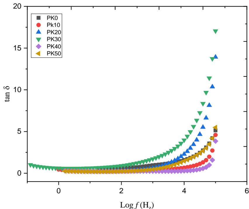
**Figure 6.** Variation of  $\tan \delta$  with frequency for PVA- $\text{K}_2\text{CO}_3$  at a different salt concentration at ambient temperature
