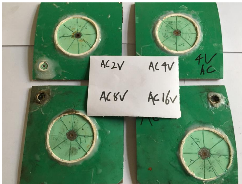
Figure 12. Physical diagram of AC interference disbonding test piece
