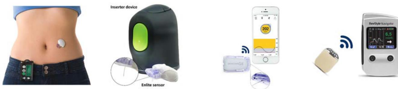
Figure 1. Examples of minimally invasive CGM systems based on electrochemical sensing techniques (reprinted with permission from MDPI [72]).
