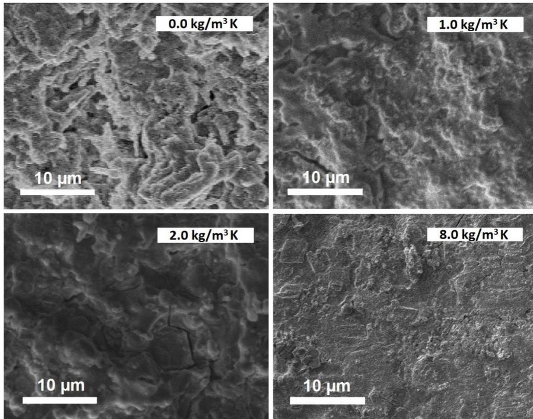
**Figure 4.** SEM images of steel rebars in different concrete samples after 8 weeks immersed to 3.5wt% NaCl environment
