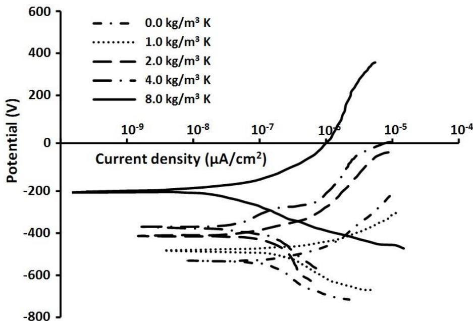
**Figure 2.** Polarization curves of DS steel reinforced concrete specimens with different concentrations of Kaolin immersed to 3.5 wt% NaCl environment for 8 weeks
