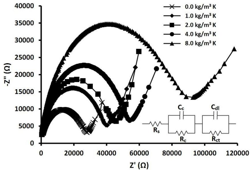
**Figure 3.** Nyquist diagrams for steel reinforced concrete specimens with different content of Kaolin admixtures after 8 weeks immersed to 3.5wt% NaCl solution. The inset shows an equivalent circuit model
