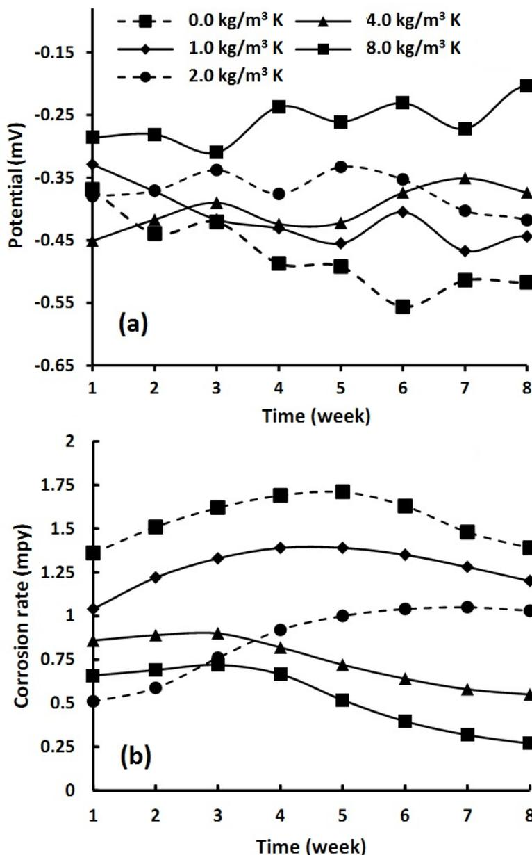
**Figure 1.** (a) Open-circuit potential and (b) Corrosion rate of reinforced concrete specimens with different Kaolin contents immersed in 3.5wt% NaCl environment
