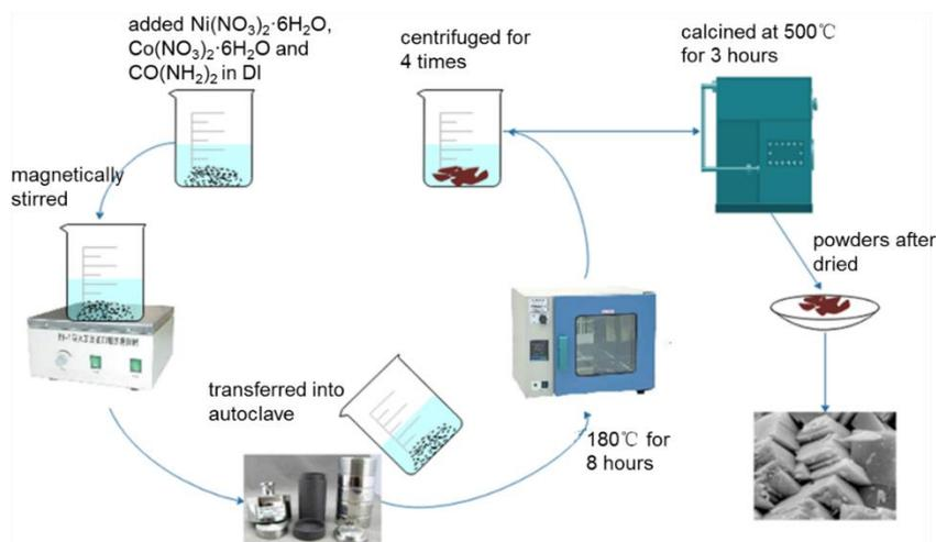
**Figure 1.** Synthesis of  $\text{NiO}/\text{Co}_3\text{O}_4$ .
