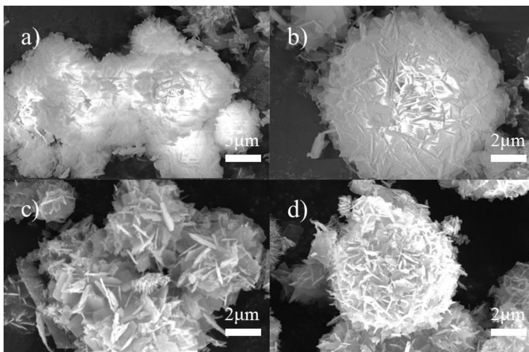
**Figure 2.** SEM images of NiO/Co<sub>3</sub>O<sub>4</sub> before and after calcination.
