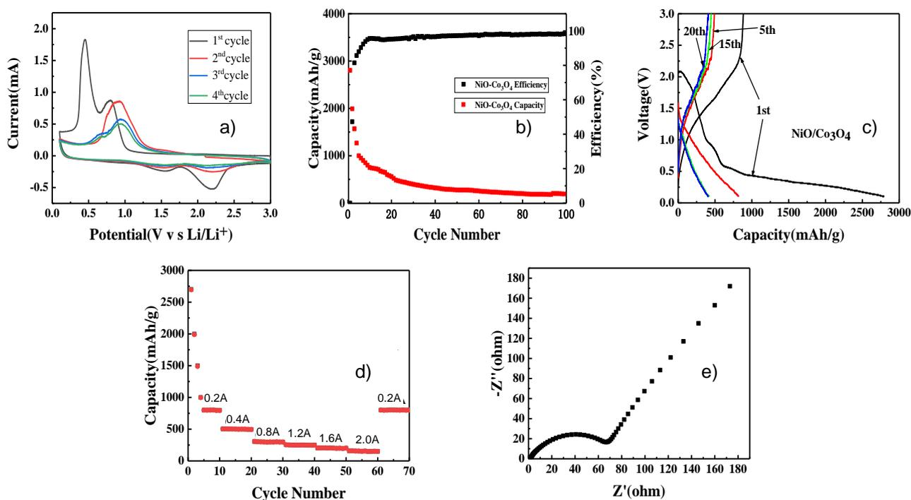
**Figure 4.** Electrochemical performance of  $\text{NiO}/\text{Co}_3\text{O}_4$ : (a) CV curves. (b) Cycling performance and coulombic efficiency. (c) Constant-current charge–discharge curves. (d) Rate capability at various current densities. (e) Impedance curves.
