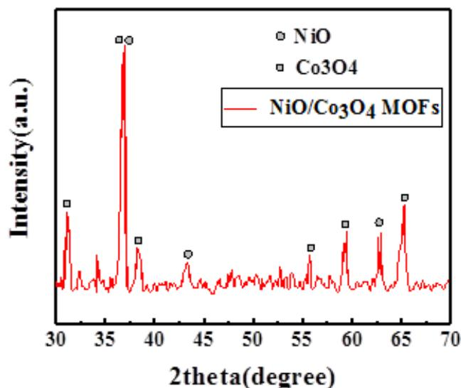
**Figure 3.** XRD pattern of NiO/Co<sub>3</sub>O<sub>4</sub>.
