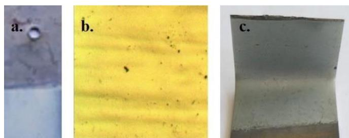
**Figure 5.** Macroscopic images (a and c) and optical microscope image (b) of the Zn film before (a and b) and after (c) a bending test
