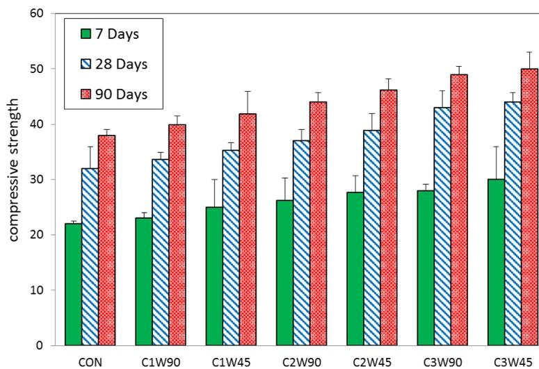
**Figure 2.** Compressive strength of concrete wrapped with CFP in different wrap fiber orientation at three different ages (7, 28 and 90 days) at room temperature
