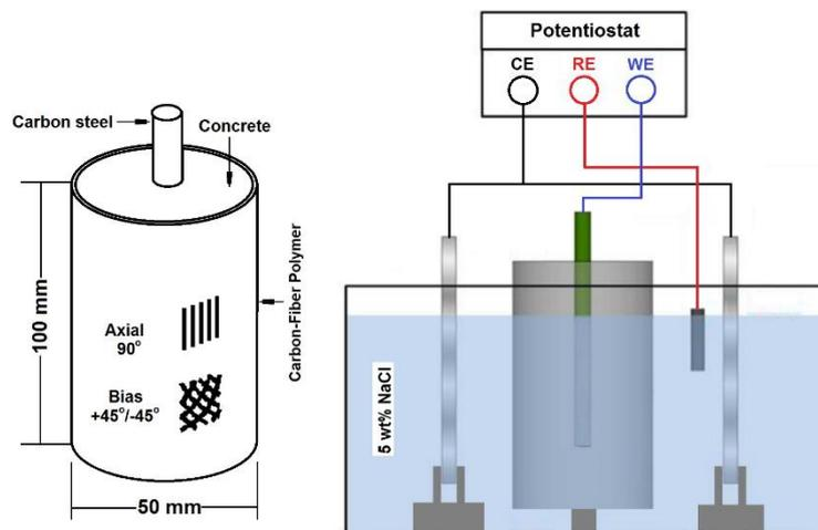
**Figure 1.** Schematic of EIS test configuration and wrap fiber orientation
