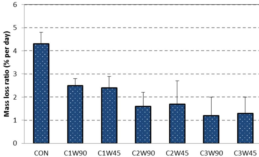
**Figure 4.** Mass loss ratio (% per day) in various samples with CFP in different wrap fiber orientation and different number of CFP layers at room temperature
