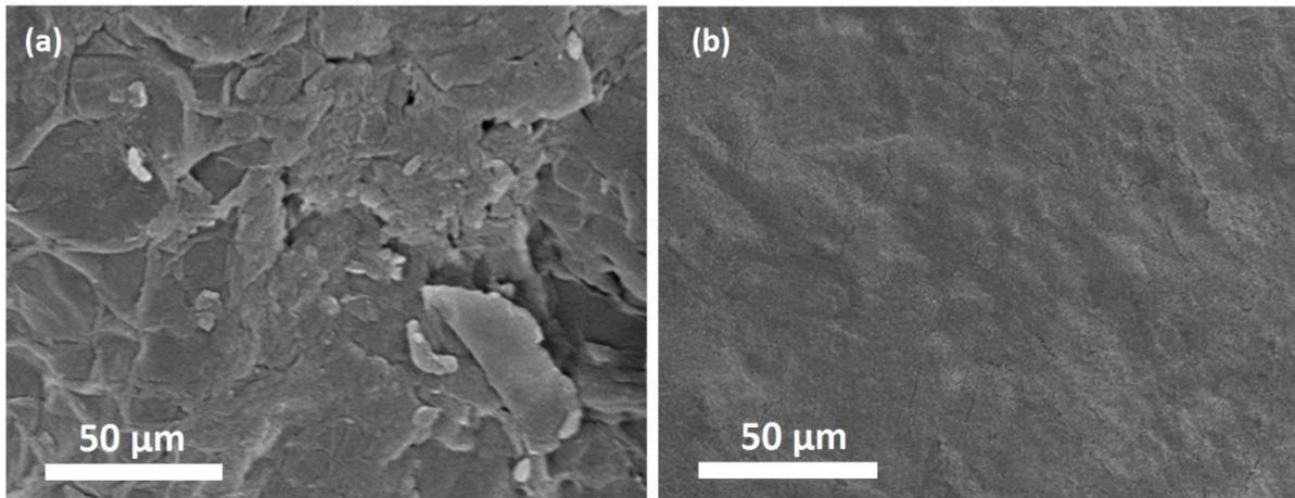
**Figure 9.** SEM surface morphology of carbon steel rebar in CON and C3W45 samples after exposed to 5 wt% NaCl solution for 4 weeks at room temperature
