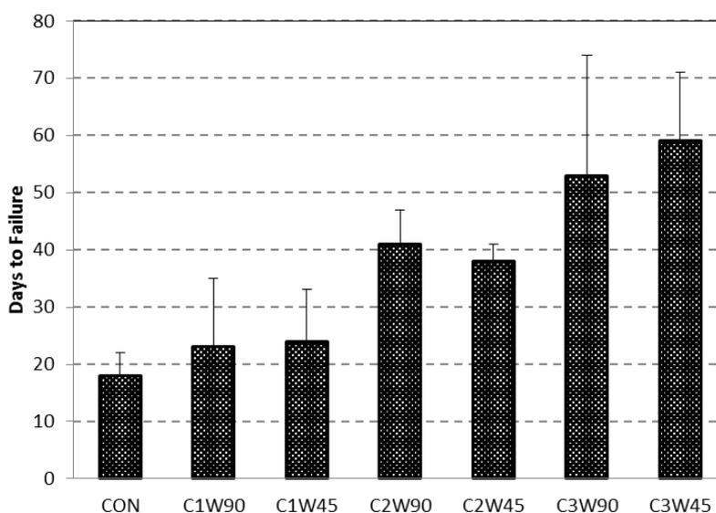
**Figure 3.** Average day to failure in various samples with CFP in different wrap fiber orientation and different number of CFP layers at room temperature
