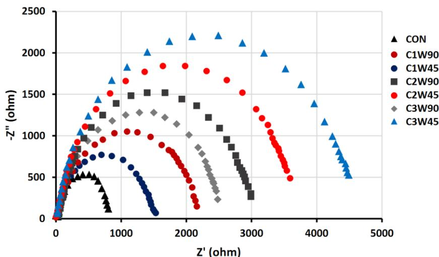
**Figure 6.** Nyquist plots of carbon steel rebars in concrete with CFP wrapped in different fiber orientation and different number of CFP layers at room temperature in 5% NaCl solution.
