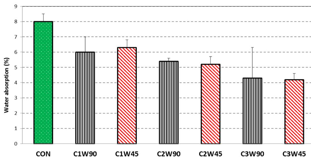
**Figure 8.** Water absorption of specimens after four weeks immersing time in 5 wt% NaCl solution at room temperature
