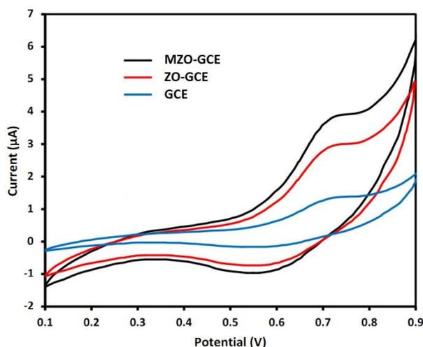
**Figure 3.** Cyclic voltammograms recorded by GCE, ZO-GCE and MZO-GCE electrodes in 0.1M PB solution, including 0.5 mM sunset yellow at  $50 \text{ mVs}^{-1}$  scan rate
