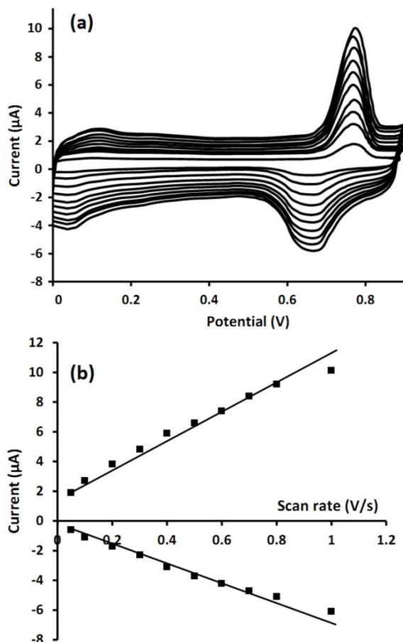
**Figure 4.** CVs of  $10 \mu\text{M}$  sunset yellow in 0.1M PB solution at pH 8.0 in various scan rates
