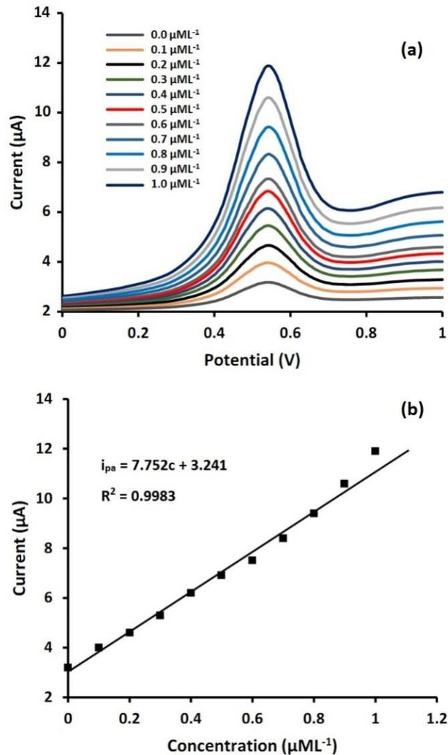
**Figure 5.** (a) DPV response of MZO-GCE electrode to successive injection of 0.1 μM sunset yellow in 0.1 M PB solution at pH 8.0 and scan rate of 50 mV s<sup>-1</sup> (b) Diagram of peak currents vs. sunset yellow concentration.
