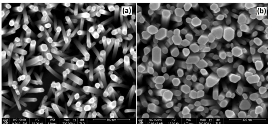
**Figure 1.** The surface morphology of (a) ZO-GCE and (b) MZO-GCE samples.
