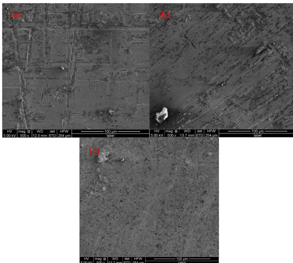
**Figure 9.** Morphology of eroded surface of carbon steels at different rotational speeds in sand-containing solution. (a) 250 rpm, (b) 500 rpm, (c) 750 rpm.
