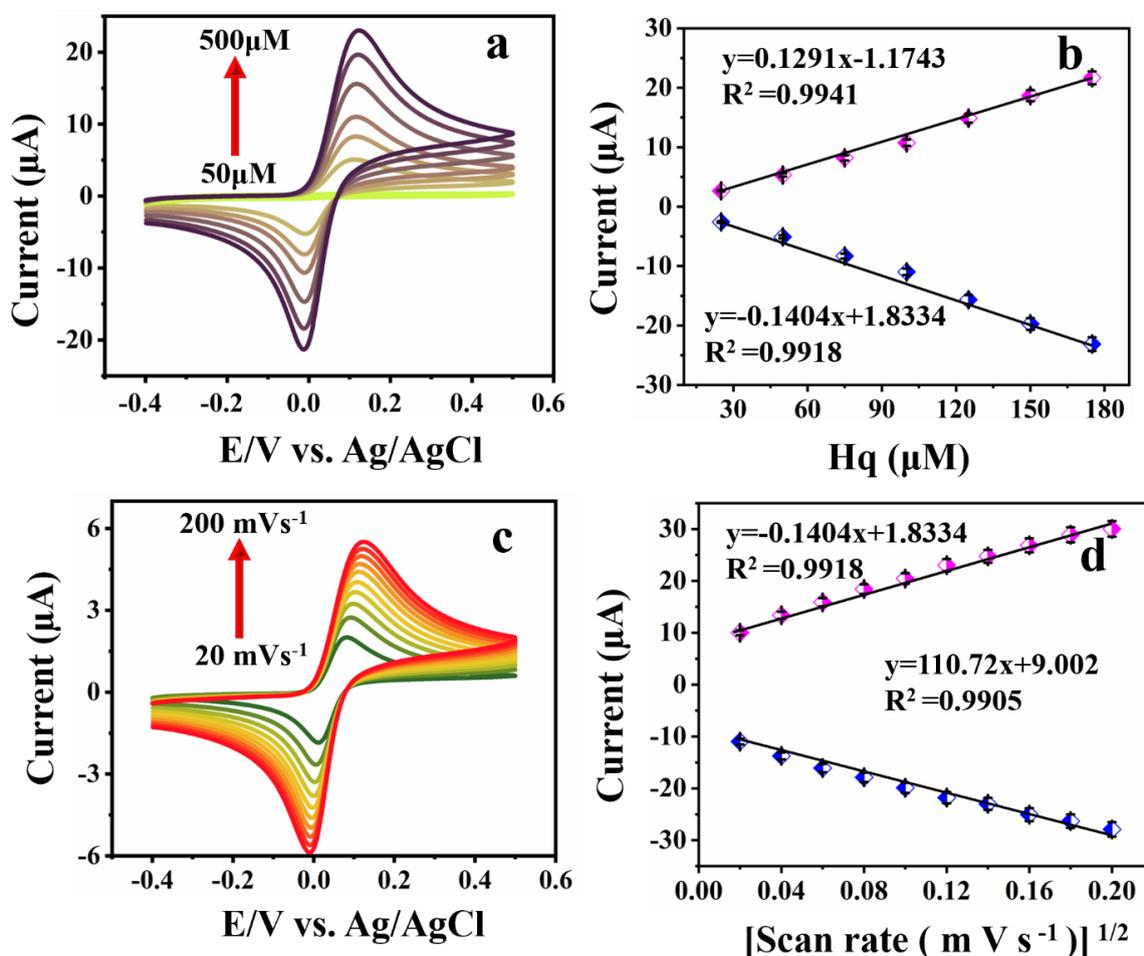
**Figure 4.** showing the cyclic voltammograms of  $\text{Zr}(\text{MoO}_4)_2/\text{rGO}$  (a) different concentration ranging from 50-500  $\mu\text{M}$  in the presence of 0.1 M of PB solution at  $50 \text{ mVs}^{-1}$  (b) respective linearity plot of (a). (c) shows the scan rate performed for  $\text{Zr}(\text{MoO}_4)_2/\text{rGO}$  ranging from 20 – 200  $\text{mVs}^{-1}$  and (d) linearity plot.
