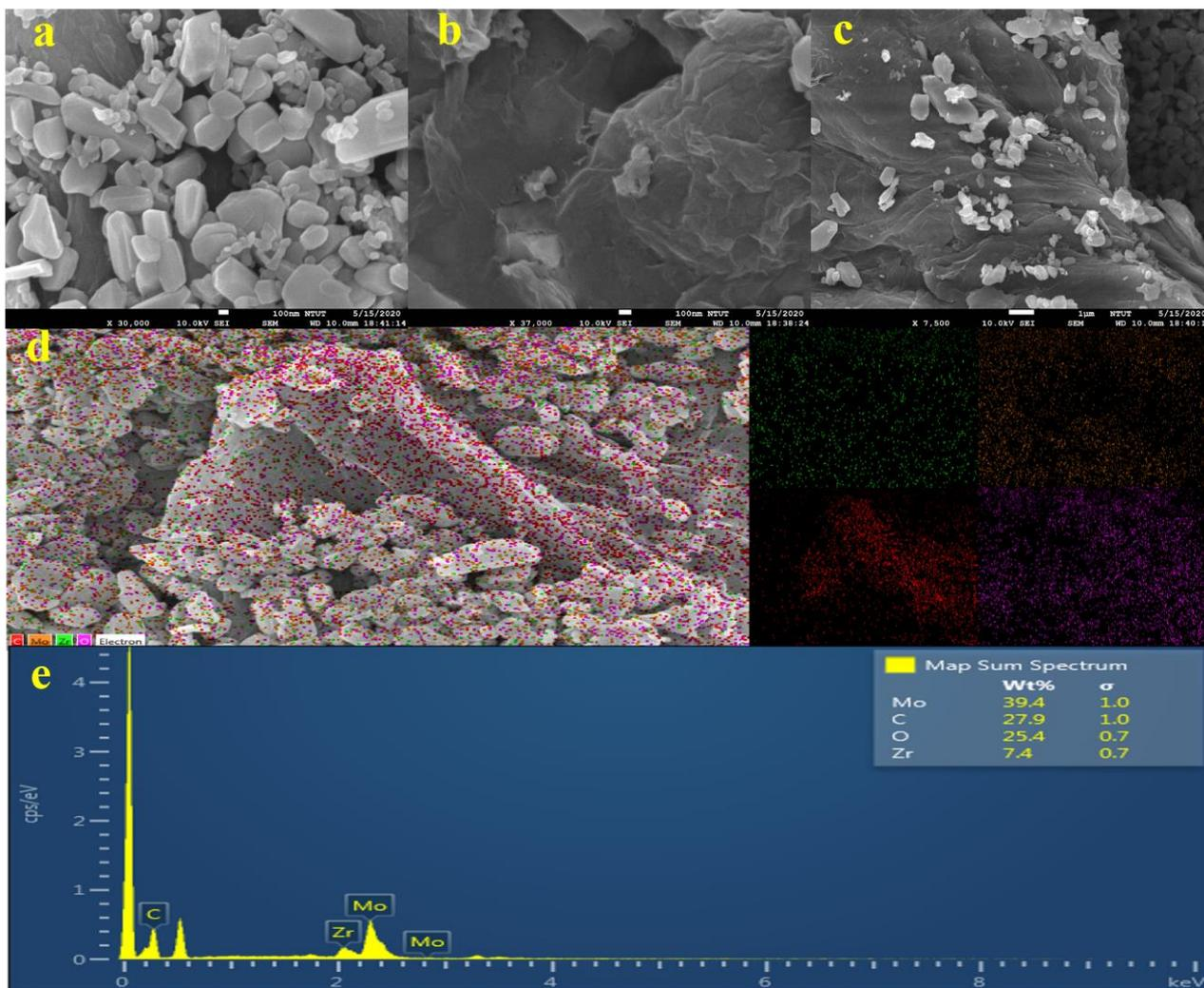
**Figure 2.** FESEM photographs of (a) ZrMo<sub>4</sub> (b) rGO (c) ZrMo<sub>4</sub>/rGO (d) elemental mapping and (e) EDAX spectrum.
