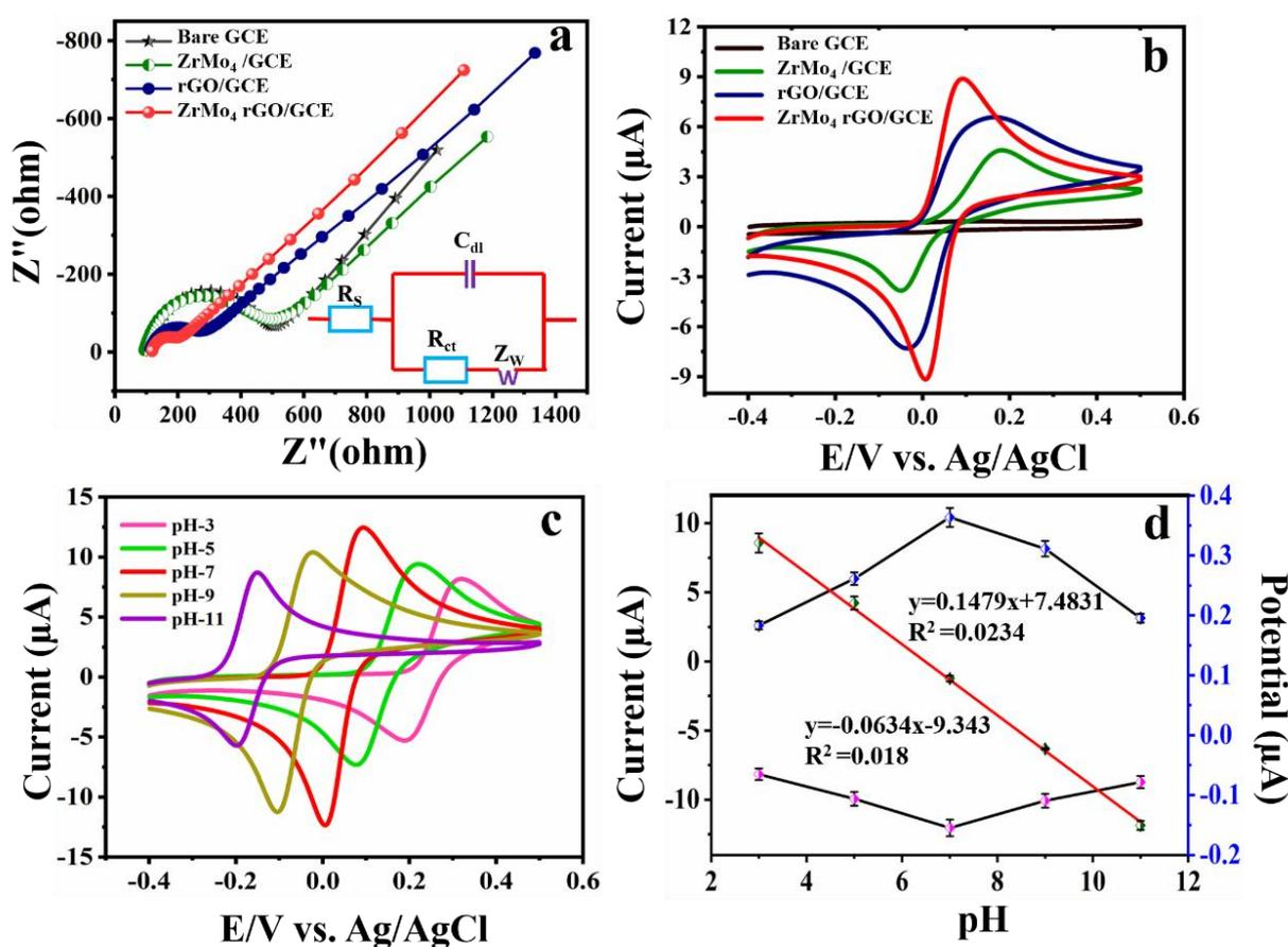
**Figure 3.** (a) EIS plots of GCE modified  $Zr(MoO_4)_2$ , rGO and  $Zr(MoO_4)_2/ rGO$  (b) different film comparison (c) varying pH studies (d) linearity plot of Ph.
