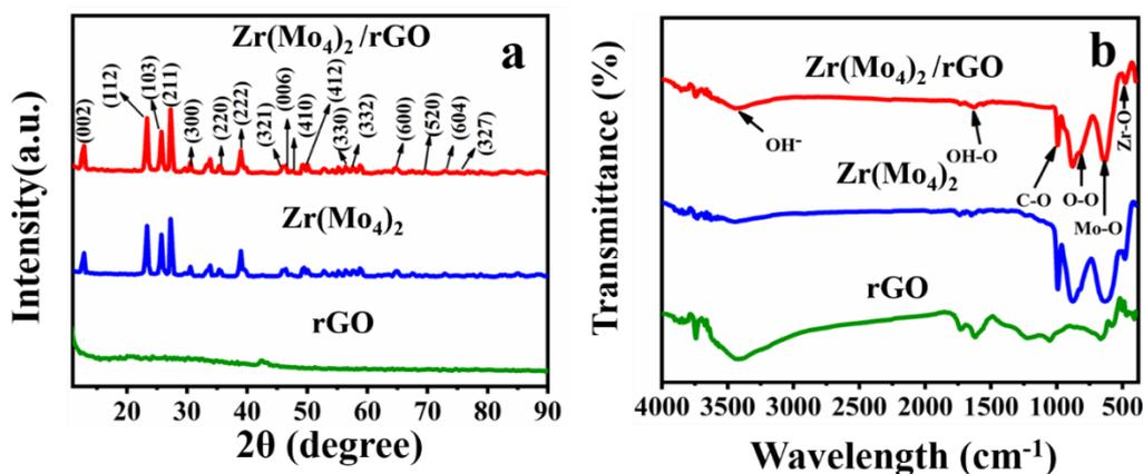
**Figure 1.** (a) XRD pattern of rGO,  $Zr(MoO_4)_2$ , and  $Zr(MoO_4)_2/rGO$  and (b) FTIR spectra of rGO,  $Zr(MoO_4)_2$ , and  $Zr(MoO_4)_2/rGO$ .
