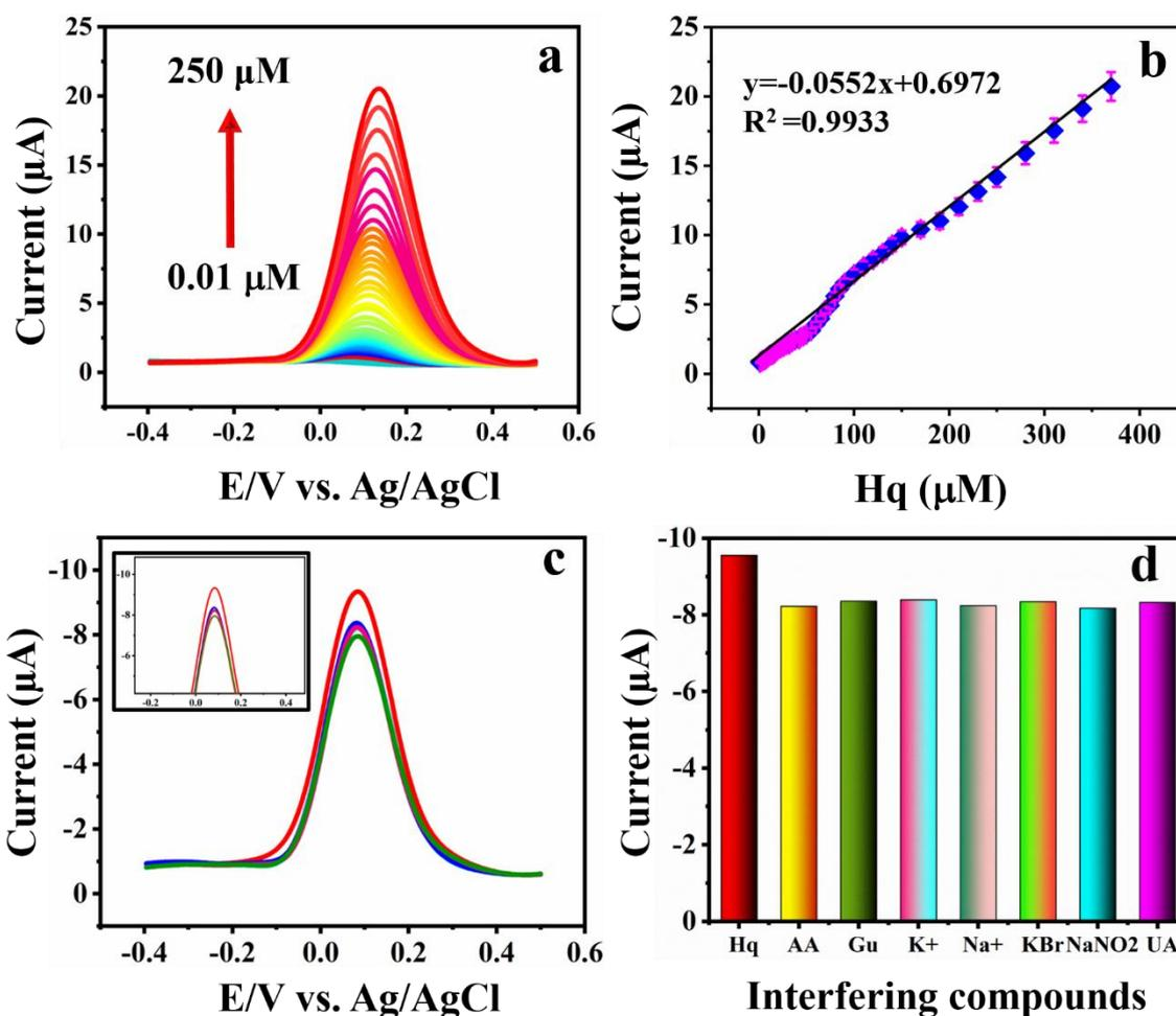
**Figure 6.** (a) DPV studies of  $Zr(MoO_4)_2/rGO$  at different concentration of HQ varying from  $0.01 \mu M$  to  $250 \mu M$  (b) linearity plot (c) interference studies plot with closer view inset shown at the top and (d) bar diagram.
