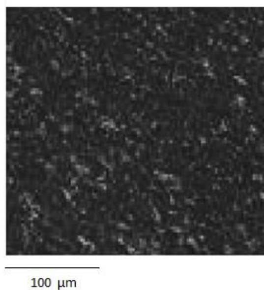
Figure 4. SEM micrograph of the titanium surface after one entire potential scan in 0.5 M NaF solution at 50 mV/s.
