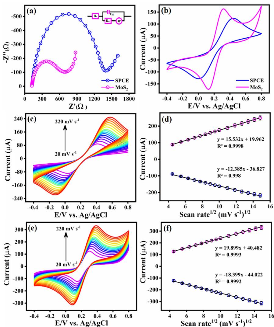
**Figure 3.** (a) EIS plot, (b) CV curve of bare SPCE and MoS<sub>2</sub>/SPCE, (c, e) The CV curve of different scan rate at 20–200 mV/s, and (d, f) corresponding calibration plot of the redox peak current and the square root of scan rate. All experiment was conducted in 5.0 mM [Fe(CN)<sub>6</sub>]<sup>3-/4-</sup>/0.1 M KCl.
