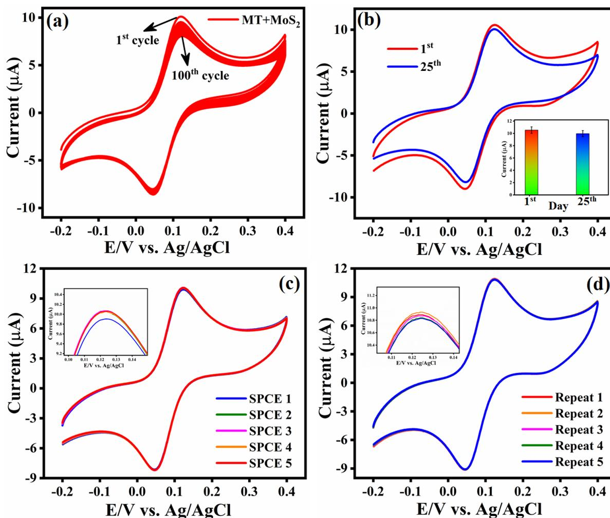
**Figure 7.** (a) CV curve of cyclic stability of 100 cycles in the  $\text{MoS}_2/\text{SPCE}$ , (b) storage stability (the result of bar diagram), (c) reproducibility of five independent electrodes, and (d) repeatability. All measurements were carried out by CV with  $\text{N}_2$ -saturated containing 0.05 M PBS (pH 7) containing 100  $\mu\text{M}$  MT at 50  $\text{mV s}^{-1}$  scan rate.
