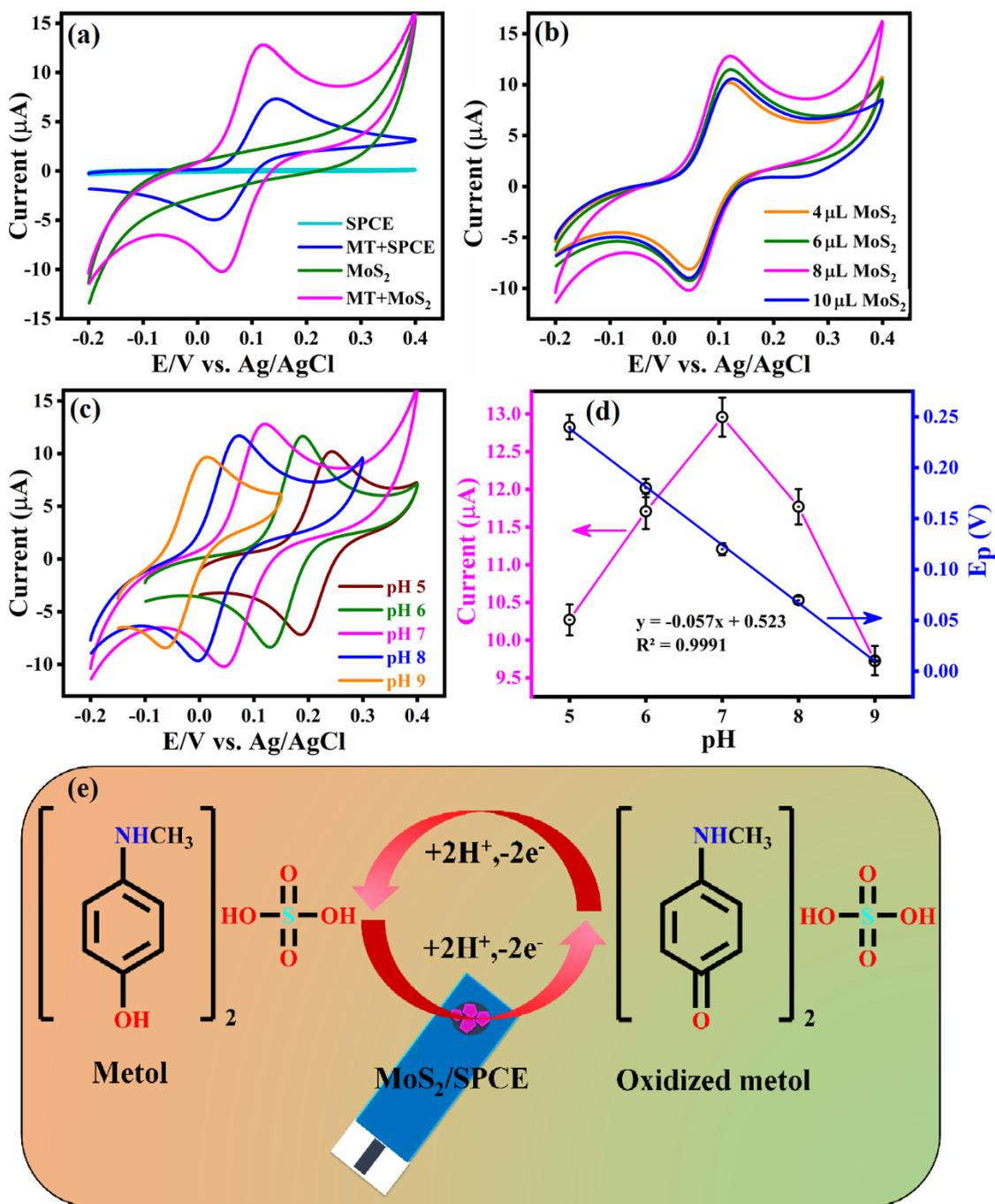
**Figure 4.** (a) CV curve of bare SPCE and MoS<sub>2</sub>/SPCE in the absence and presence of MT, (b) various loading catalysis is 4, 6, 8, and 10 μL (mg/mL), (c) CV response of different pH from 5 to 9 (0.05 PBS). (d) the linear plot between oxidation peak current and peak potential versus different pH. All the experiment were performed, N<sub>2</sub>-saturated 0.05 M PBS (pH 7) in 00 μM MT, and (e) the possible electrochemical redox mechanism of MT.
