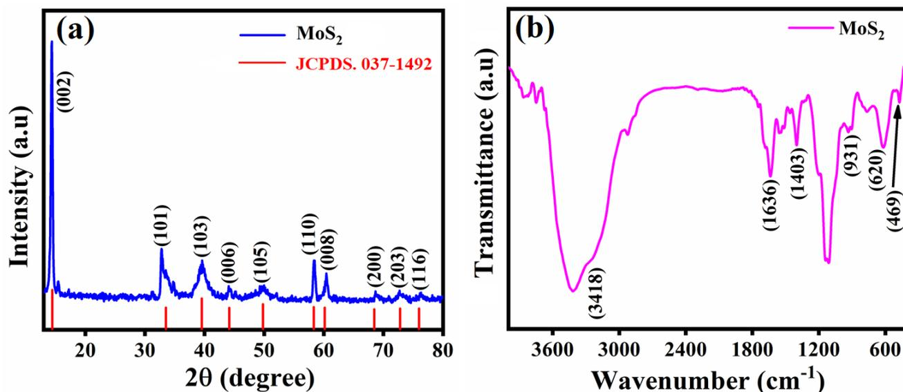
**Figure 1.** (a) XRD pattern, and (b) FT-IR spectra of the flake-like MoS<sub>2</sub>.
