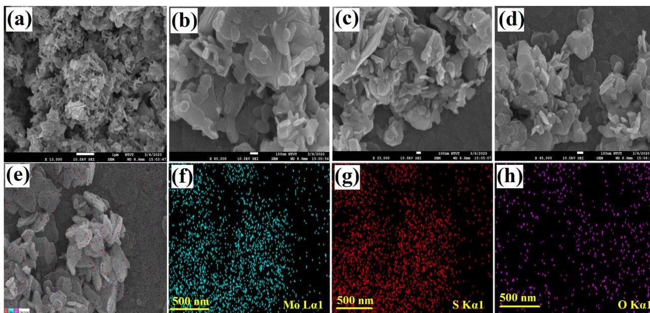
**Figure 2.** (a–d) Different magnification FE-SEM images of MoS<sub>2</sub> flake-like structure, (e) FE-SEM-elemental mapping analysis (f) Mo, (g) S, and (h) O element of MoS<sub>2</sub>.
