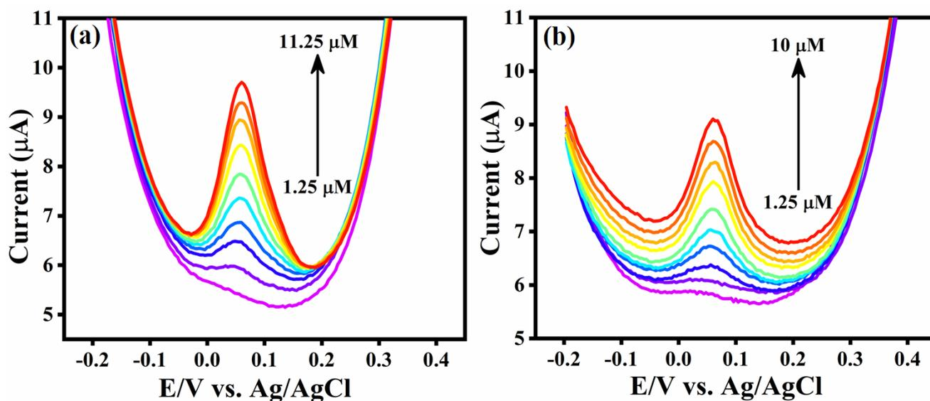
**Figure 8.** DPV response of real sample (a) river water and (b) tap water in 0.05 M PBS (pH 7) with various amount of MT.
