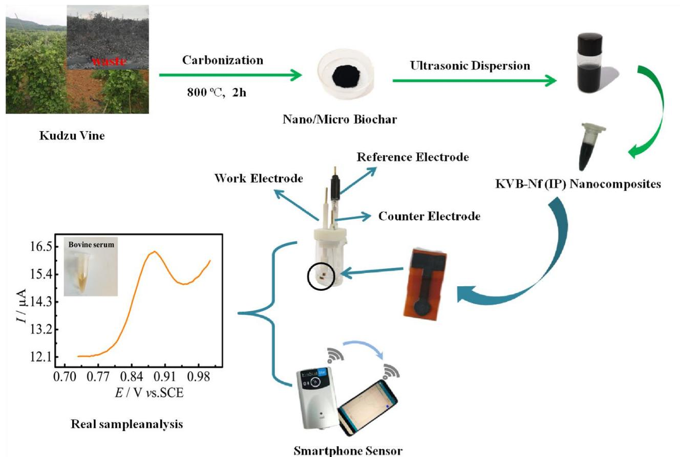
**Scheme 1.** Wireless bluetooth sensing platform based on KVB/FCE for portable intelligent analysis of CLB in bovine serum sample using cheap miniaturized analyzer composed of both smartphone and electrochemical mini-workstation.
