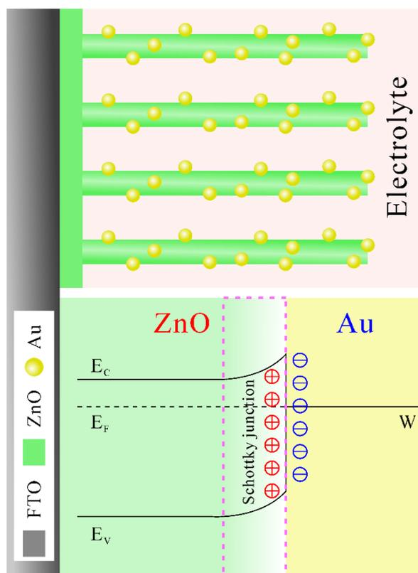
**Figure 4.** The schematic diagram of Schottky junction in ZnO/Au interface, which help trapping electron during charging and electron transport during discharging.
