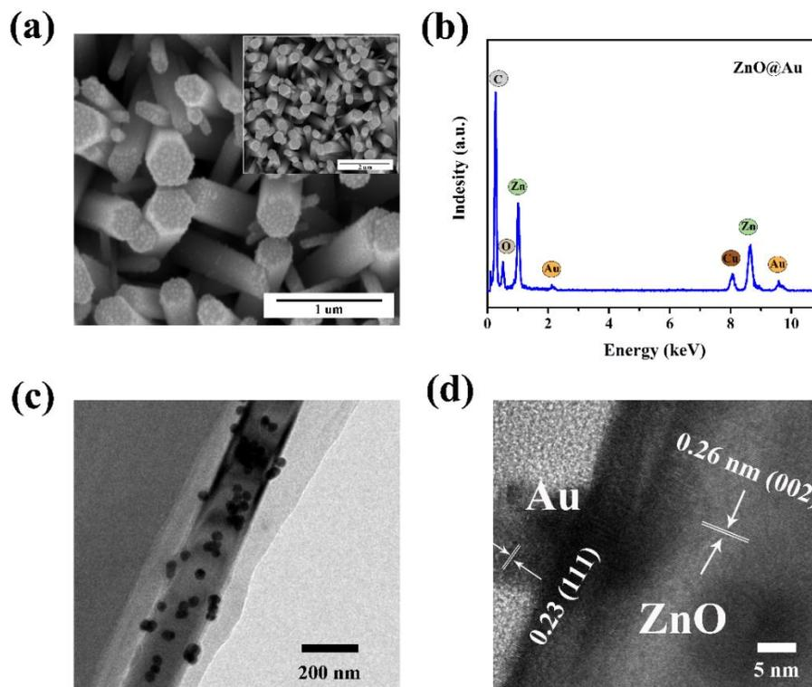
**Figure 2.** (a) SEM images of the hybrid ZnO@Au nanorod array electrodes. (b) EDX analysis of the the hybrid ZnO@Au nanorod array electrodes. (c) TEM images of the hybrid ZnO@Au nanorod array electrodes. (d) HRTEM images of the hybrid ZnO@Au nanorod array electrodes.
