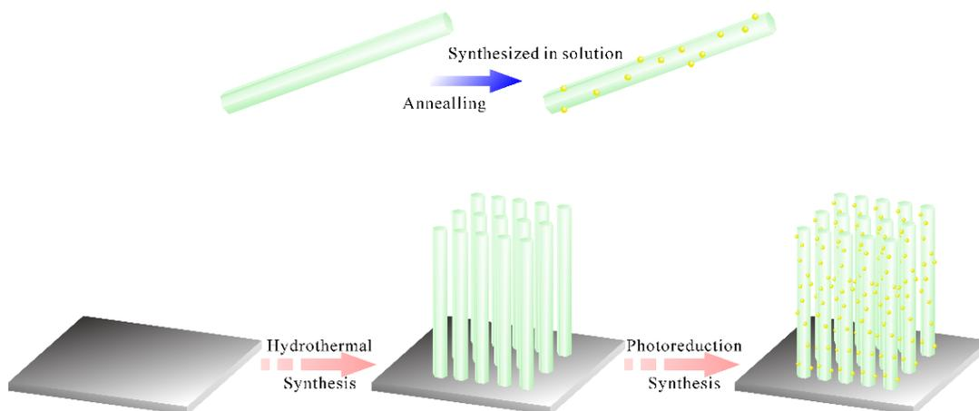
**Figure 1.** Schematic illustration of the construction of hybrid ZnO@Au nanorod array electrode
