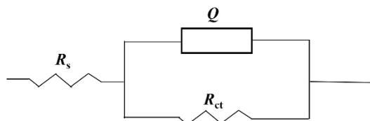
**Figure 6.** EEC for fitting the EIS experimental data.
