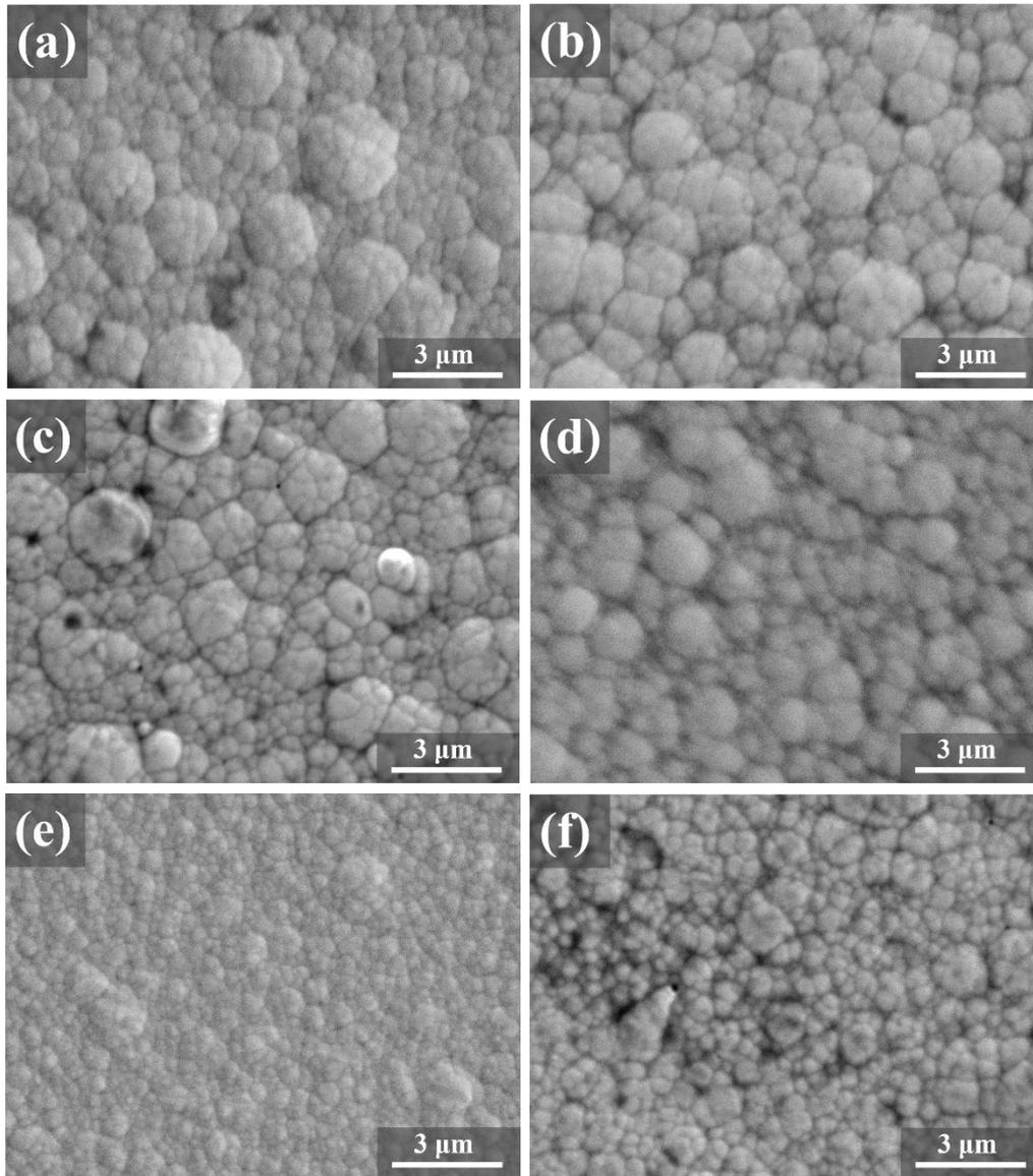
**Figure 3.** Surface morphologies of the obtained Ni-Mo coating (a) and Ni-Mo/TiO<sub>2</sub> coatings (b: Ni-Mo/TiO<sub>2</sub> I, c: Ni-Mo/TiO<sub>2</sub> II, d: Ni-Mo/TiO<sub>2</sub> III, e: Ni-Mo/TiO<sub>2</sub> IV, and f: Ni-Mo/TiO<sub>2</sub> V).
