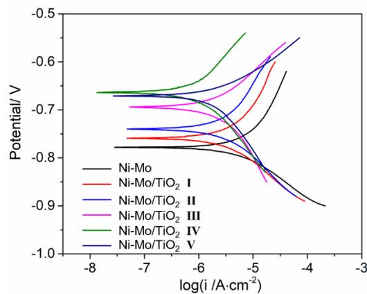
**Figure 4.** Polarization curves of the obtained Ni-Mo coating and Ni-Mo/TiO<sub>2</sub> coatings in the 3.5 wt.% NaCl solution.
