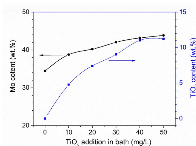
**Figure 1.** Comparisons of the coatings deposited from baths containing different amounts of TiO<sub>2</sub> nanoparticles.
