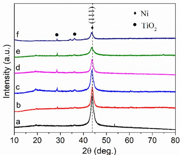
**Figure 2.** XRD patterns of the obtained Ni-Mo coating (a) and Ni-Mo/TiO<sub>2</sub> coatings (b: Ni-Mo/TiO<sub>2</sub> I, c: Ni-Mo/TiO<sub>2</sub> II, d: Ni-Mo/TiO<sub>2</sub> III, e: Ni-Mo/TiO<sub>2</sub> IV, and f: Ni-Mo/TiO<sub>2</sub> V)
