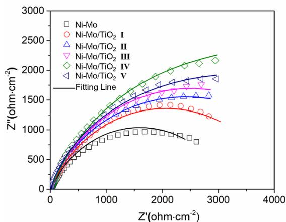
**Figure 5.** Nyquist plots of the obtained Ni-Mo coating and Ni-Mo-TiO<sub>2</sub> coatings in the 3.5 wt.% NaCl solution.
