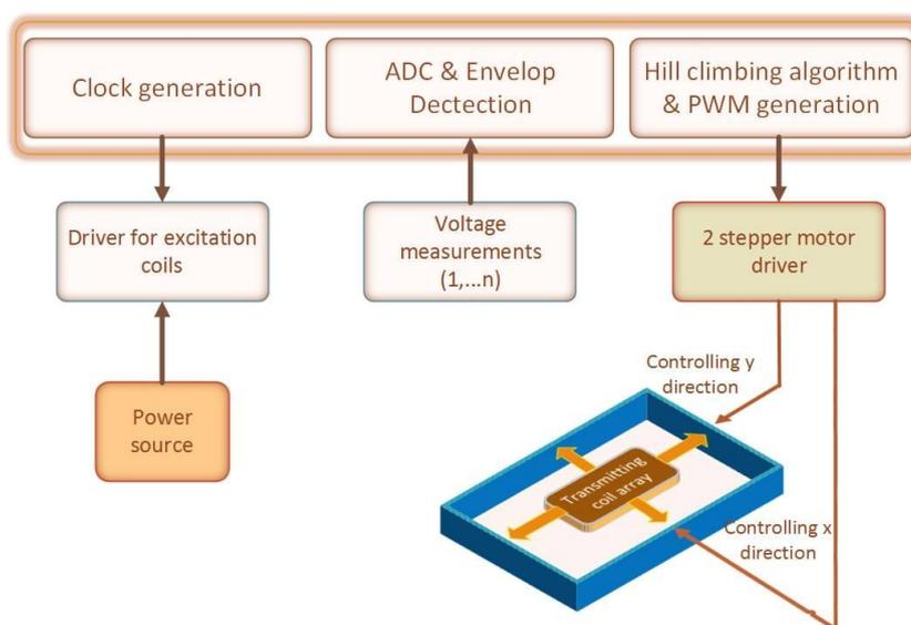
**Figure 3.** The proposed wireless battery charging system of the quadcopter
