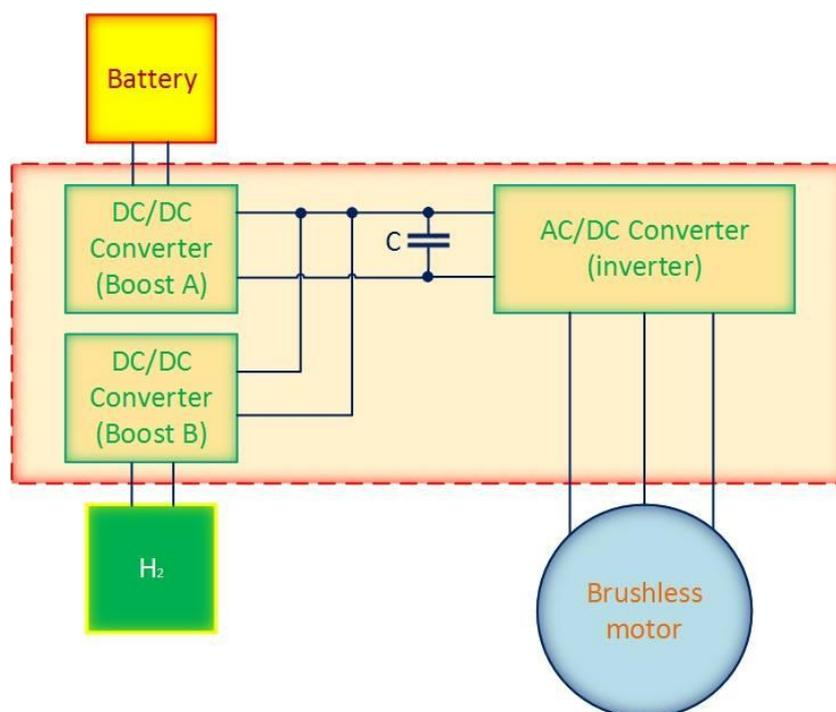
**Figure 4.** UAV hybrid power system of Fuel cell and Battery
