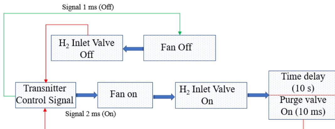
**Figure 5.** Flow diagram design of the fuel cell controller
