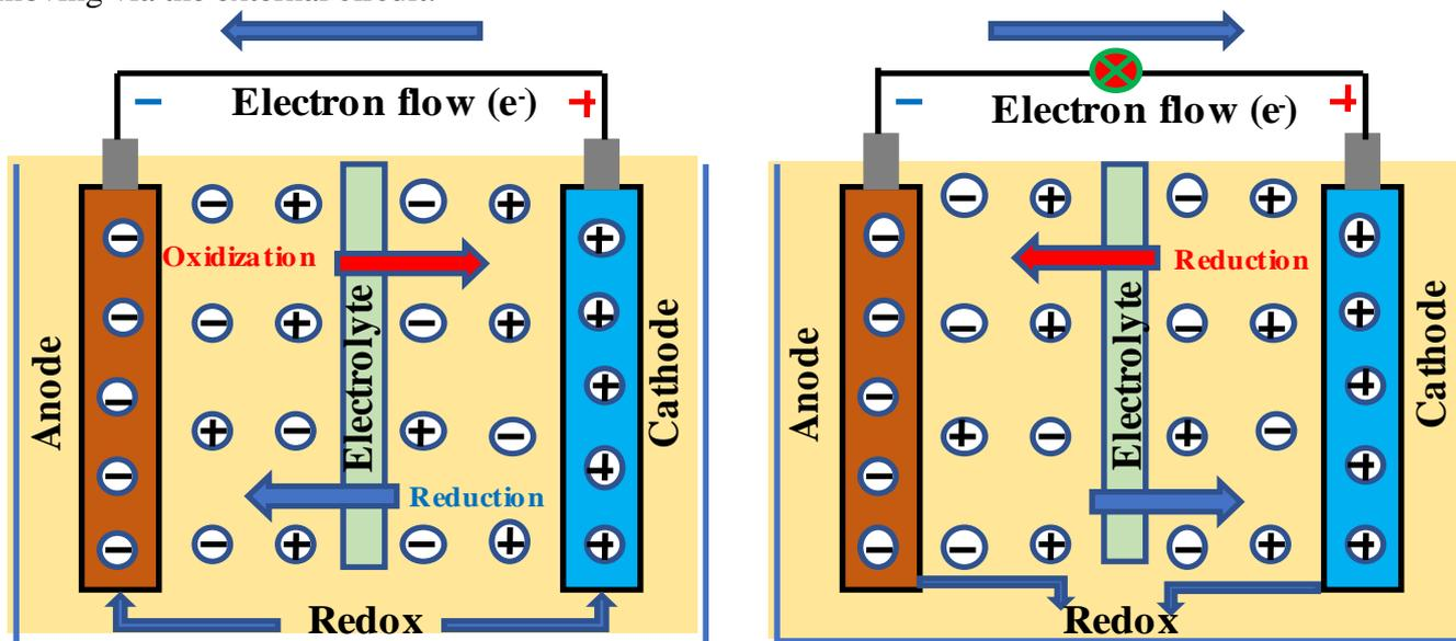
**Figure 1.** Battery cell operation under (a) charging mode and (b) discharging mode
