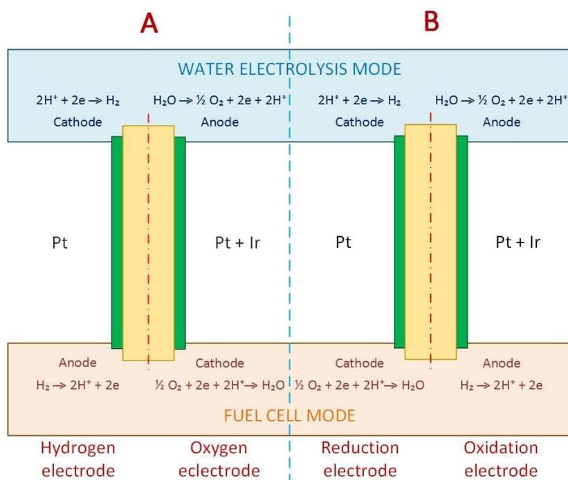
**Figure 9.** Schematic procedure of the working principles of the URFC system
