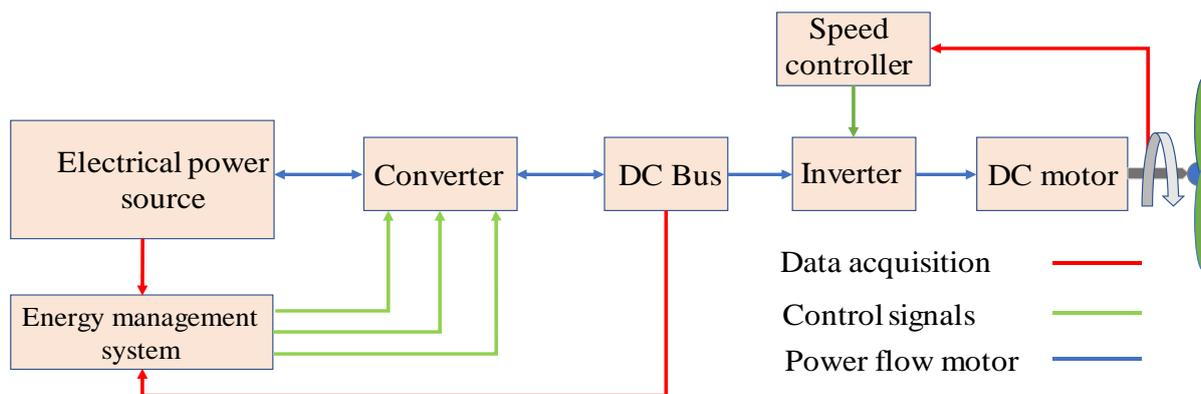
**Figure 2.** A typical propulsion system diagram of UAVs
