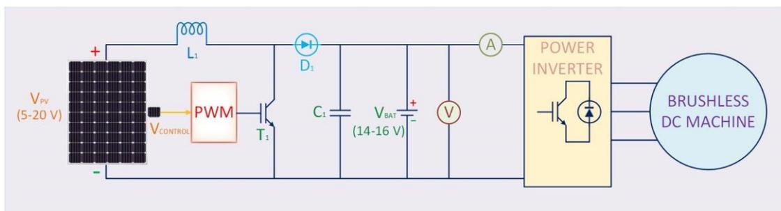
**Figure 7.** Power system design of the solar system for UAV
