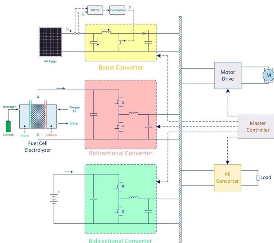
**Figure 8.** Hybrid power system of battery, fuel cell and solar energy for UAVs
