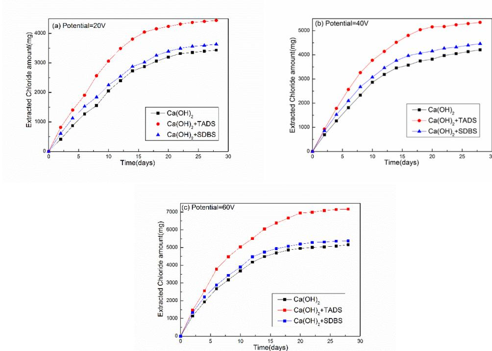
**Figure 2.** Changes of total chloride amounts in the anode and cathode electrolytic solutions with time, the applied potentials were (a) 20 V, (b) 40V and (c) 60 V, respectively.
