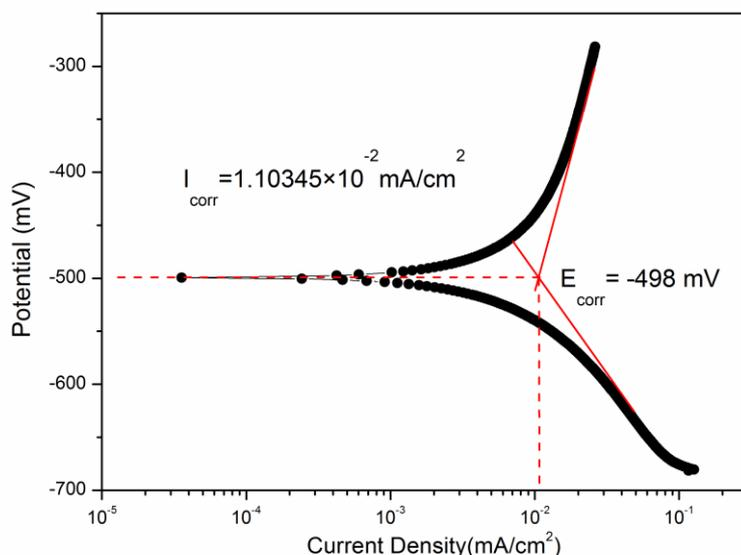
**Figure 7.** Potentiodynamic polarization curve for embedded steel in the mortar sample before the ECE treatment.
