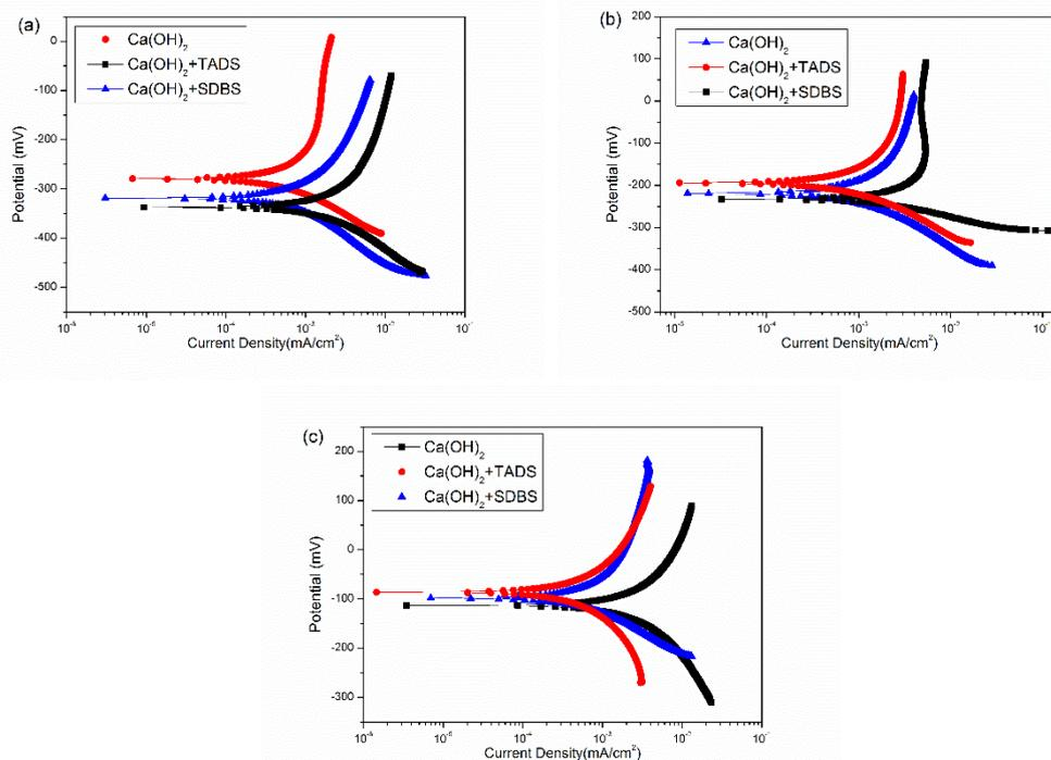
**Figure 8.** Potentiodynamic polarization curves for embedded steels in the mortar samples after the ECE treatments with various electrolyte solutions at the different potentials of (a) 20 V, (b) 40 V, and (c) 60 V.
