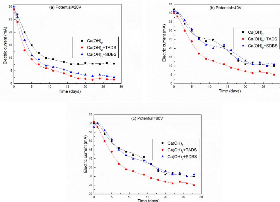
**Figure 5.** Variations of the electric current with the treatment time, the applied potentials were (a) 20 V, (b) 40V and (c) 60 V, respectively.
