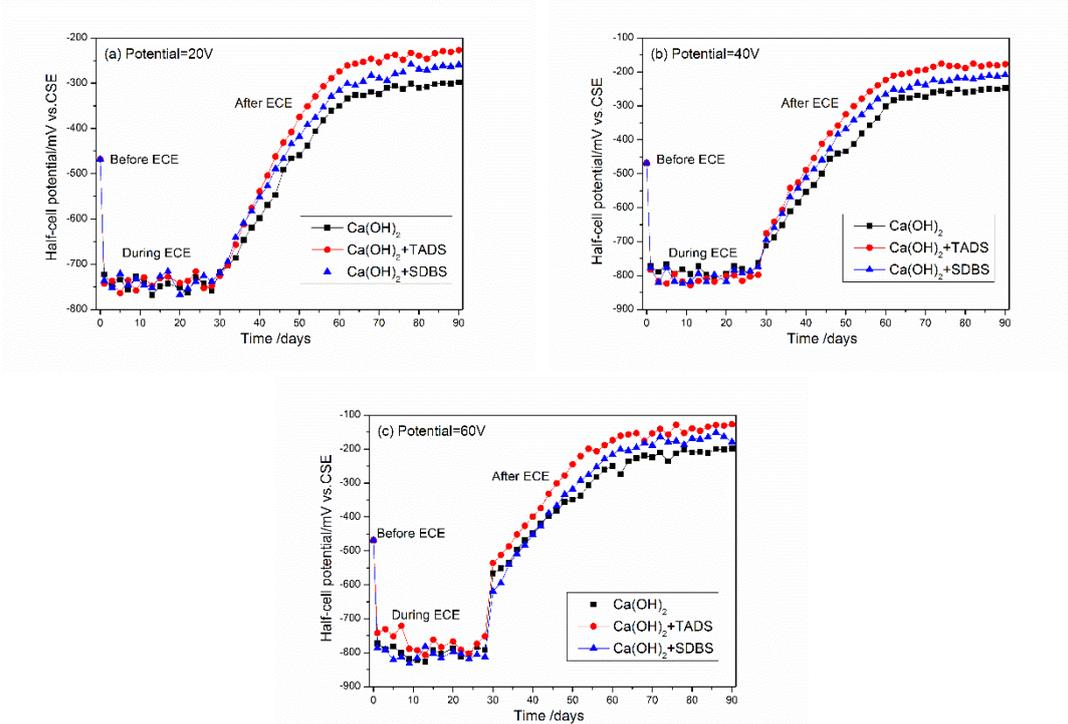
**Figure 6.** HCPs of the steels in the mortar samples at the applied potentials of (a) 20 V, (b) 40 V and (c) 60 V.
