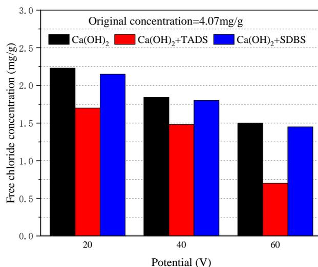
**Figure 3.** Changes of free chloride concentrations in the mortar sample near the steel bar with the applied potential after ECE treatment.
