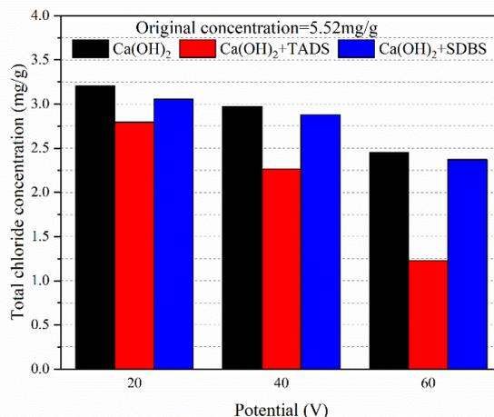
**Figure 4.** Changes of total chloride concentrations in the mortar sample near the steel bar with the applied potential after ECE treatment.
