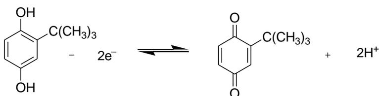
**Scheme 1.** The oxidation reaction equation of TBHQ at the modified electrode
