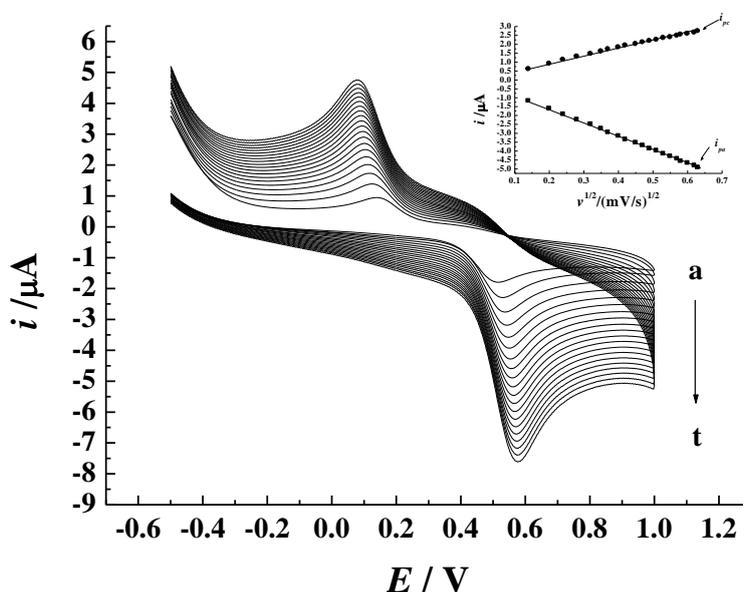
**Figure 5.** CVs of  $1.00 \times 10^{-4}$  mol/L TBHQ in PBS (pH 2.2) of different scan rate at ADC/GCE. Oxidation and reduction peak currents and the square root of scan rate show the linearity (Insert). Scan rate from a to t corresponds to 20, 40, 60, 80, 100, 120, 140, 160, 180, 200, 220, 240, 260, 280, 300, 320, 340, 360, 380, 400 mV/s.
