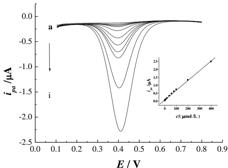
**Figure 7.** DPVs of different concentrations of TBHQ at ADC/GCE in PBS (pH 2.2). Letters from a to i correspond to concentration of 0.4, 6.0, 10, 20, 40, 60, 80, 100  $\mu\text{mol/L}$ . Insert is the plot of the oxidation peak current versus concentration of TBHQ.
