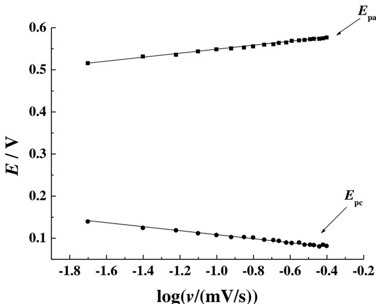
**Figure 6.** Linearity of the peak potentials of  $1.00 \times 10^{-4}$  mol/L TBHQ versus the logarithms of the scan rates
