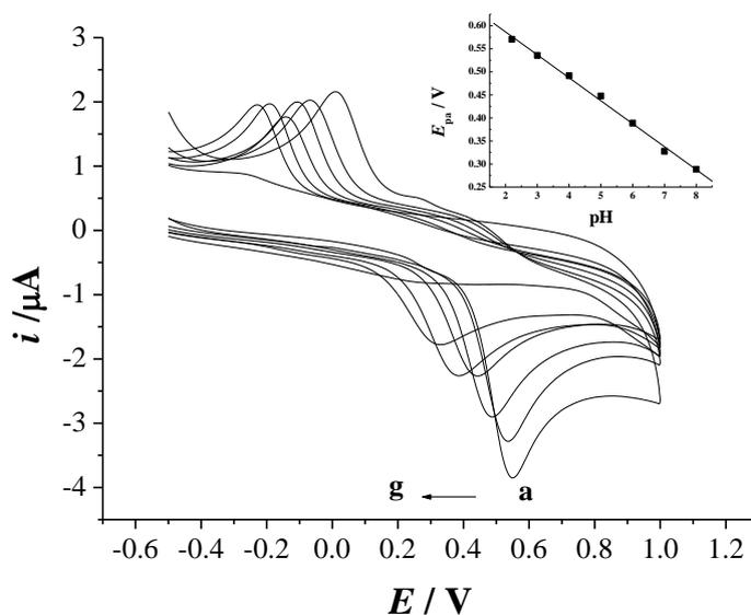
**Figure 4.** CVs of  $1.0 \times 10^{-4}$  mol/L TBHQ in PBS of different pH values (a to g: 2.2, 3.0, 4.0, 5.0, 6.0, 7.0 and 8.0) on the ADC/GCE. Insert is the plot of peak potential of TBHQ vs. pH value of PBS. Scan rate is 100 mV/s.
