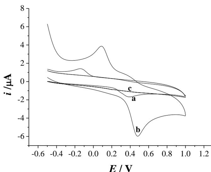
**Figure 3.** CVs of  $1.00 \times 10^{-4} \text{ mol/L}$  TBHQ at bare GCE (a), ADC/GCE (b) and ADC/GCE in PBS (pH=2.2) (c), scan rate is  $100 \text{ mV/s}$
