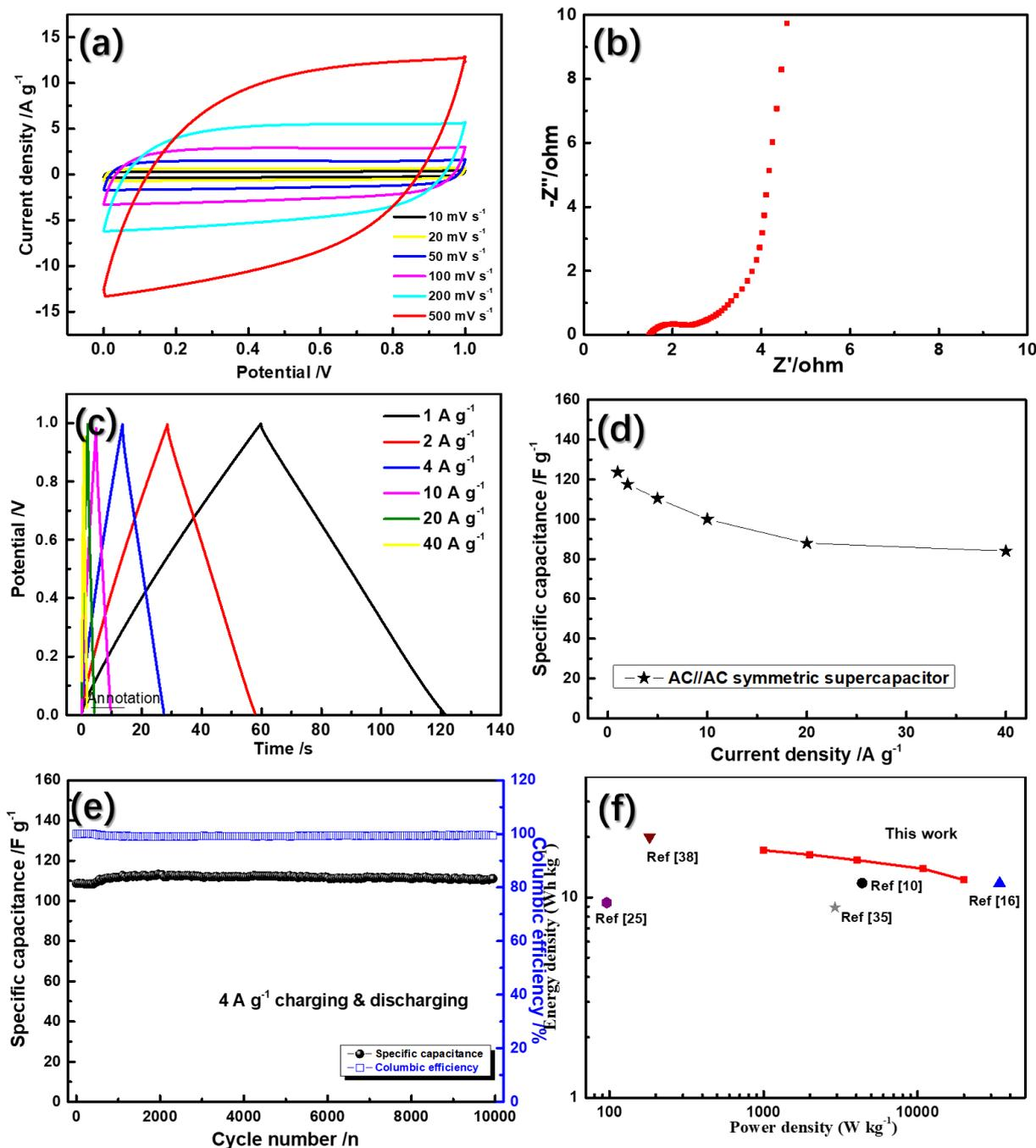
**Figure 8.** (a) CV curves at various scanning rates, (b) EIS spectra at discharge state, (c) GCD profiles at different current densities, (d) Relationship between current densities and specific capacitance, (e) Cycling stability and columbic efficiency, and (f) power density & energy density of the symmetric supercapacitors.
