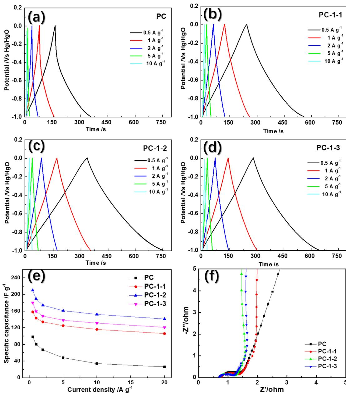
**Figure 7.** GCD profiles of (a) PC sample, (b) PC-1-1 sample, (c) PC-1-2 sample and (d) PC-1-3 sample at various current densities; (e) Relationship between current density and specific capacitance; (f) EIS spectra of PC samples at discharge state.
