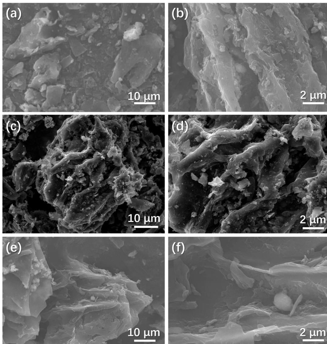
**Figure 2.** SEM morphologies of PC samples (a-b) PC-1-1, (c-d) PC-1-2 and (e-f) PC-1-3.
