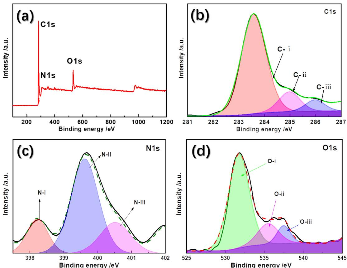
Figure 5. X-ray spectra of PC-1-2 sample (a) full spectrum, (b) C1s, (c) N1s, and (d) O1s.
