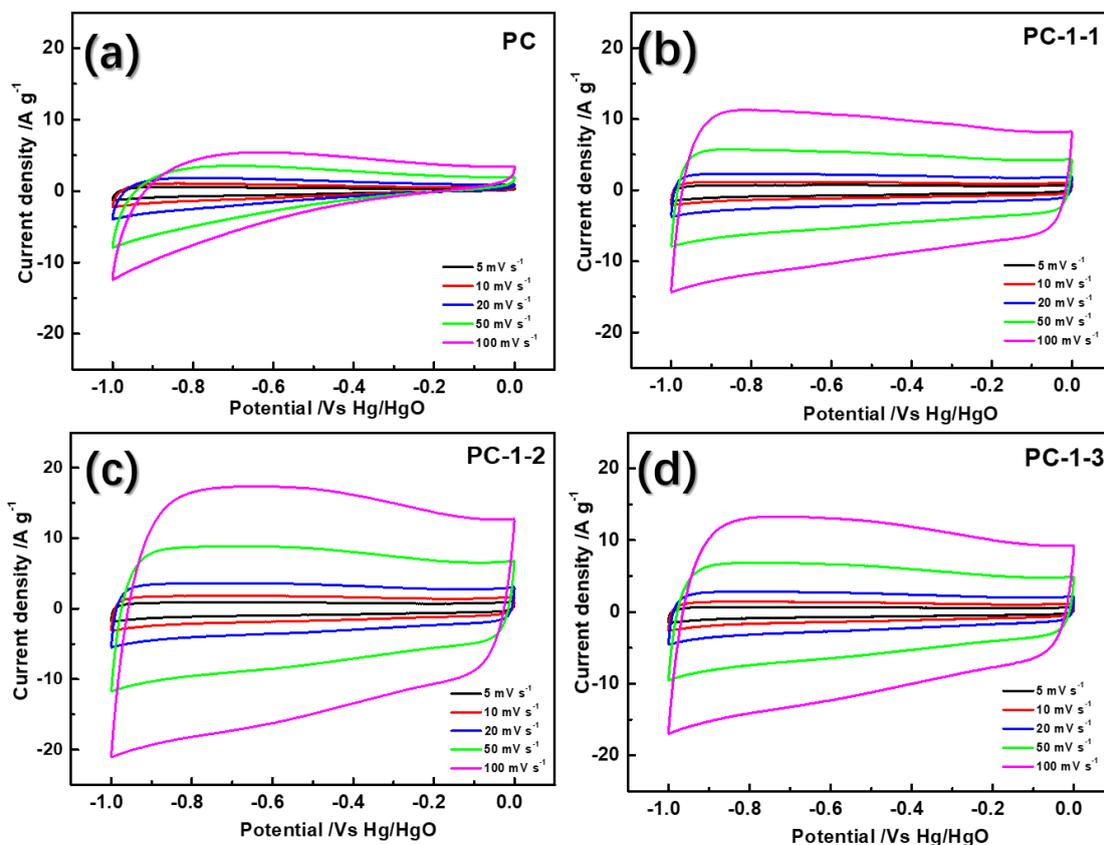
**Figure 6.** CV curves of (a) PC sample, (b) PC-1-1 sample, (c) PC-1-2 sample and (d) PC-1-3 sample at various scanning rates.
