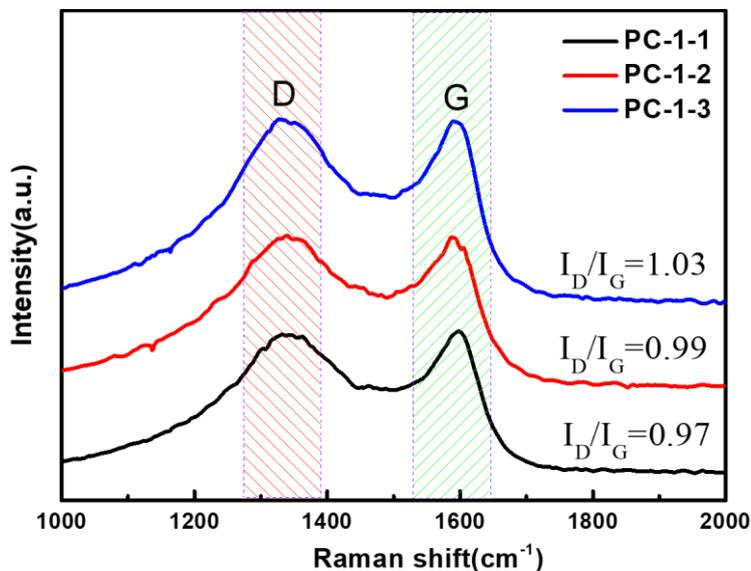
Figure 4. Raman spectra of PC-1-1, PC-1-2 and PC-1-3 samples.
